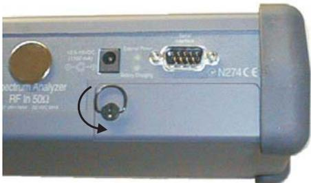
**Figure 6.** Rotate the Battery Access Door Handle
