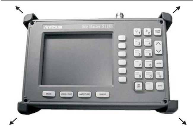
**Figure 11.** Removing the Corner Bumpers
