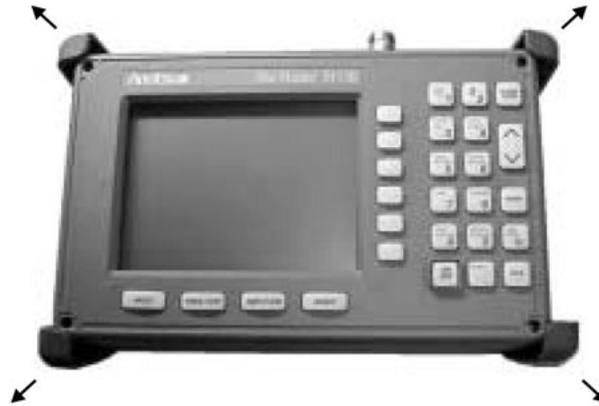
**Figure 3-8.** Removing the Corner bumpers
