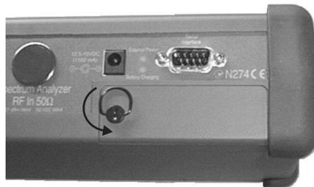
**Figure 5.** Rotate the Battery Access Door Handle
