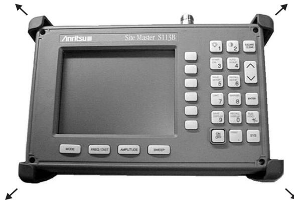
**Figure 9.** Removing the Corner Bumpers
