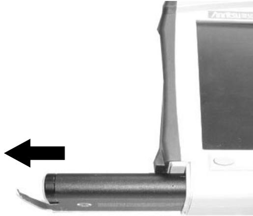
**Figure 7.** Removing the Battery
