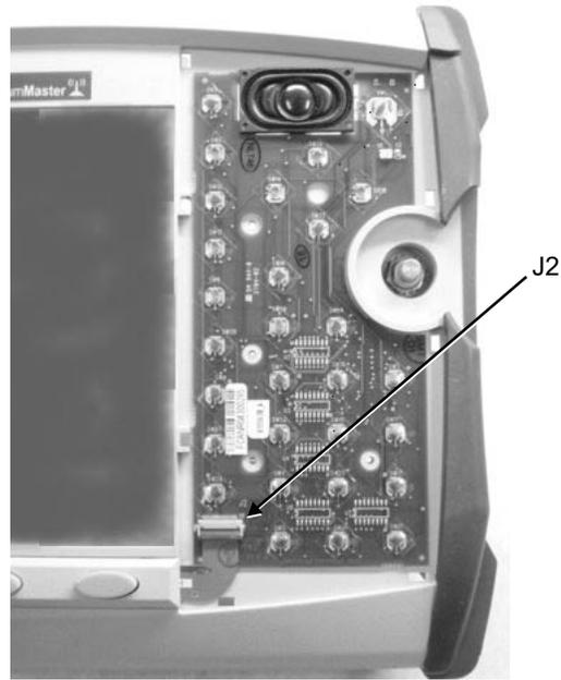
**Figure 19.** Keypad PCB
