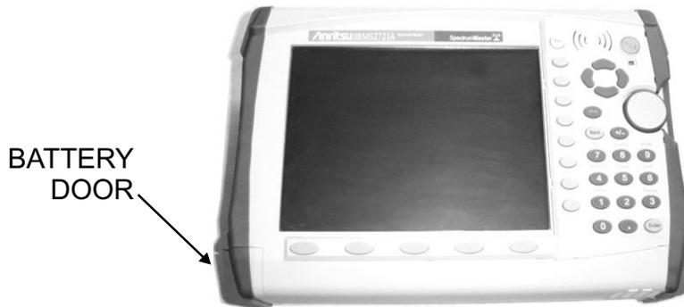
**Figure 4.** Battery Access Door Location
