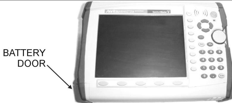
**Figure 7.** Battery Access Door Location
