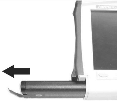
**Figure 10.** Removing the Battery
