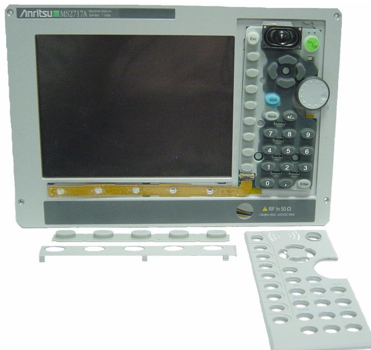
**Figure 4-32.** Keypads and Bezels, Front Panel
