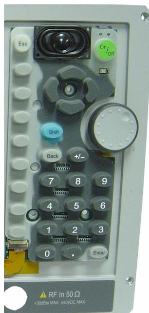
**Figure 4-30.** Numeric Keypad Rubber Membrane
