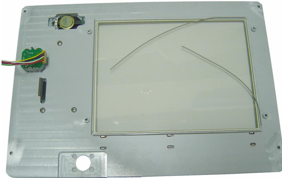
Figure 4-27. Front Panel Gaskets for LCD Display
