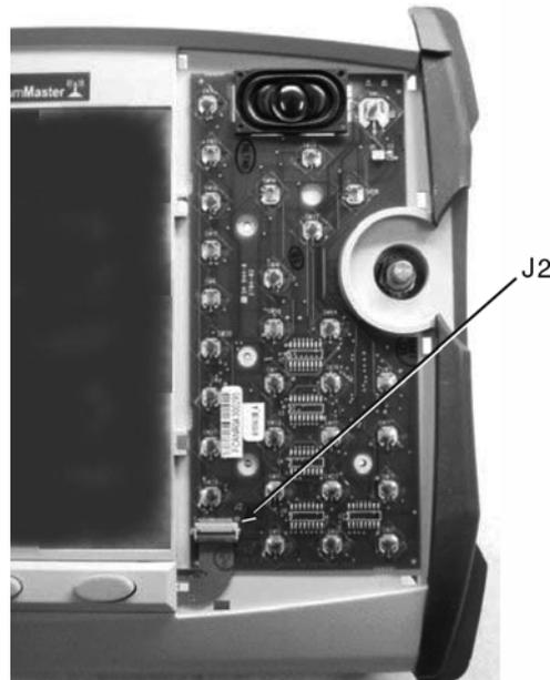
**Figure 5-6.** J2 Connector on Keypad PCB
