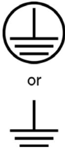
When supplying power to this equipment, connect the accessory 3-pin power cord to a 3-pin grounded power outlet. If a grounded 3-pin outlet is not available, use a conversion adapter and ground the green wire, or connect the frame ground on the rear panel of the equipment to ground. If power is supplied without grounding the equipment, there is a risk of receiving a severe or fatal electric shock.
