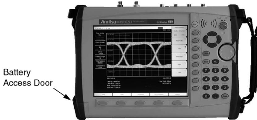
**Figure 4-1.** MP1026 Battery Access Door Location
