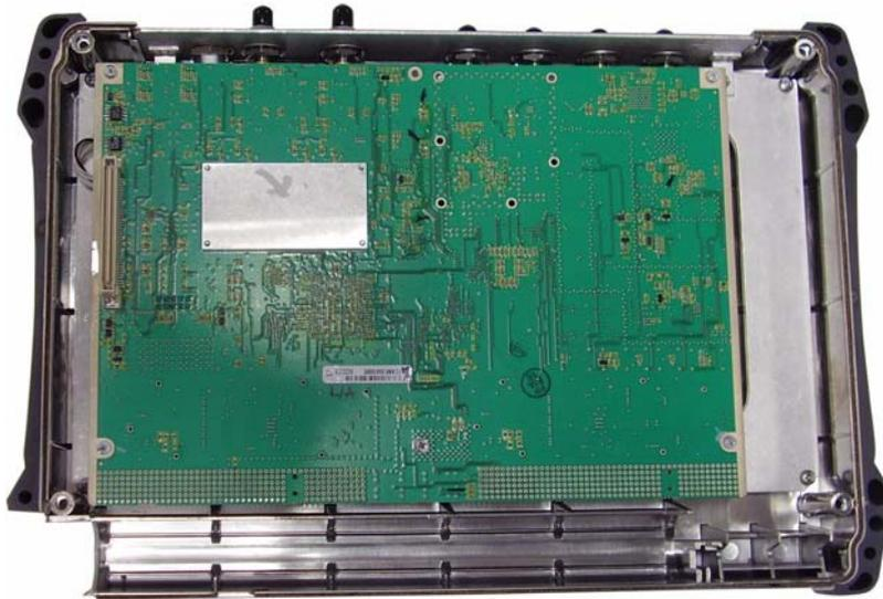
**Figure 5-4.** Oscilloscope PCB
