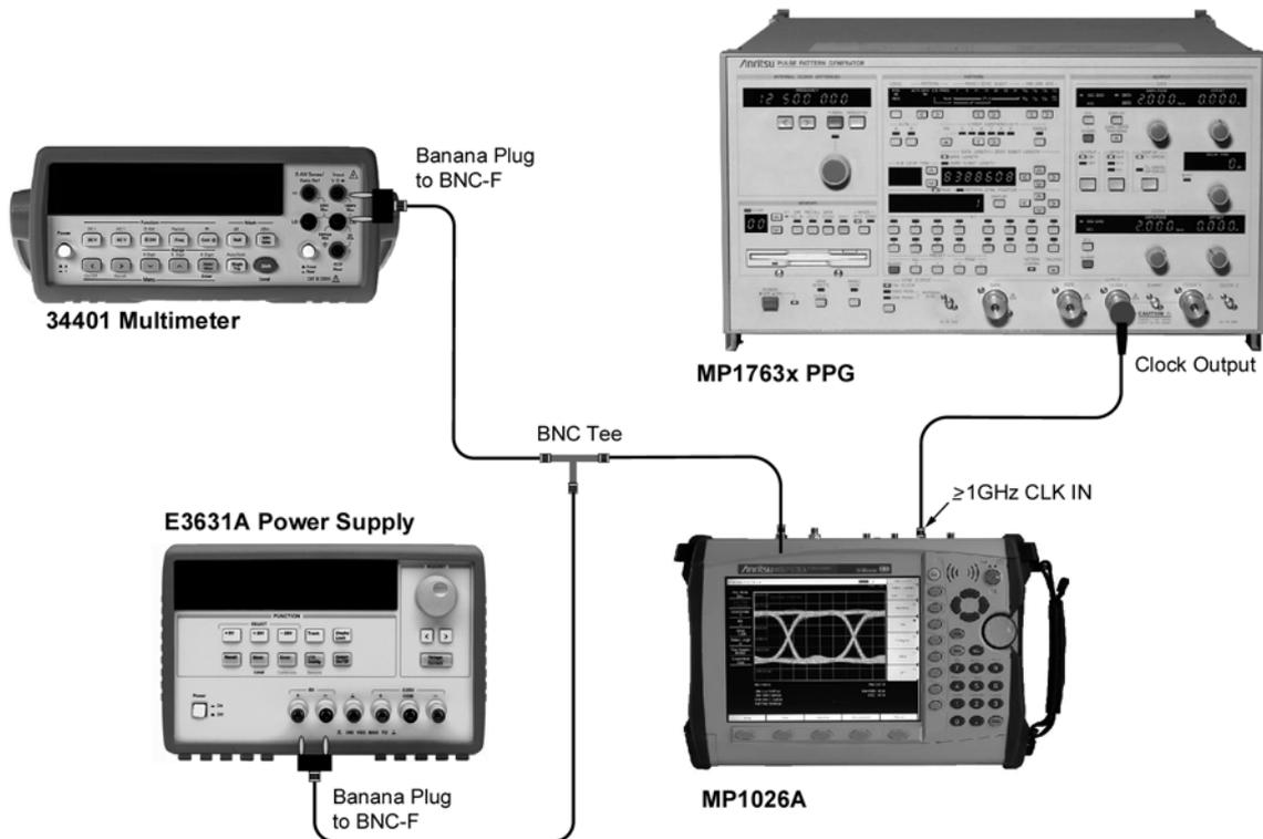
**Figure 3-2.** Amplitude Accuracy Test Setup
