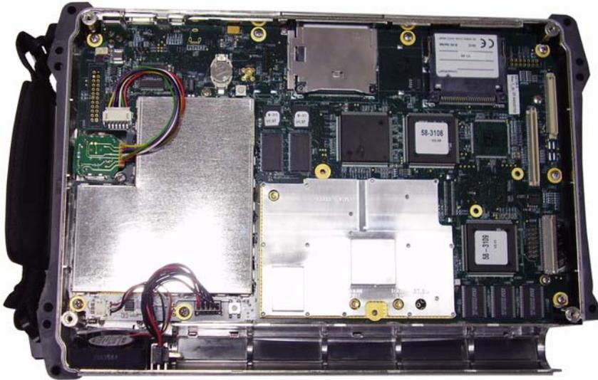
Figure 5-3. Removing the Main PCB
