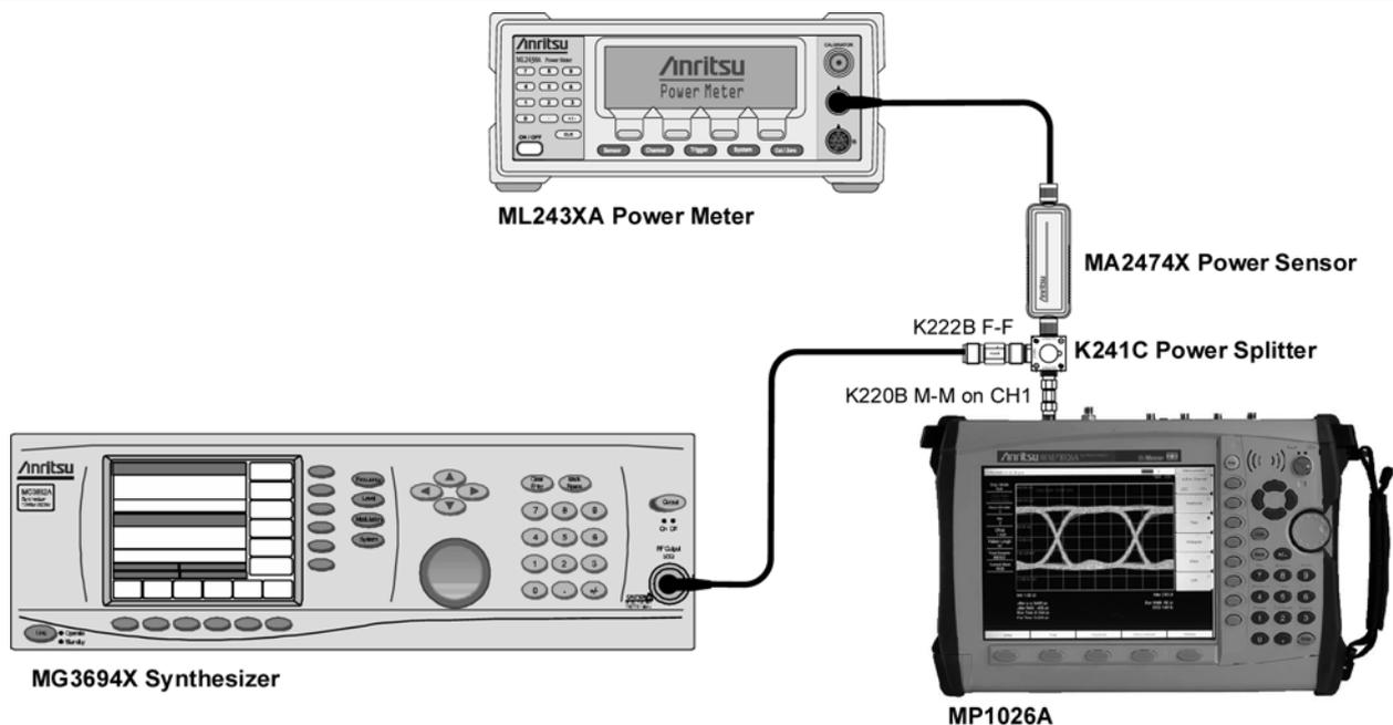
**Figure 3-1.** Bandwidth Verification Setup
