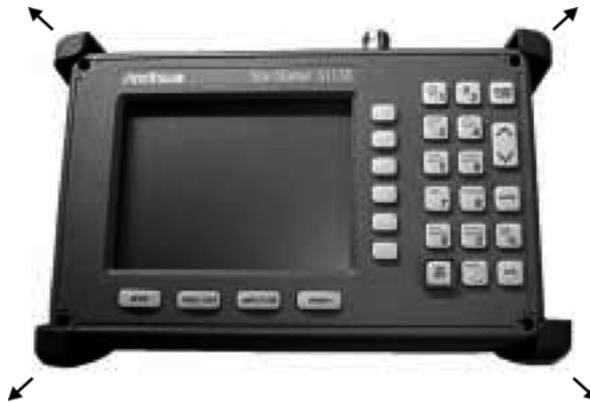
**Figure 3-3.** Removing the Corner Bumpers
