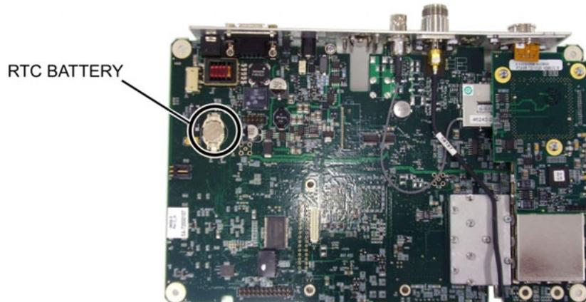
Figure 3-6. RTC Battery Location
