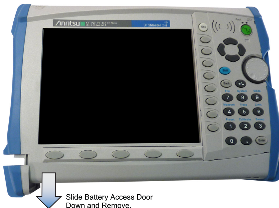
Figure 6-3. Removing the Battery Access Door
