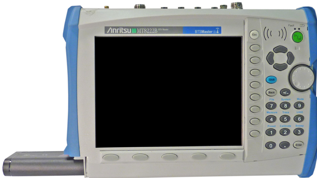
Figure 6-4. Removing the Battery
