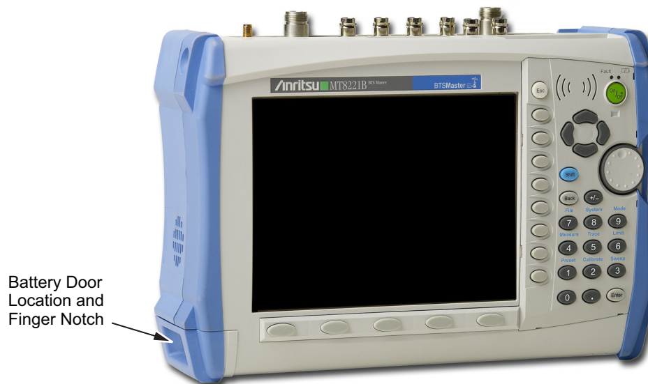
Figure 6-1. Battery Access Door Location and Finger Notch
