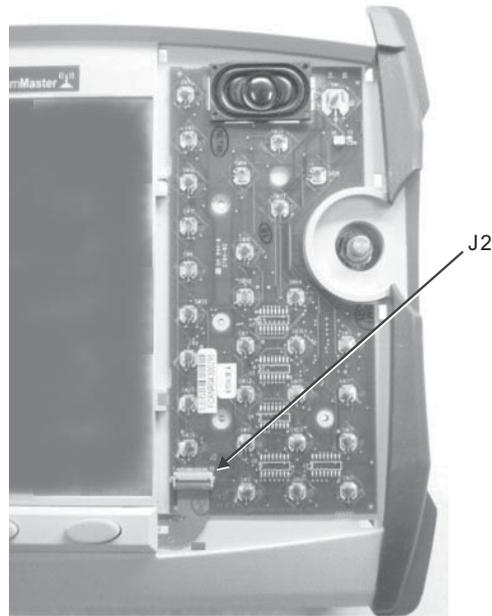
**Figure 5-15.** Connector J2 on Keypad PCB
