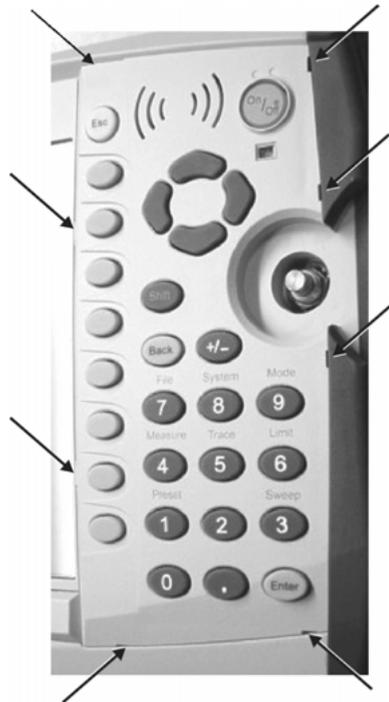
**Figure 5-14.** Locking Tabs on Front Bezel
