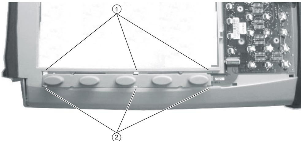
1. Location of three (3) upper locking tabs on the Soft Key Switch Bezel and underlying Soft Key Membrane.
