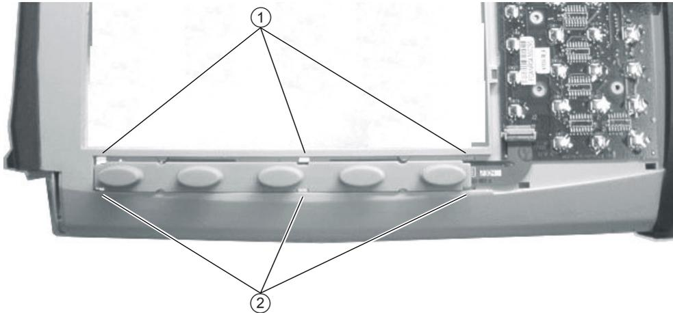
1. Location of three (3) upper locking tabs on the Soft Key Keypad Bezel (not shown) and the Keypad Membrane.
