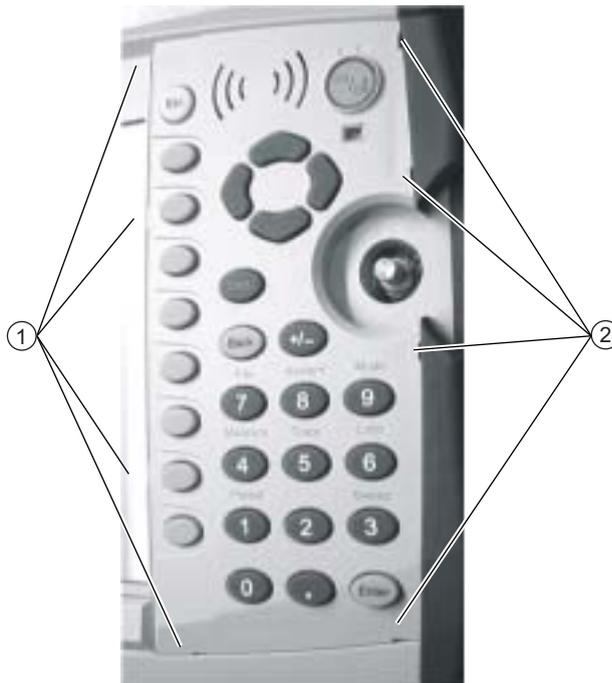
1. Location of Main Keypad Switch Bezel four (4) left side locking tabs
