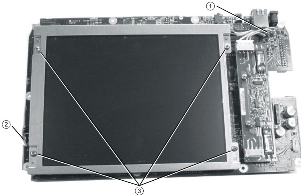
1. LCD Backlight Cable, permanently attached to LCD. Connects to Backlight Power Inverter Assembly.
