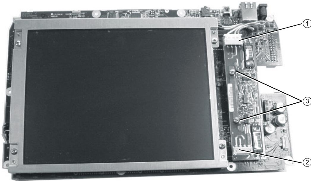
1. LCD Backlight Cable, permanently attached to LCD. Connects to LCD Backlight Power Inverter Assembly.
