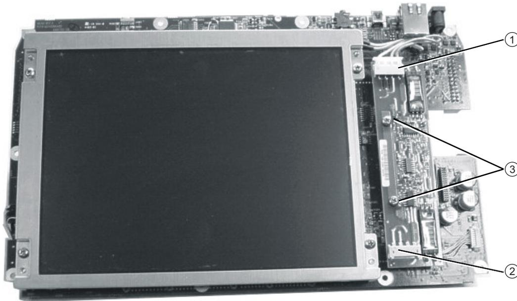
1. LCD Backlight Cable, permanently attached to LCD Assembly.
