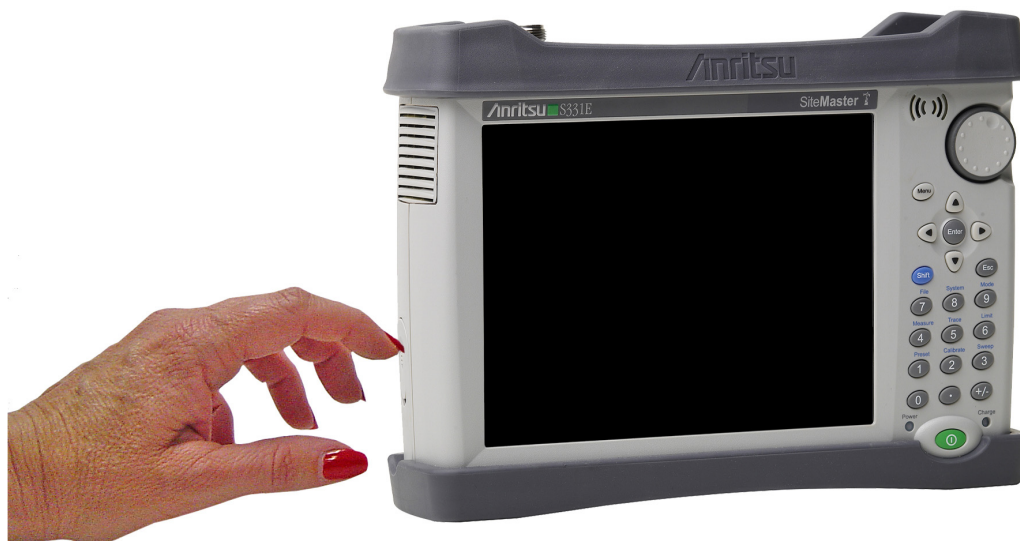
Figure 5-2. Opening the Battery Access Door
