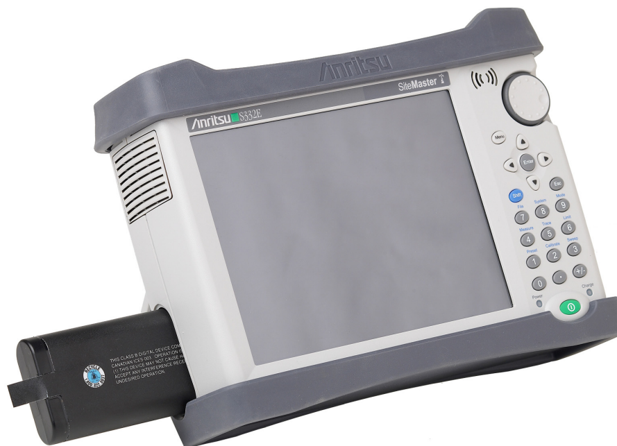
Figure 5-3. Removing the Battery
