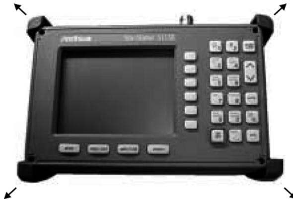
**Figure 3-3.** Removing the Corner Bumpers
