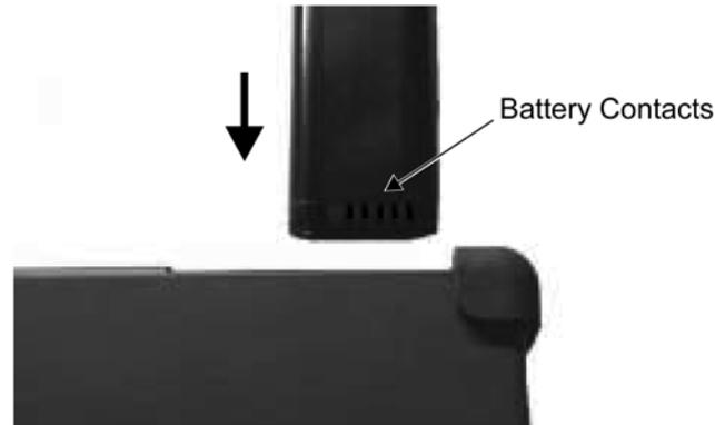
**Figure 3-2.** Battery Pack Replacement
