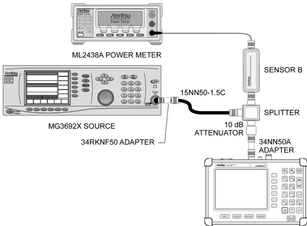
**Figure 2-2.** Level Accuracy with Frequency Test Setup
