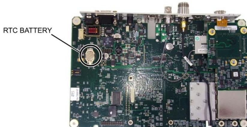
**Figure 3-6.** RTC Battery Location
