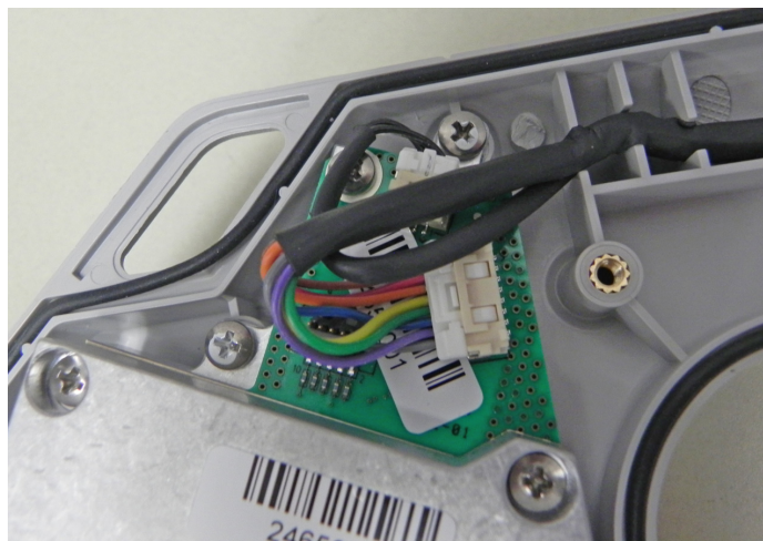
Figure 3-6. Remove the Cables from the Motherboard
