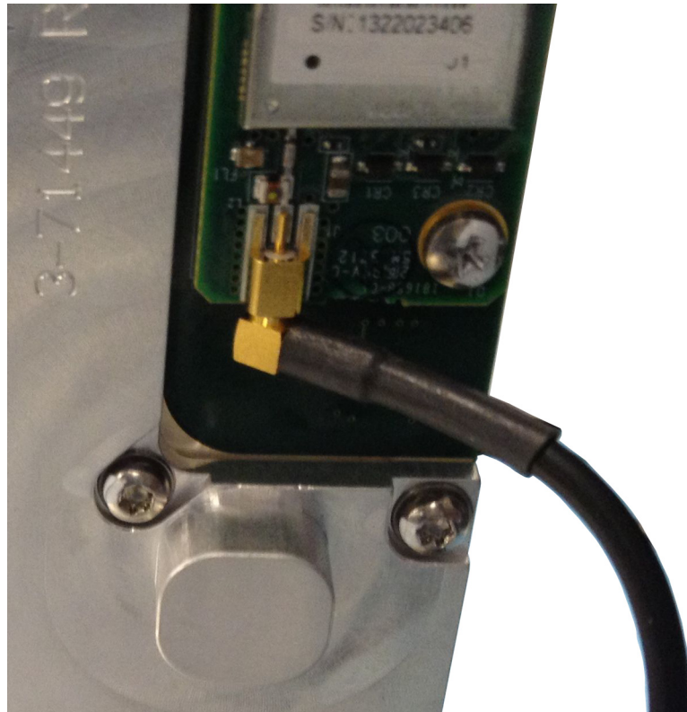
Figure 5-43. GPS Module with MMCX Cable Attached
