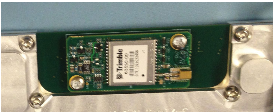
Figure 5-42. GPS Module (Option 31) on Motherboard
