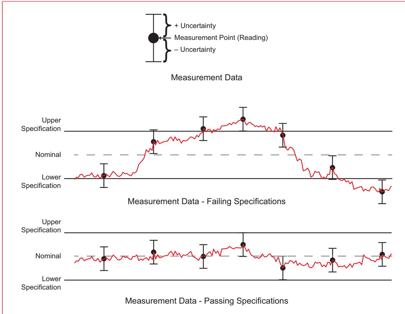
**Figure 2-1.** Pass/Fail Determination
