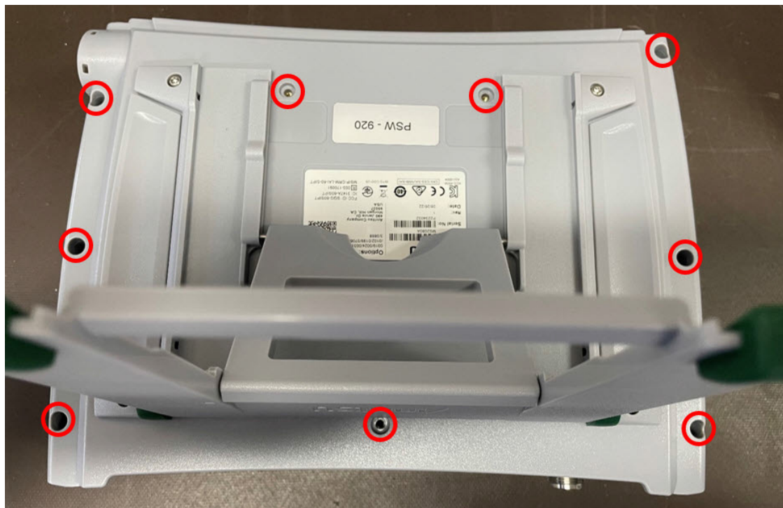
Figure 5-5. Rear Case Removal
