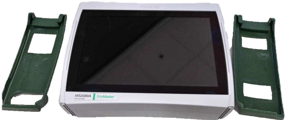
Figure 5-4. Side Bumpers Removal
