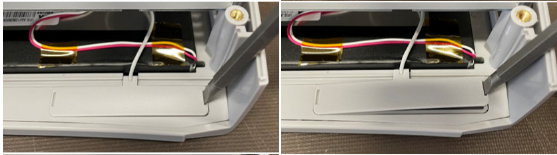
Figure 5-12. Releasing the Wi-Fi antennas
