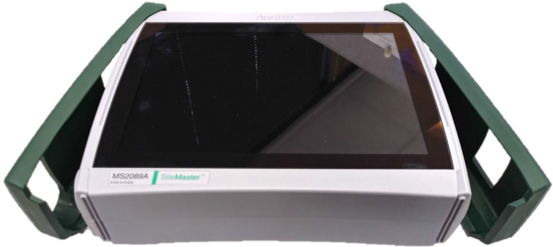
Figure 5-3. Pulling of Side Bumpers
