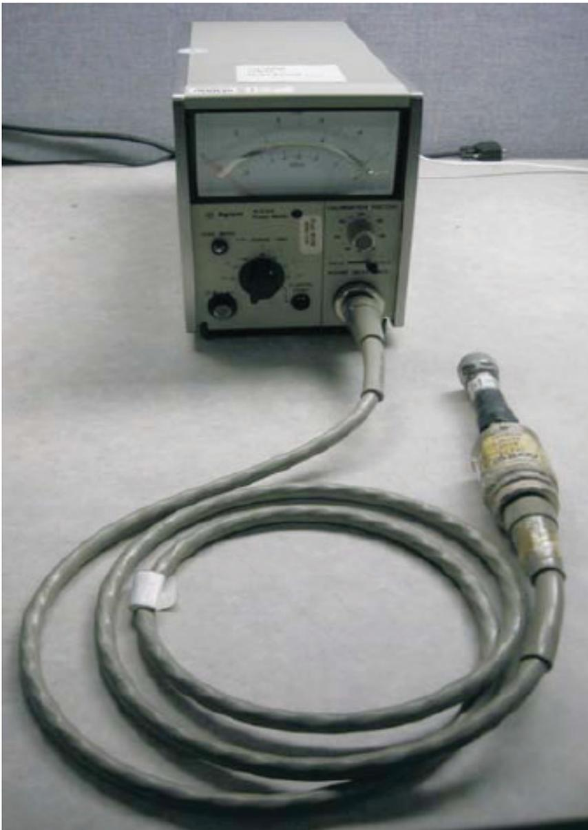
432A Power Meter shown connected to the 8478B Power Sensor.
