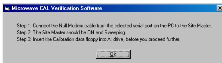
**Figure 2-1.** CAL Verification Software Opening Dialog Box
