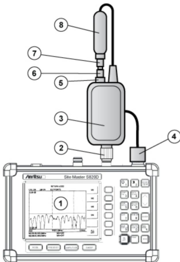
Figure 2-10. Two-Port Cable Loss Measurement Accuracy Connections
