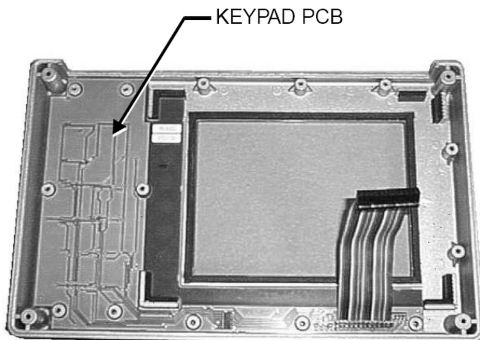
**Figure 3-6.** Front Panel Keypad PCB Location
