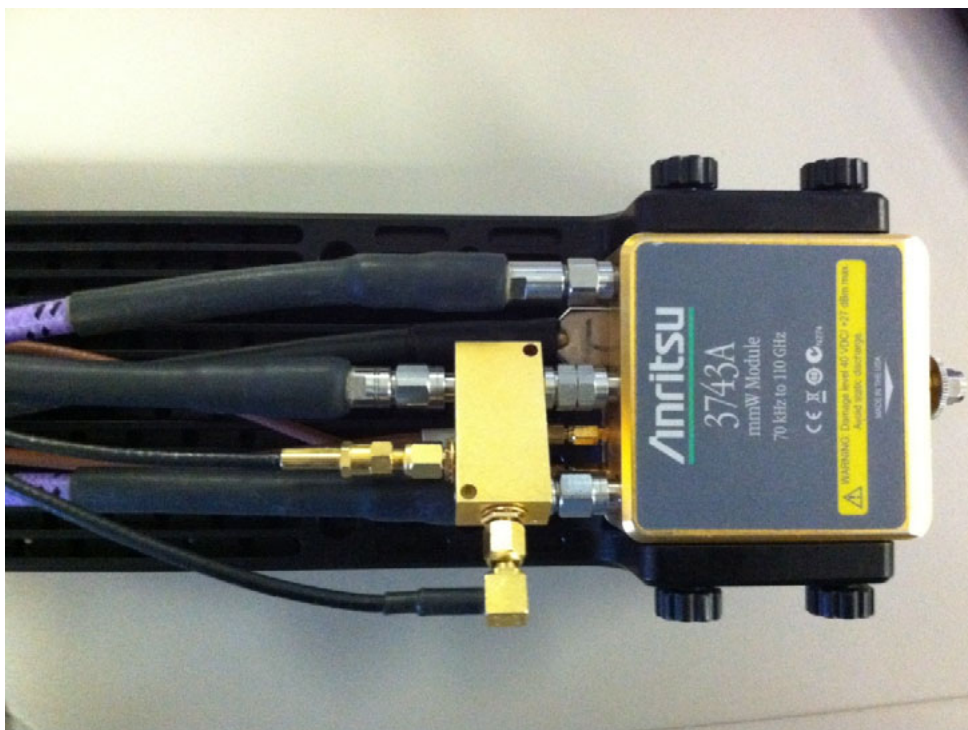
Figure 16-21. The connection of a Kelvin bias tee to a mm-wave module is shown here.
