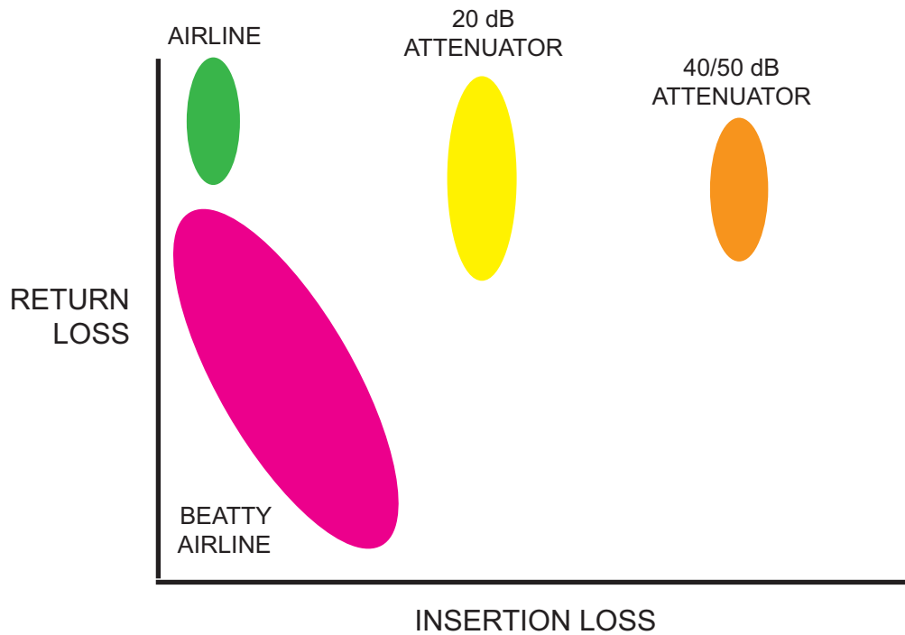
Figure 10-2. Regions of Parameter Coverage of Verification Kit Component
