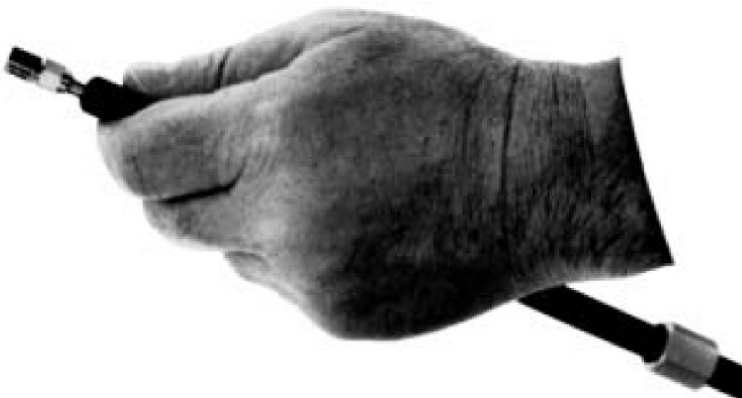
Figure 1-9. Holding F-F Sliding Terminator
