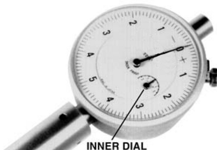
Figure 1-16. Fine Lock Adjustment with Gauge Inner Dial Reading “0”
