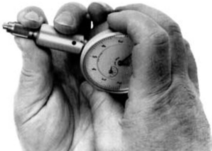
Figure 1-18. Preparing the Gauge for the Female Adapter
