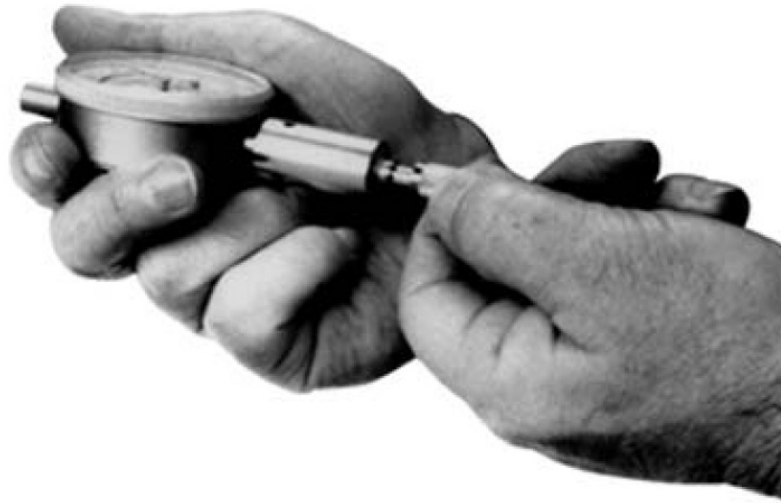
Figure 1-12. F-F Sliding Terminator, Installing Gauge
