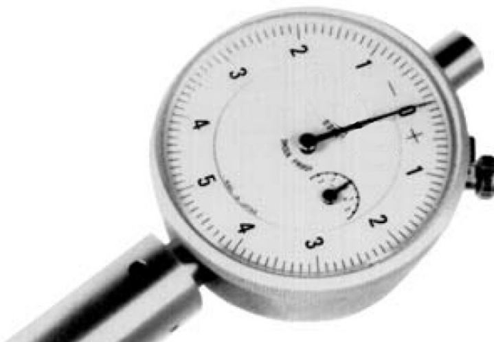
Figure 1-7. Dial Bezel and Pointer at “0”
