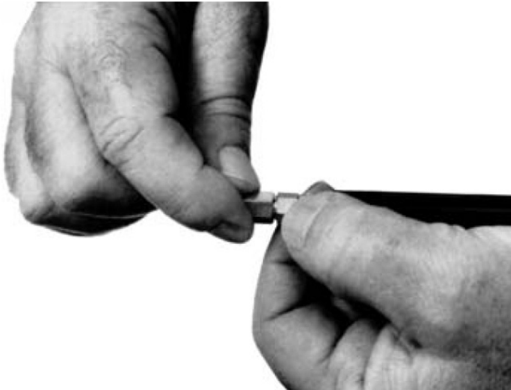
Figure 1-11. F-F Sliding Terminator, Removing Flush Short
