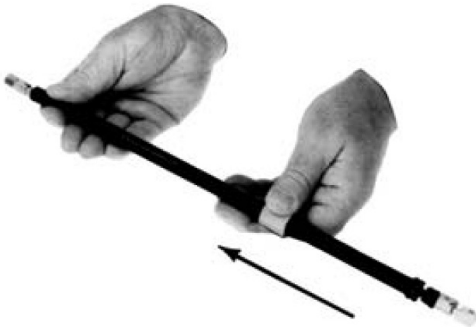
Figure 1-8. F-F Sliding Terminator, Towards End Closest to Connector
