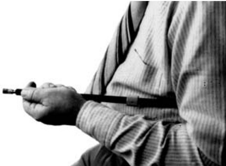
Figure 1-10. Holding F-F Sliding Terminator, Ready to Measure
