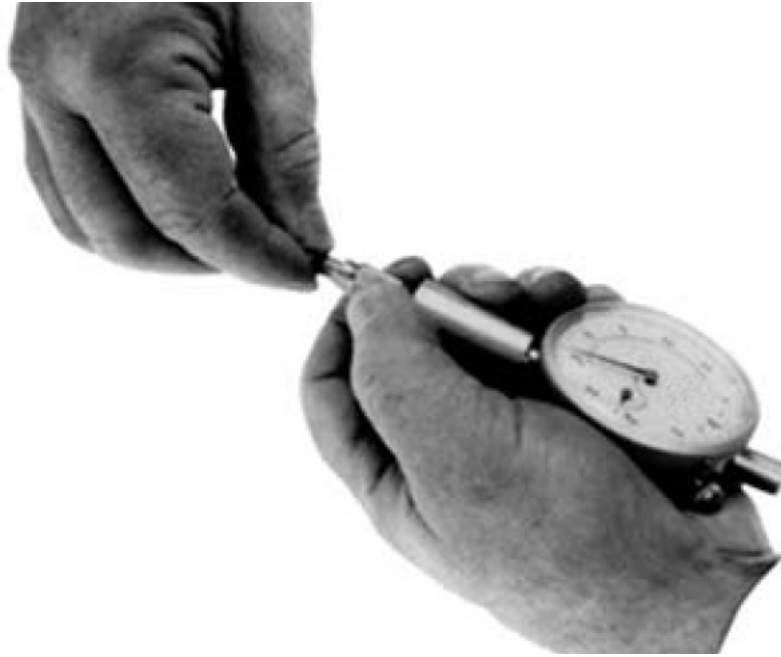
Figure 1-20. Installing the Female Adapter on the Gauge
