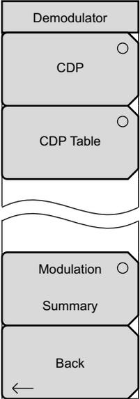
**CDP:** The first press of this submenu key displays the Code Domain Power and also displays an arrow on the submenu key symbol (to indicate that a sub menu is available).
