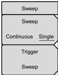
**Sweep Single/Continuous:** This submenu key toggles between continuous sweep and single sweep. In single sweep mode, the results of a sweep are displayed on the screen while the instrument awaits a trigger event to start a new sweep.
