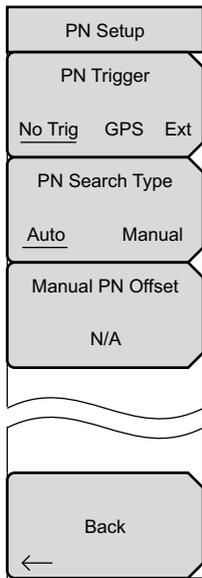
**PN Trigger:** This submenu key toggles through “No Trig” (no trigger), “GPS”, and “Ext” (external trigger).
