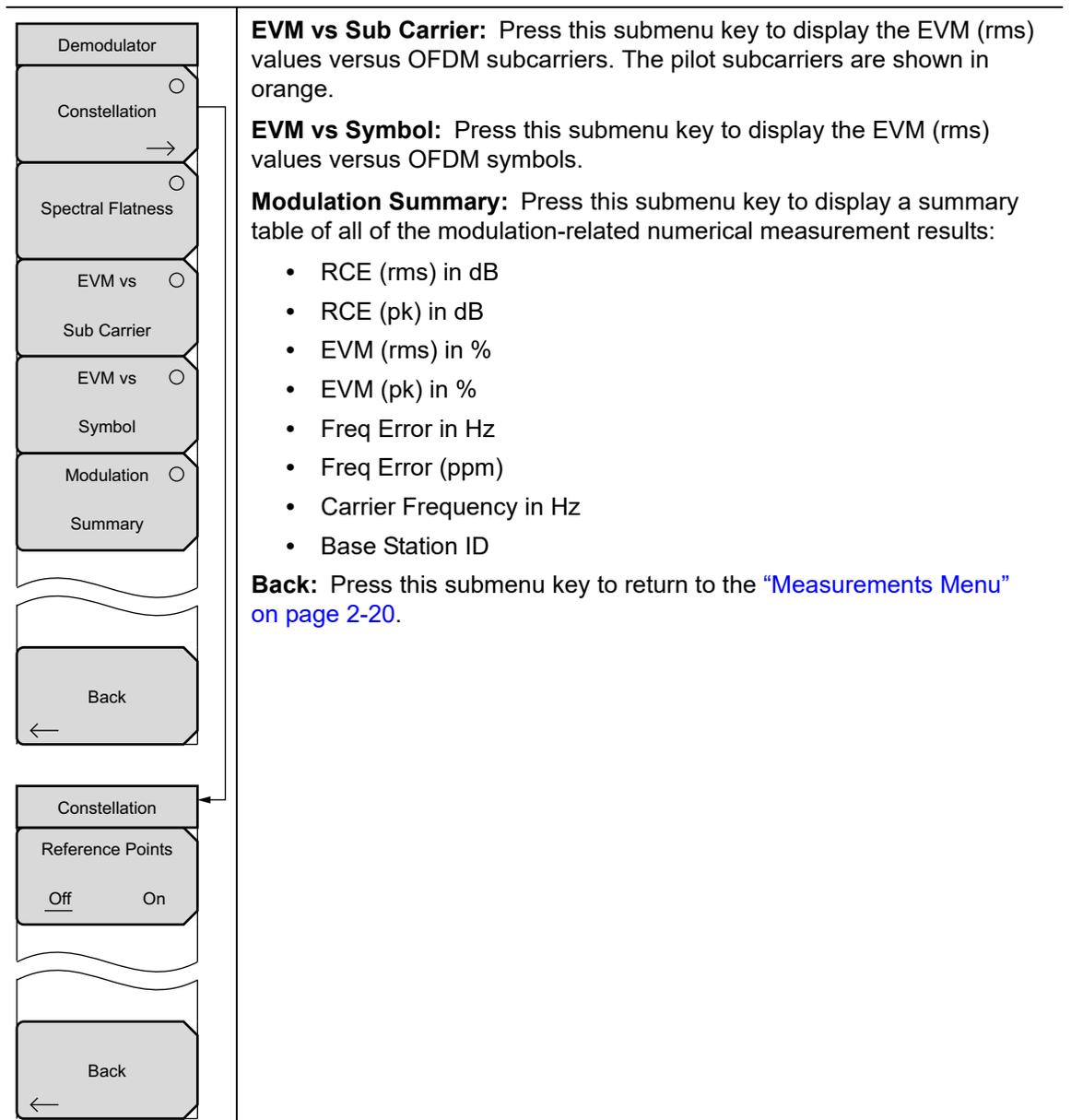
Figure 2-19. Fixed WiMAX Demodulator Menu (2 of 2)
