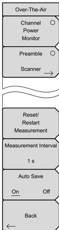
**Channel Power Monitor:** Displays the Channel Power (RSSI) value over a variable time period that is specified with the Measurement Interval submenu keys.
