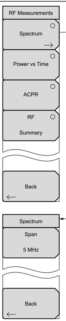
The diagram illustrates the RF Measurements Menu structure. The main menu includes options for Spectrum, Power vs Time, ACPR, RF, and Summary. A 'Back' button is located below the main menu. The Spectrum submenu is shown below, containing options for Span (currently set to 5 MHz) and another 'Back' button. Arrows indicate the flow from the main menu to the Spectrum submenu and from the Spectrum submenu back to the main menu.
