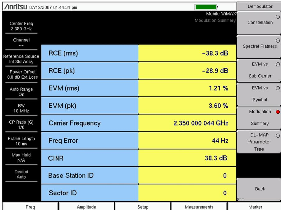
**Figure 3-10.** Mobile WiMAX Demodulator Modulation Summary Measurement
