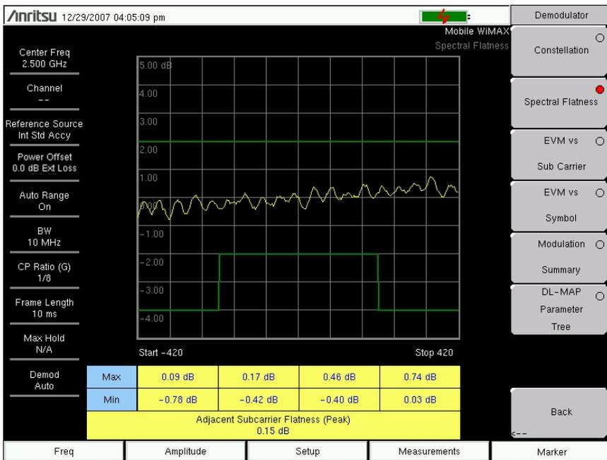
Figure 3-7. Mobile WiMAX Demodulator Spectral Flatness Measurement
