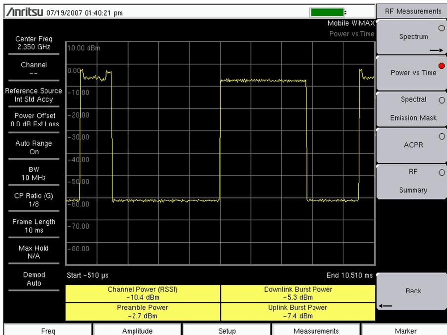
**Figure 3-2.** Mobile WiMAX Power versus Time Measurement
