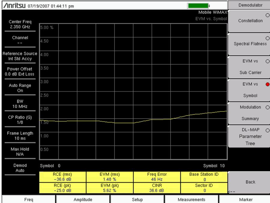
Figure 3-9. Mobile WiMAX Demodulator EVM versus Symbol Measurement
