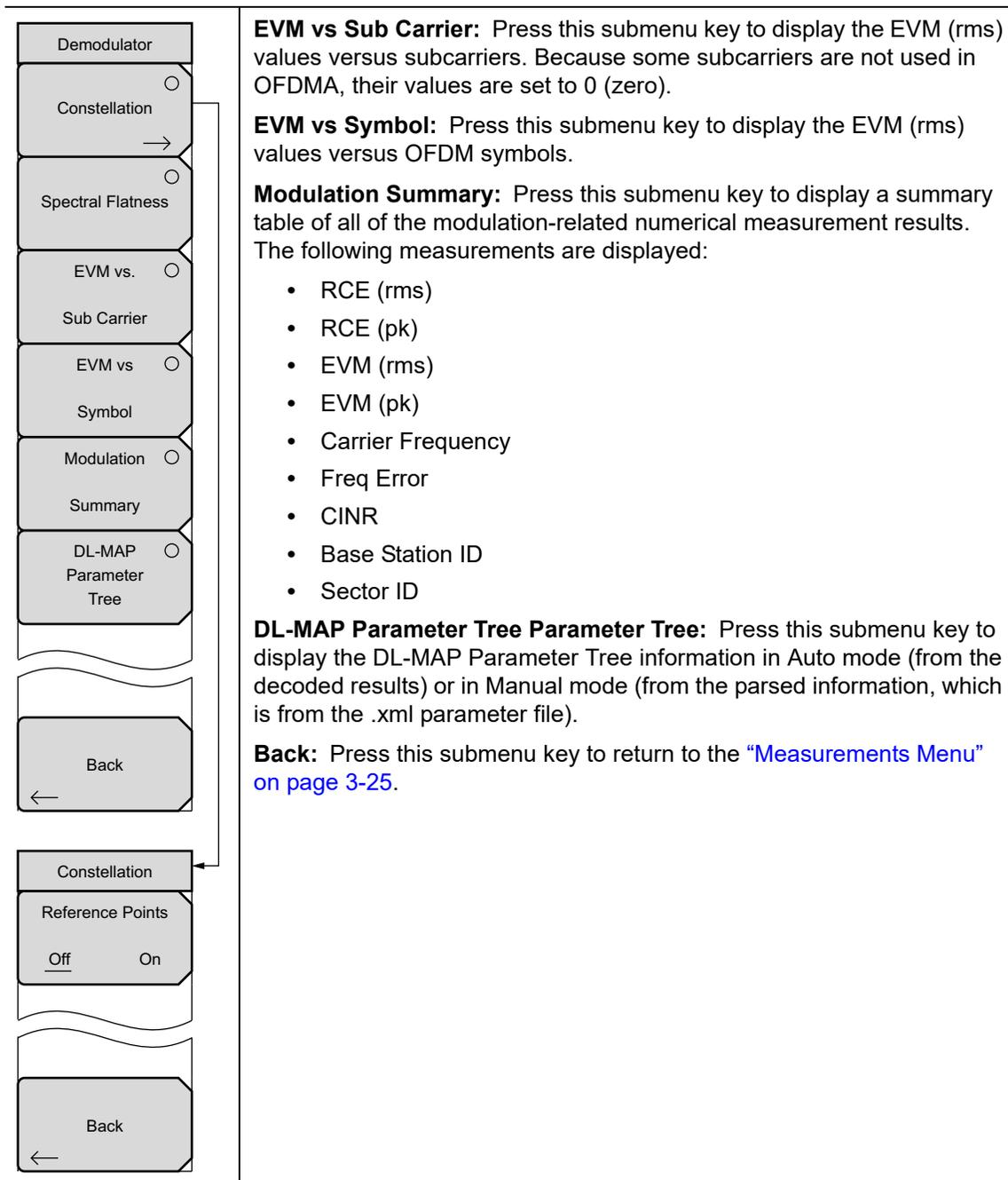
Figure 3-26. Mobile WiMAX Demodulator Menu (2 of 2)
