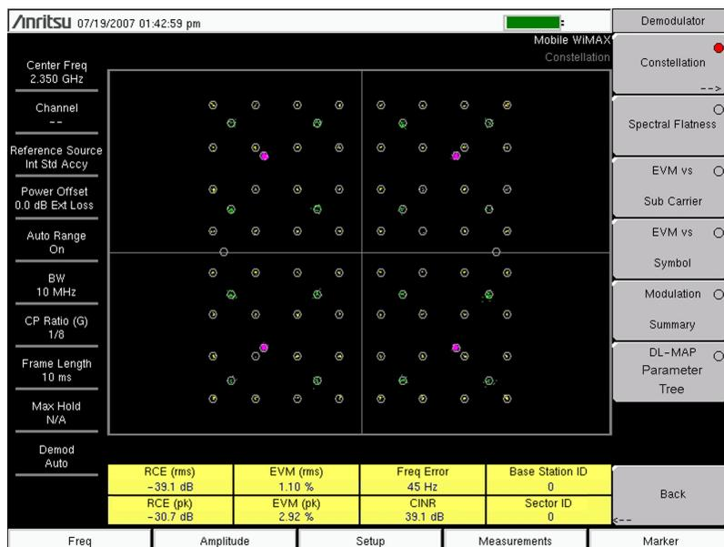
**Figure 3-6.** Mobile WiMAX Demodulator Constellation Measurement
