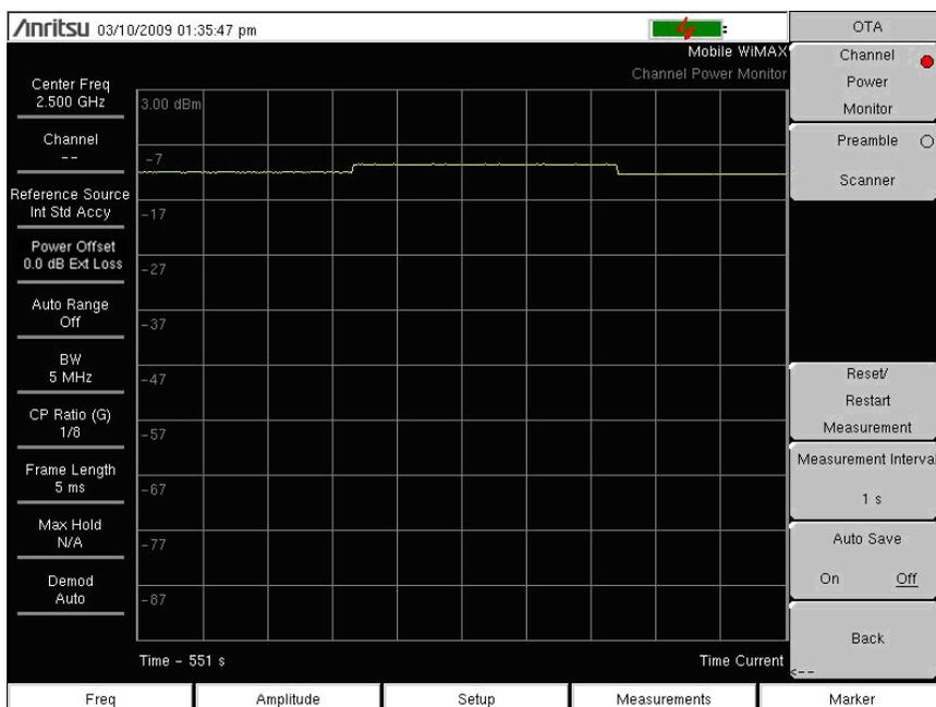
**Figure 3-12.** Mobile WiMAX OTA Channel Power Monitor Measurement
