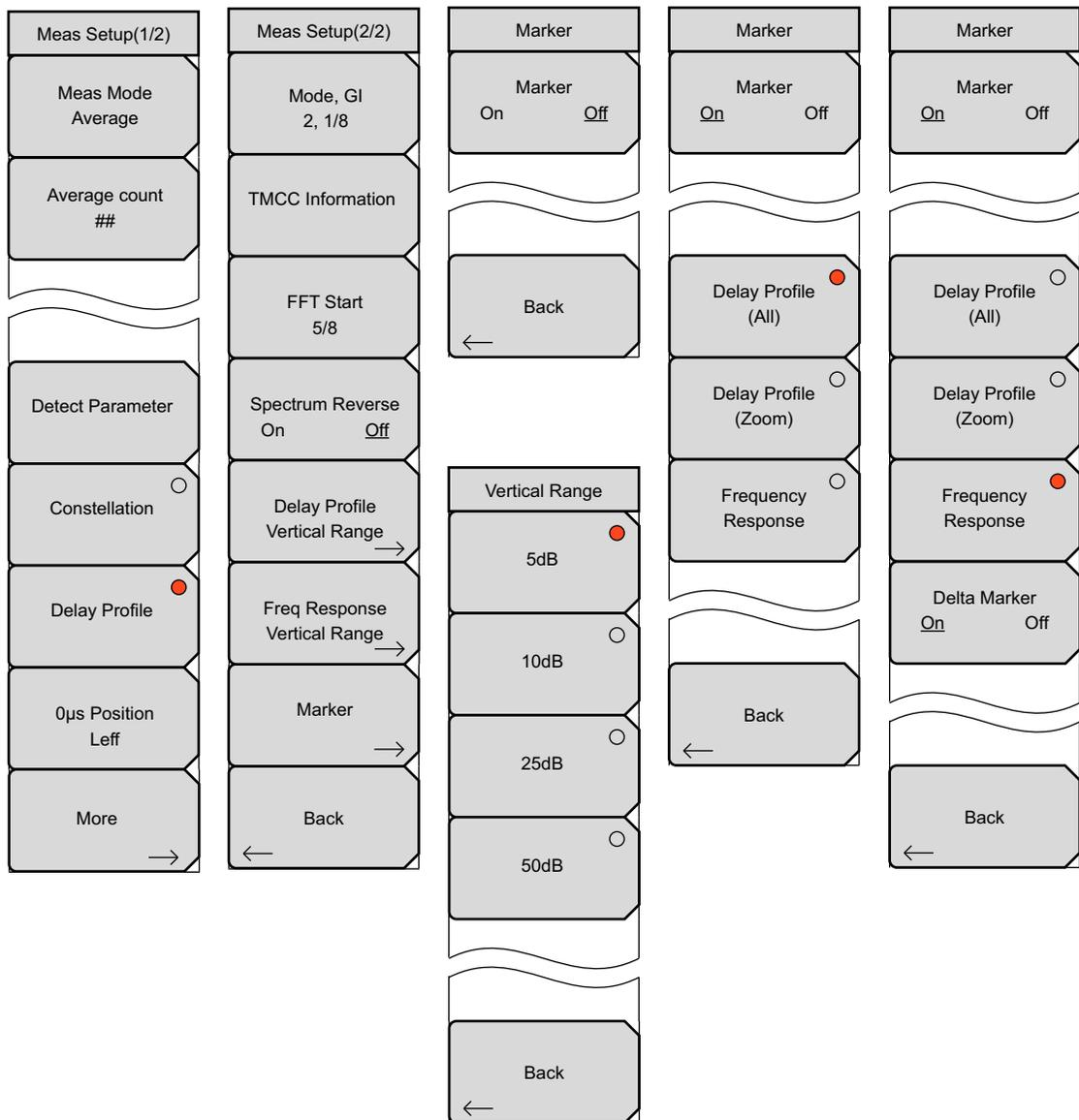
**Figure 4-12.** Delay Profile Setup and Marker Menus
