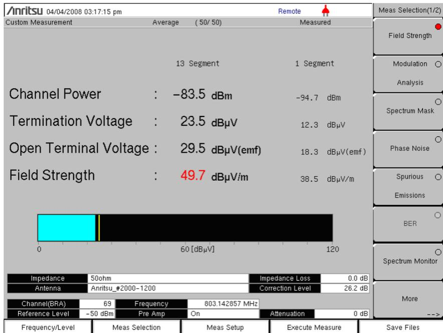
**Figure 4-3.** Measurement Screen and Meas Selection (1/2) Menu
