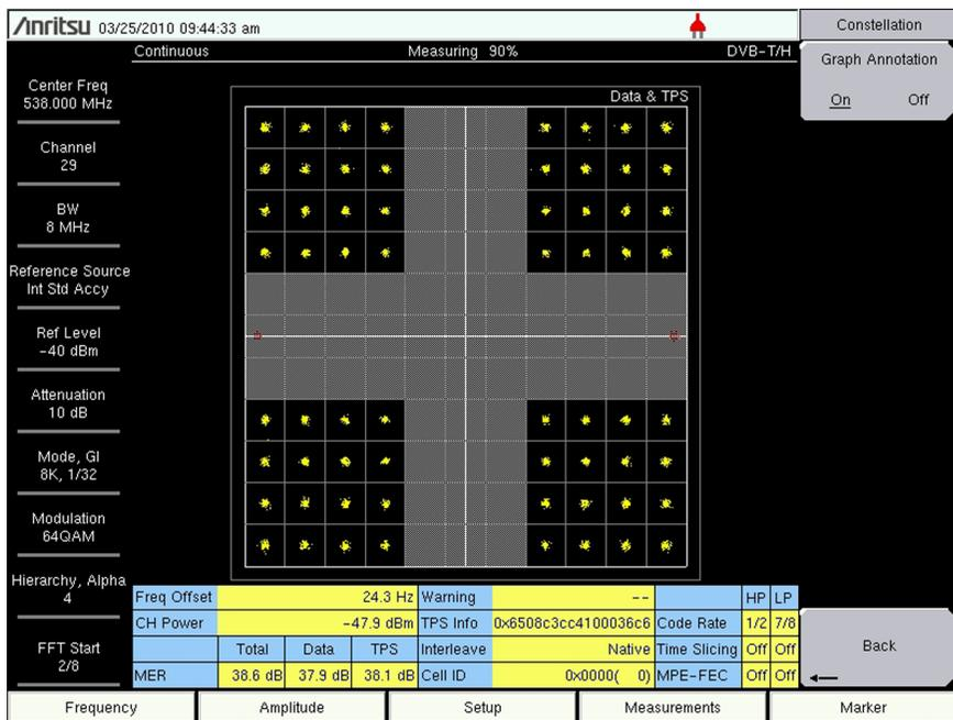
Figure 2-8. 64QAM with Hierarchy set to 4
