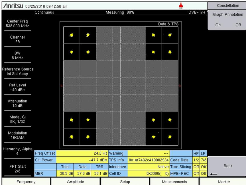
Figure 2-6. 16QAM with Hierarchy set to 4
