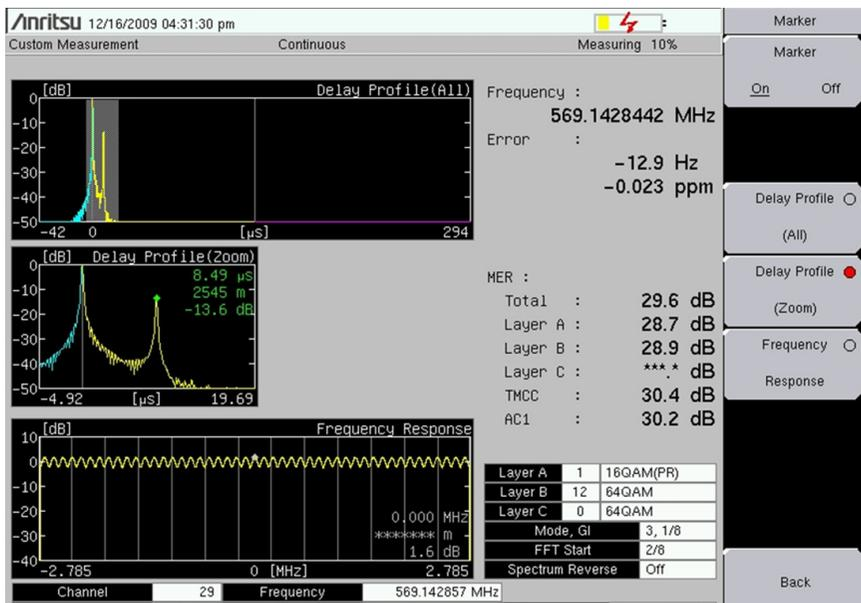
Figure 4-61. Marker Enabled in Delay Profile (Zoom) Graph
