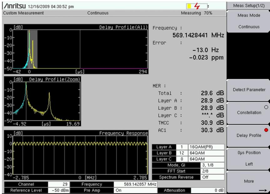
Figure 4-60. Modulation Analysis – Delay Profile Measurement Display
