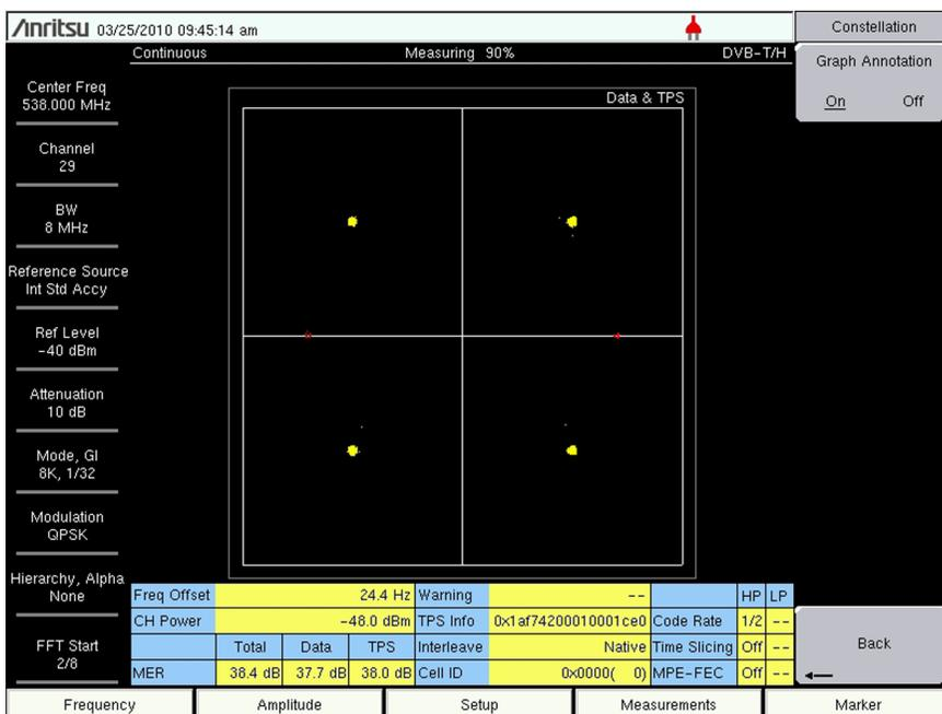
Figure 2-2. QPSK with Hierarchy set to None
