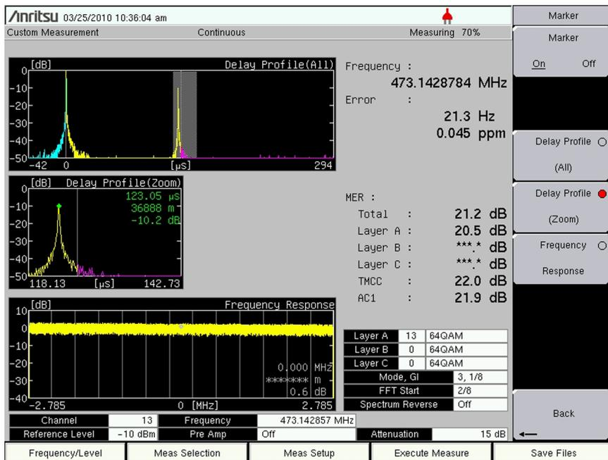
**Figure 4-62.** Marker Enabled in Delay Profile (Zoom) Graph
