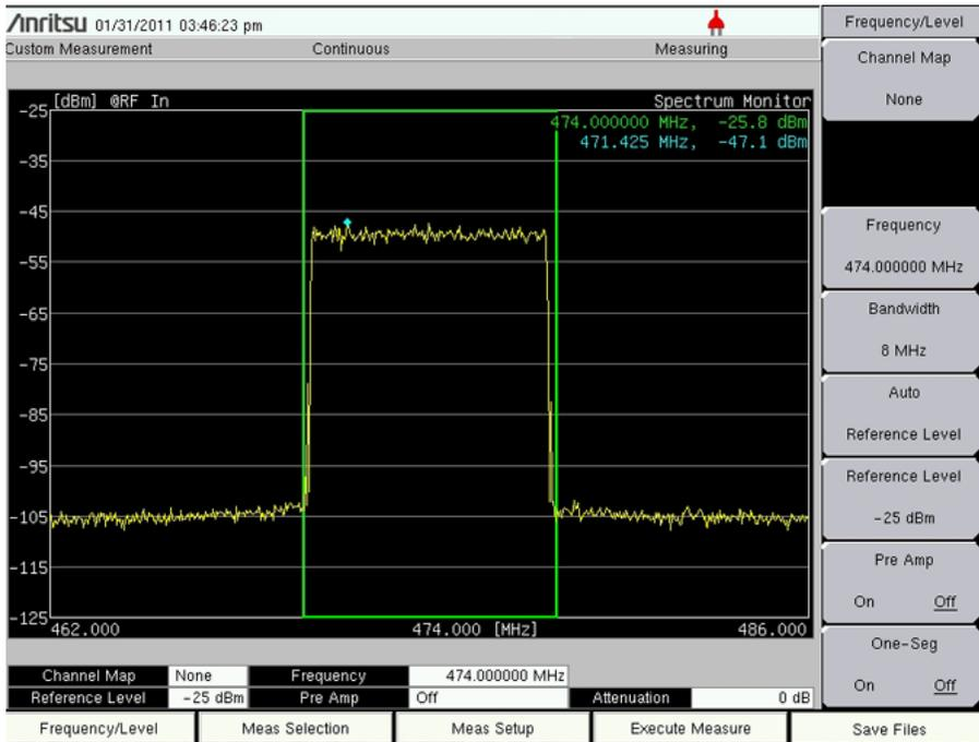
**Figure 4-27.** Spectrum Monitor with 8 MHz Bandwidth Selected
