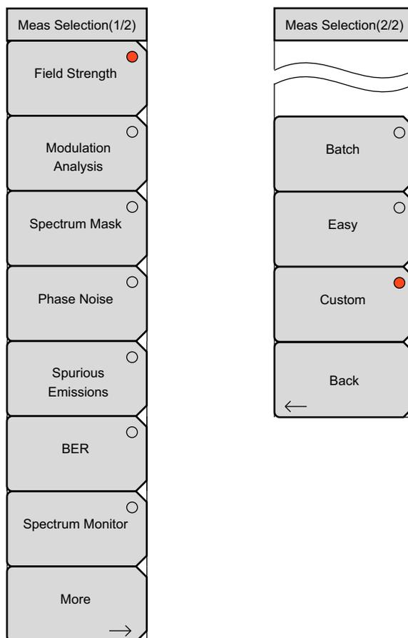
**Figure 4-32.** Measurement Selection Menus for Custom and Easy
