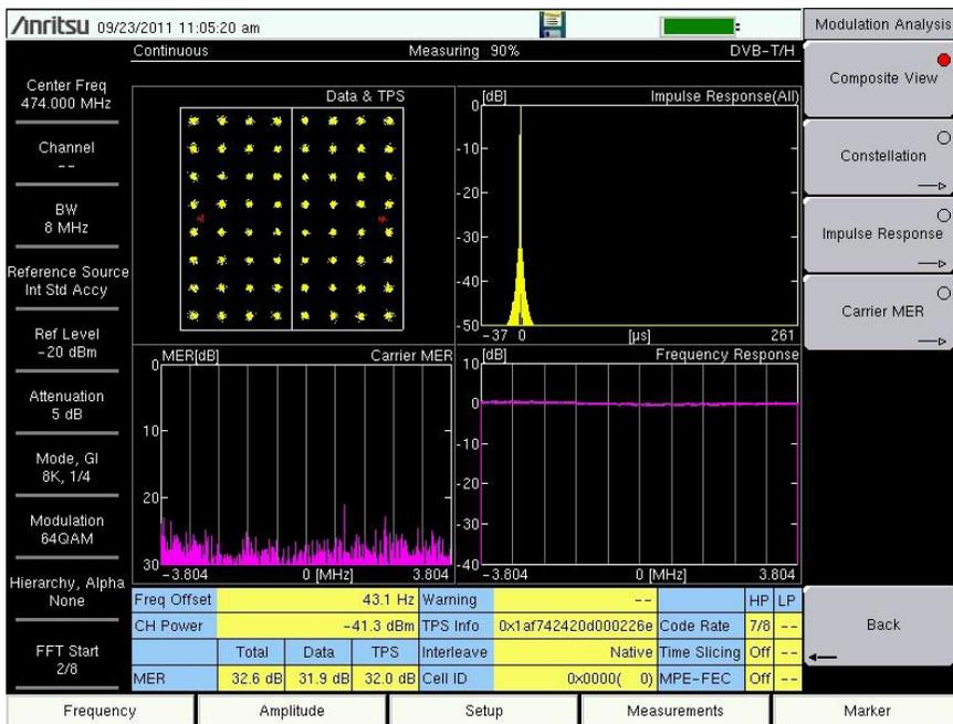
Figure 2-1. A 64QAM Constellation Graph in Composite View
