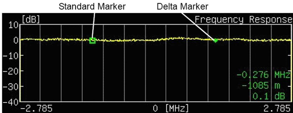
Figure 4-66. Frequency Response Graph with Delta Marker
