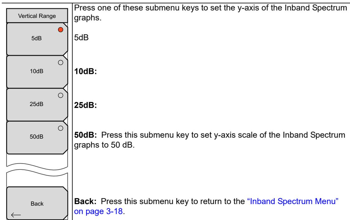
**Figure 3-15.** Vertical Range Menu (Inband Spectrum)
