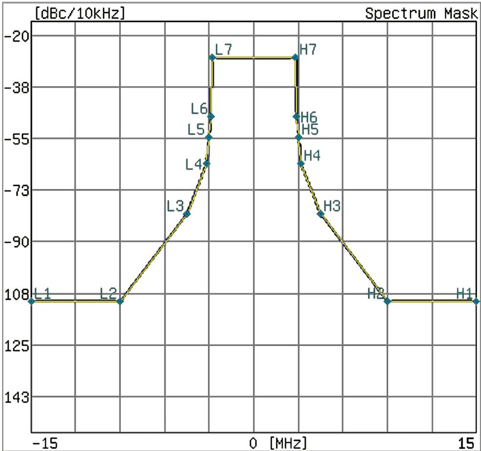
Figure 4-18. Noncritical Mask for UHF (Brazil) Channel Map
