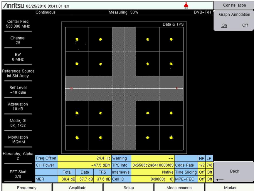
Figure 2-5. 16QAM with Hierarchy set to 2
