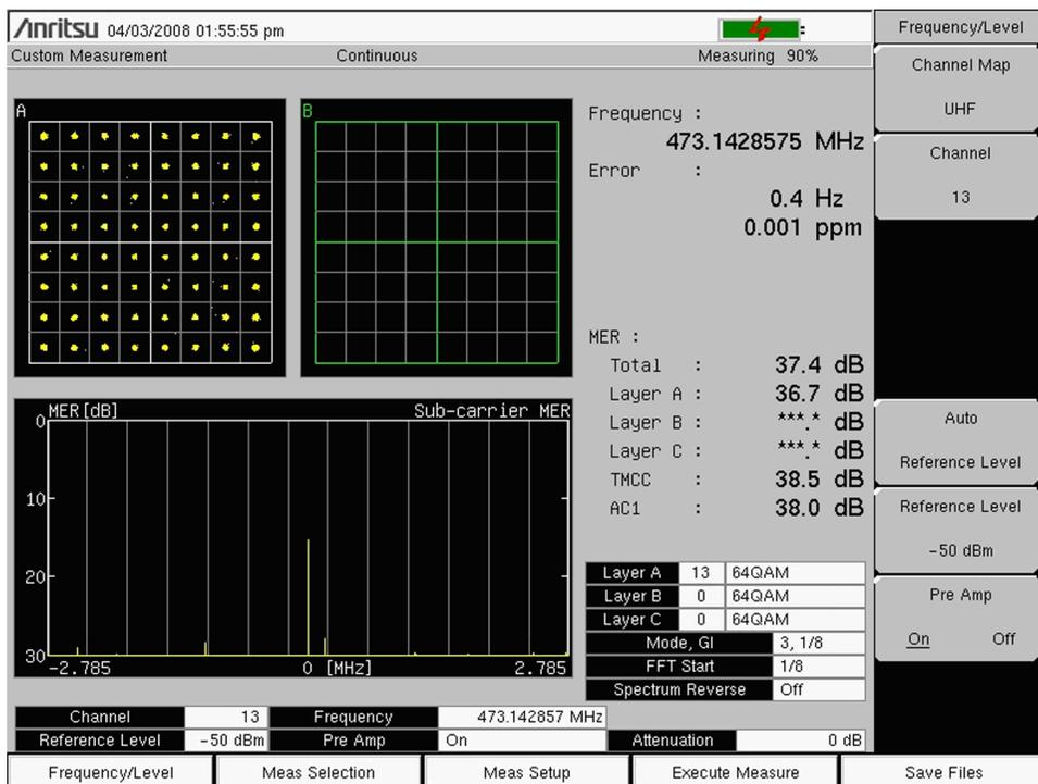
**Figure 4-11.** Modulation Measurement Screen – Constellation Display
