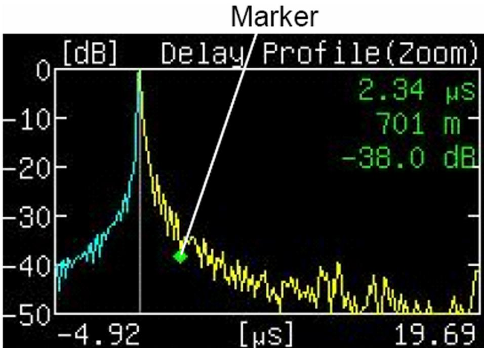
Figure 4-64. Enlarged (Zoom) Graph of Delay Profile
