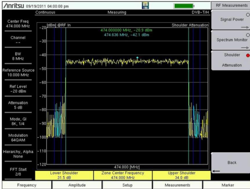
Figure 2-11. Shoulder Attenuation Measurement Screen
