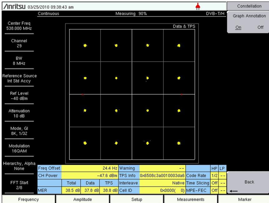
Figure 2-3. 16QAM with Hierarchy set to None
