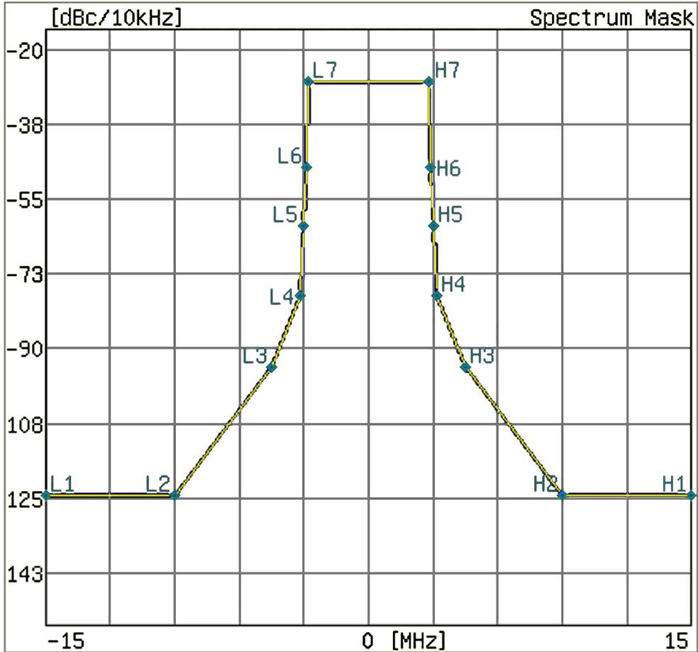
Figure 4-16. Critical Mask for UHF (Brazil) Channel Map
