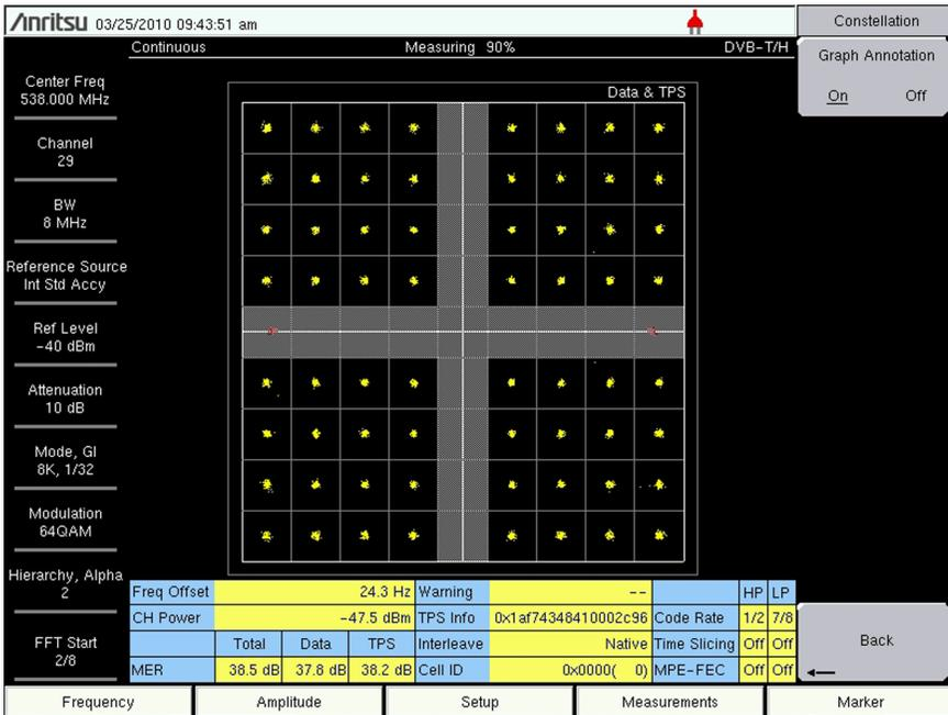
Figure 2-7. 64QAM with Hierarchy set to 2
