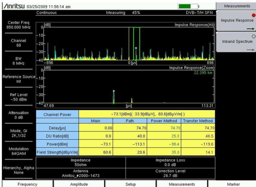
Figure 3-1. Impulse Response Measurement
