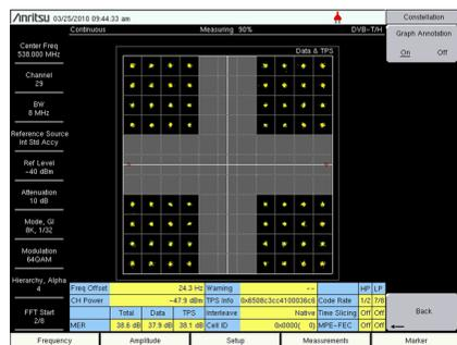
Figure 1-2. DVB-T/H Modulation and Hierarchy Settings
