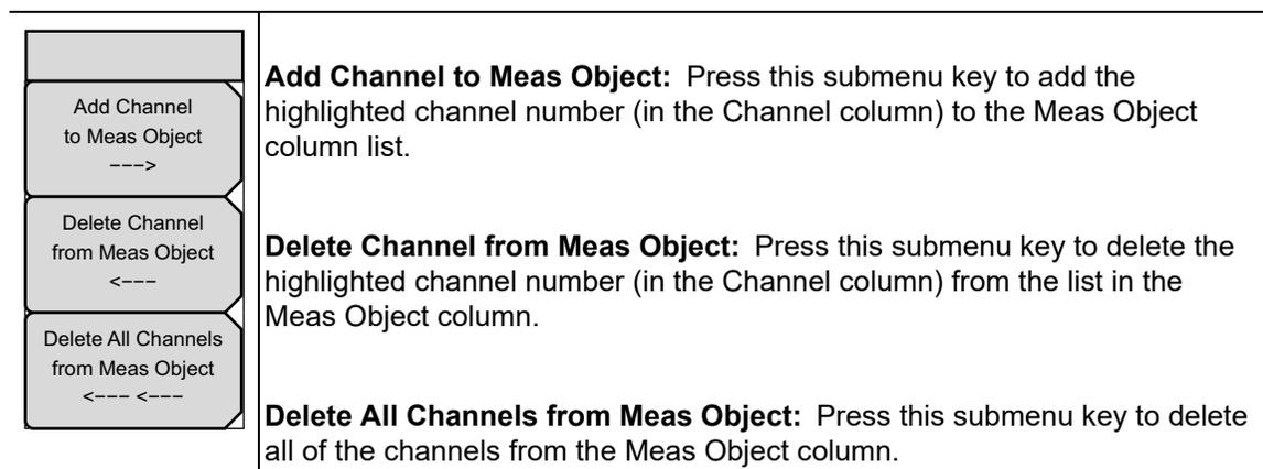
**Figure 4-7.** Select Channel Menu (Batch Measurement Mode)
