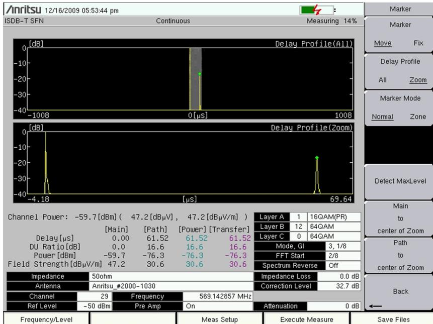
**Figure 5-1.** SFN Delay Profile Measurement
