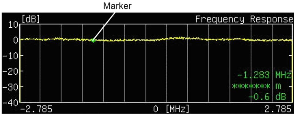
Figure 4-65. Frequency Response Graph with Standard Marker
