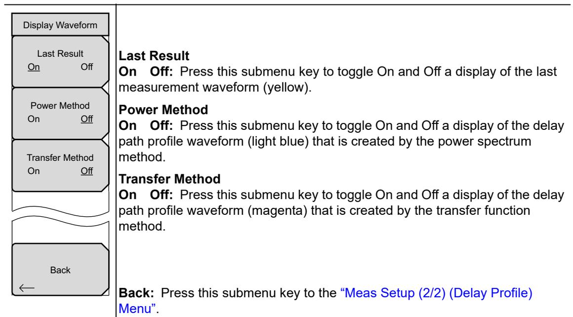
**Figure 5-16.** Display Waveform Menu
