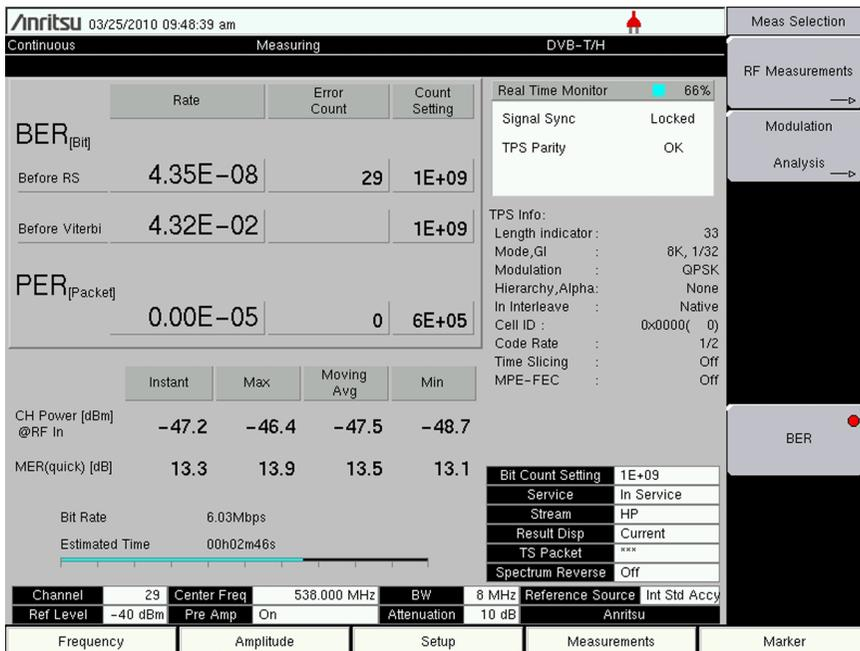
Figure 2-27. Bit Error Rate (BER) Measurements
