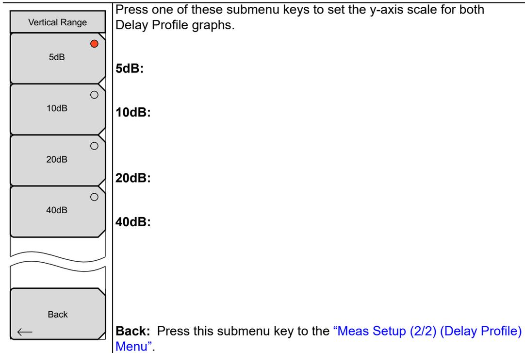
**Figure 5-15.** Vertical Range Menu (Delay Profile)
