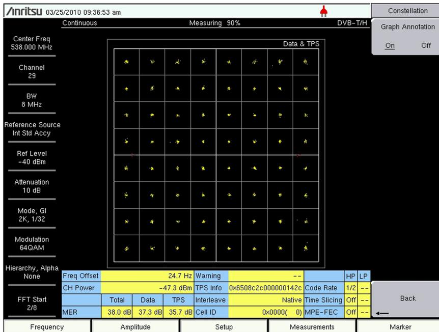
Figure 2-4. 64QAM with Hierarchy set to None
