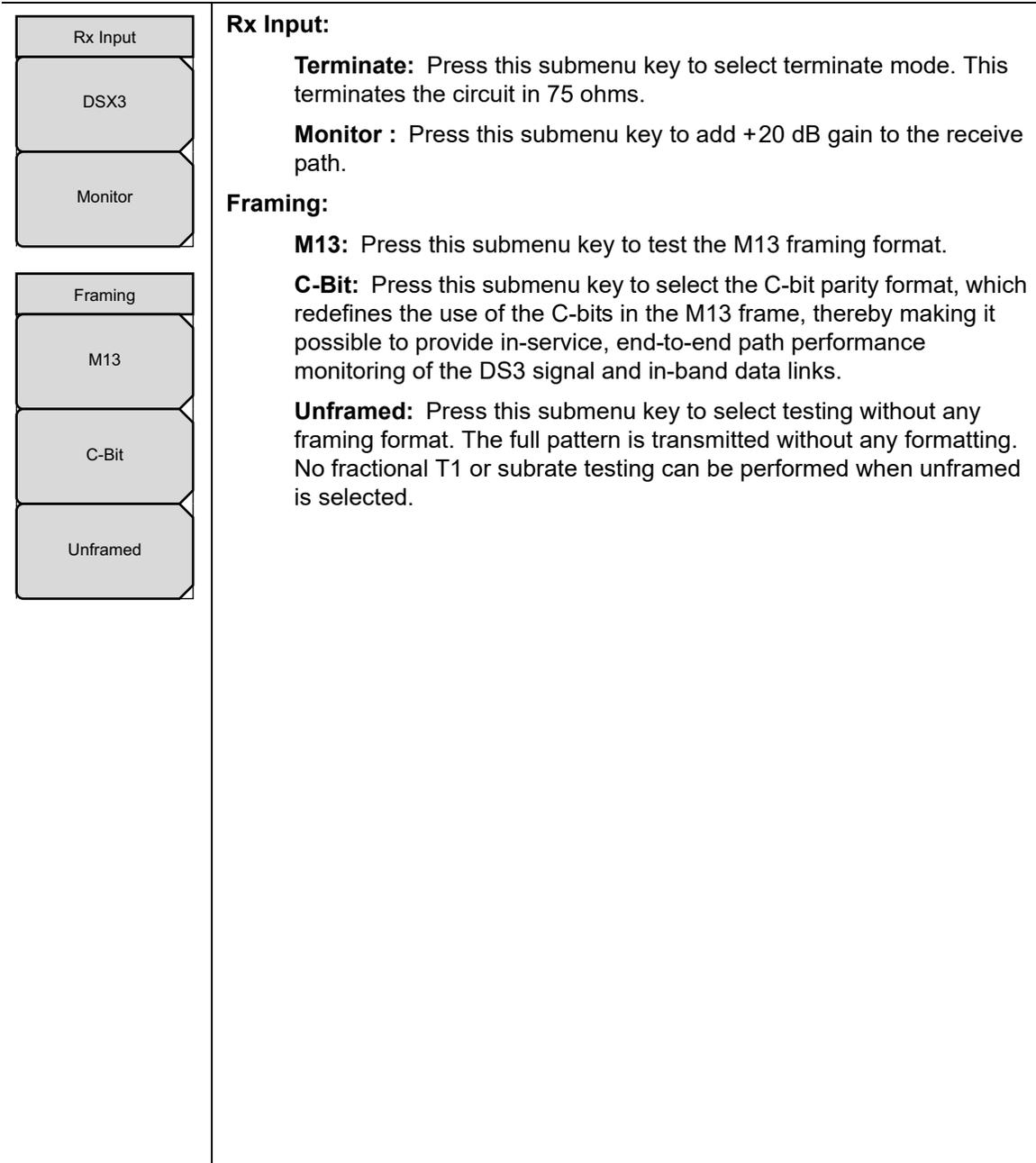
Figure 6-9. T3 Signal Setup (2 of 2)
