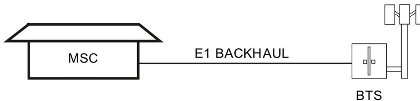
**Figure 2-4.** One Possible E1 - 2 Mb/s Network Topology
