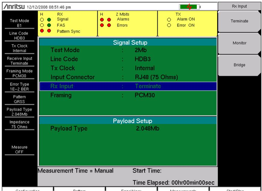
**Figure 2-9.** Configuration Rx Input
