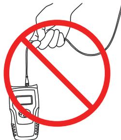
Be careful not to hit the end of an optical connector against anything hard such as the floor or a desk by dropping the optical fiber cable.
