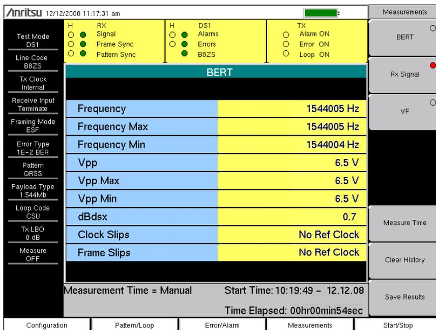
Figure 5-7. Vpp Measurement
