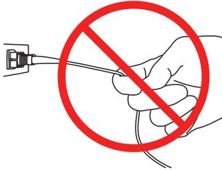
Do not excessively bend, fold, or pinch an optical fiber cable.
