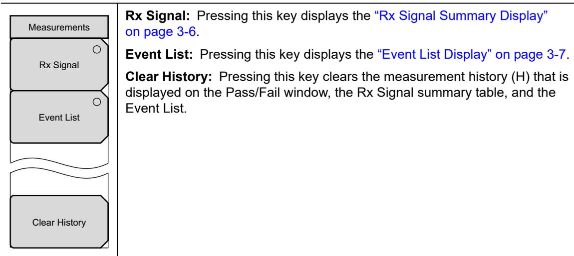
Figure 3-15. Measurements Menu
