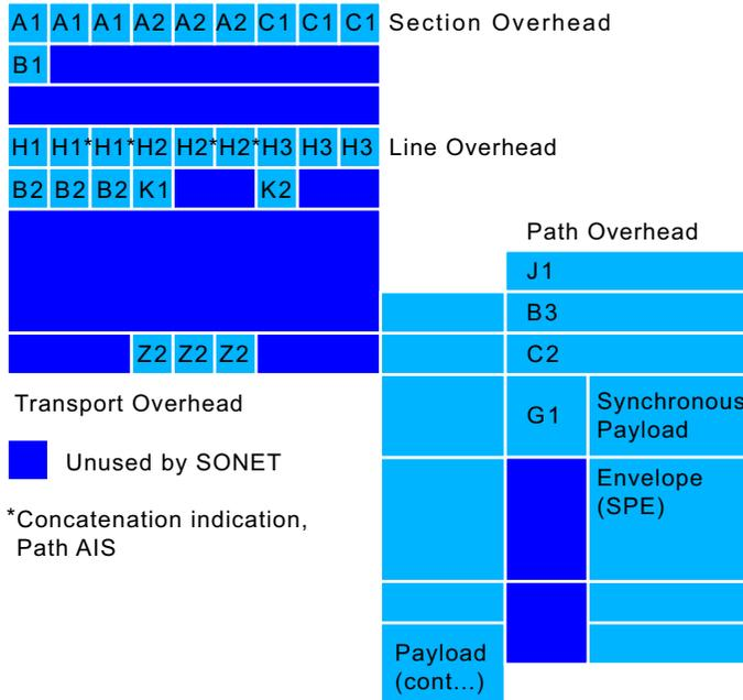
**Figure 3-2.** OC-3c Frame Structure
