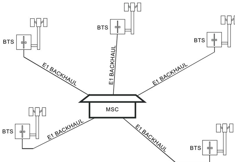
**Figure 2-1.** Typical Wireless Network Backhaul E1 - 2 Mb/s Link
