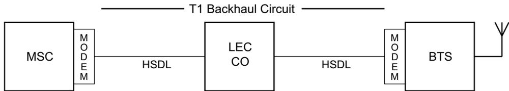
**Figure 5-3.** BTS and MSC Configuration
