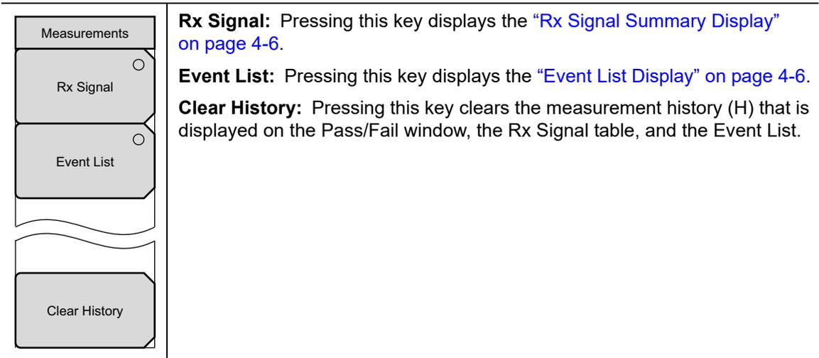
Figure 4-16. Measurements Menu
