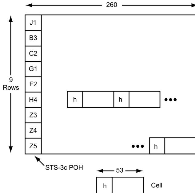
Figure 3-3. OC-3c POH & Payload, Not Including the TOH
