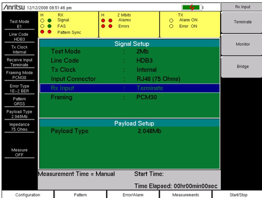
**Figure 2-6.** Configuration Setup
