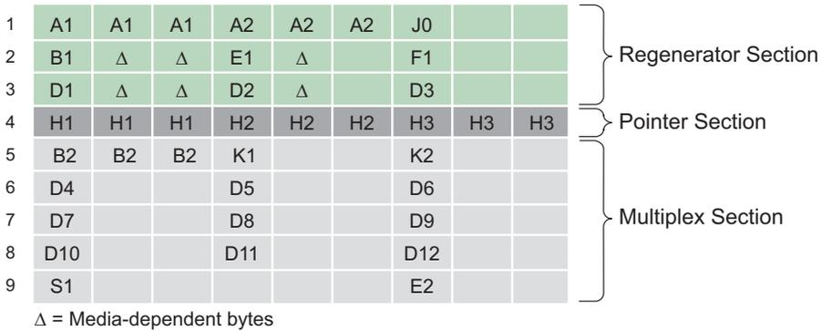
Figure 4-2. STM-1 Overhead Structure
