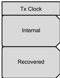
**Internal:** The transmit clock uses the internal clock oscillator (155.52 MHz).
