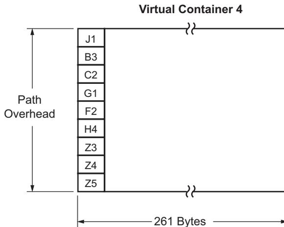
Figure 4-3. Path Overhead and Virtual Container 4 Payload Structure
