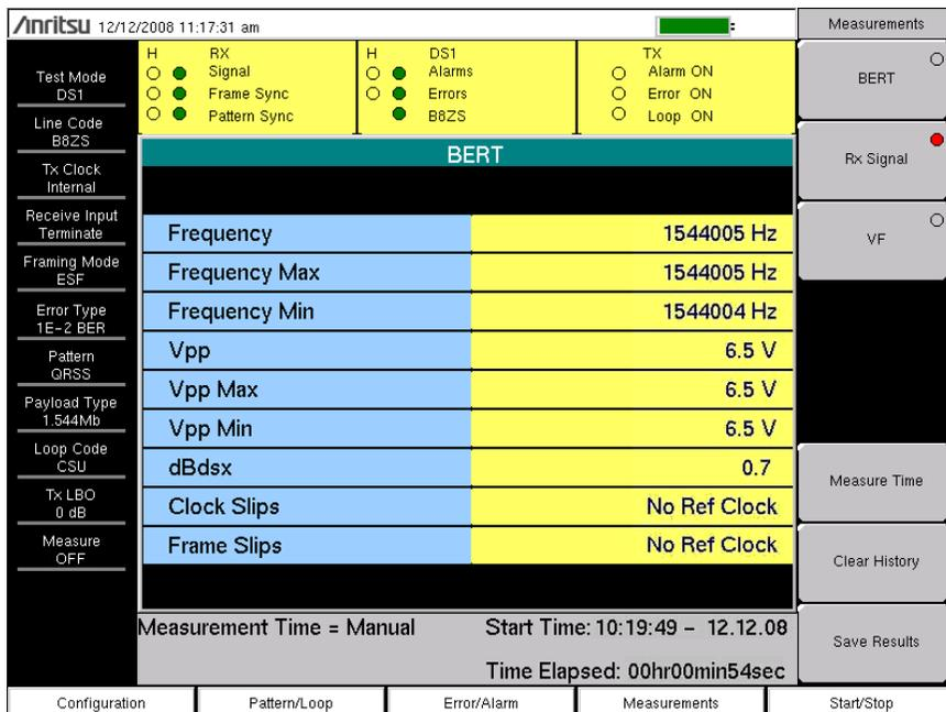
**Figure 5-8.** Vpp Out-of-Service Measurement
