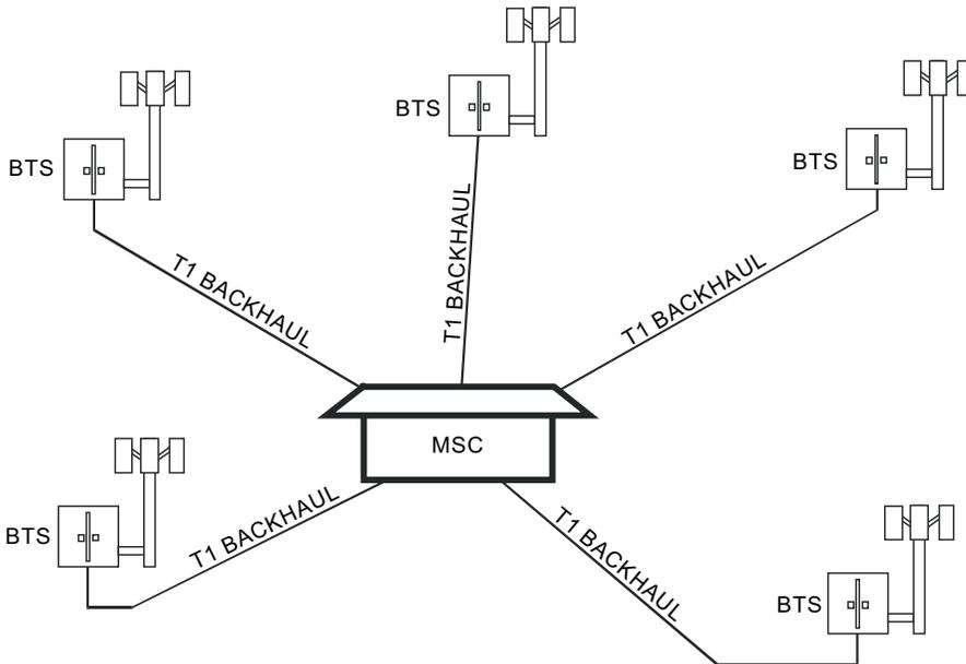
**Figure 5-1.** Typical Wireless Network T1 Backhaul Links
