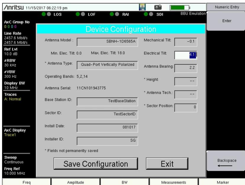
Figure 2-25. Electrical Tilt Entry
