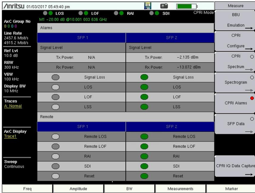
Figure 2-59. CPRI Alarms Screen (Dual-Port Model Is Shown)
