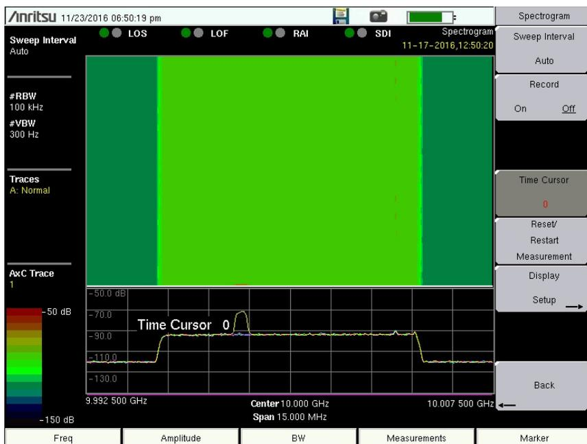
**Figure 2-6.** CPRI Spectrogram Display
