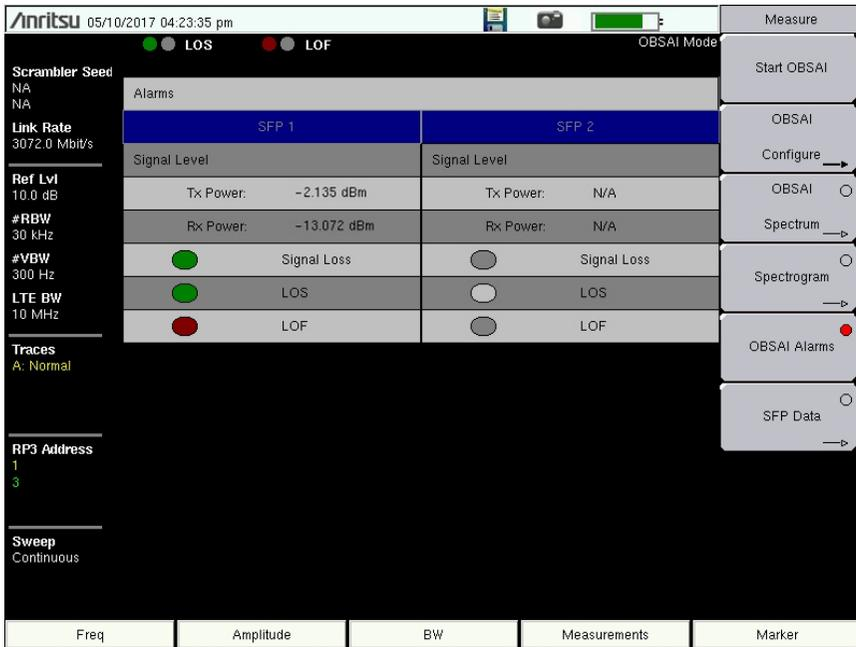
Figure 2-22. OBSAI Alarms Screen (dual-SFP Model Is Shown)
