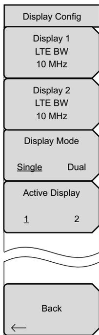
**Display 1 LTE BW:** This is the LTE carrier bandwidth for Display 1. Press this key to display the Select Bandwidth list box illustrated in [Figure 2-25](#). Use the touch screen, arrow keys, or rotary knob to highlight the LTE carrier bandwidth, then press **Enter**. Selectable values are 5 MHz, 10 MHz, 15 MHz, and 20 MHz.
