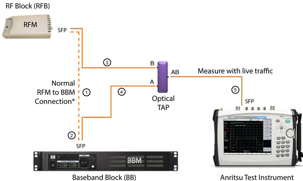
\* Lock down the Radio before disconnecting fiber from BBM
