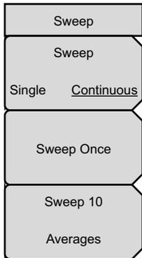
**Sweep Single/Continuous:** This submenu key toggles between continuous sweep and single sweep. In single sweep mode, the results of a sweep are displayed on the screen while the instrument awaits a trigger event to start a new sweep.
