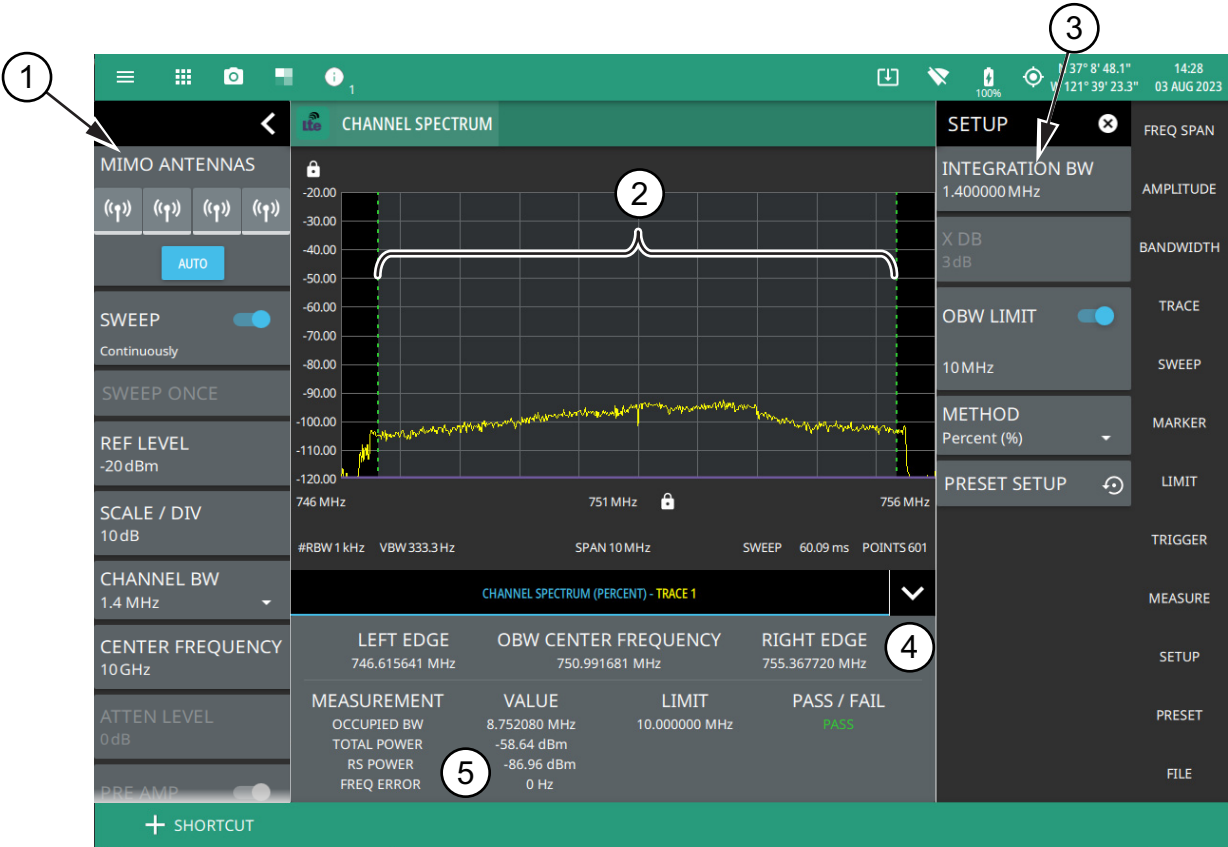
Figure 2-41. LTE Channel Spectrum (Occupied Bandwidth) Measurement (1 of 2)
