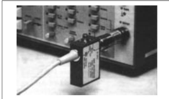
**Step 3.** Insert the compensation washer into the opening of the WSMA female connector, as shown.
