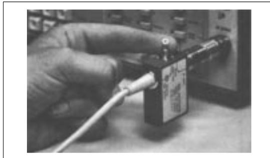
**Step 4.** Connect beaded end of the air line per application. Tilt the air line horizontally. At unbeaded end, center the inner conductor with the center of the connector opening.
