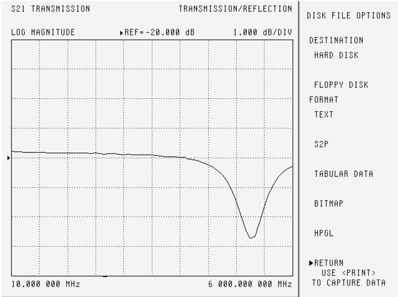
**Figure 2-3.** Example of a bad display response
