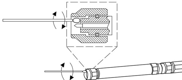
Use only denatured alcohol and the proper size of cotton swab. Gently rotate the swab around the center pin being careful not to stress or bend the pin or you will damage the connector.
