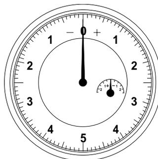
**Figure 3-2.** Pin Depth Gauge
