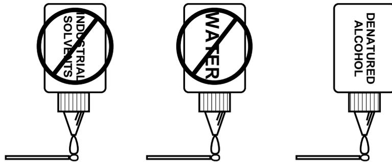
Do NOT use Industrial Solvents or Water on connector. Use only Denatured Alcohol.
