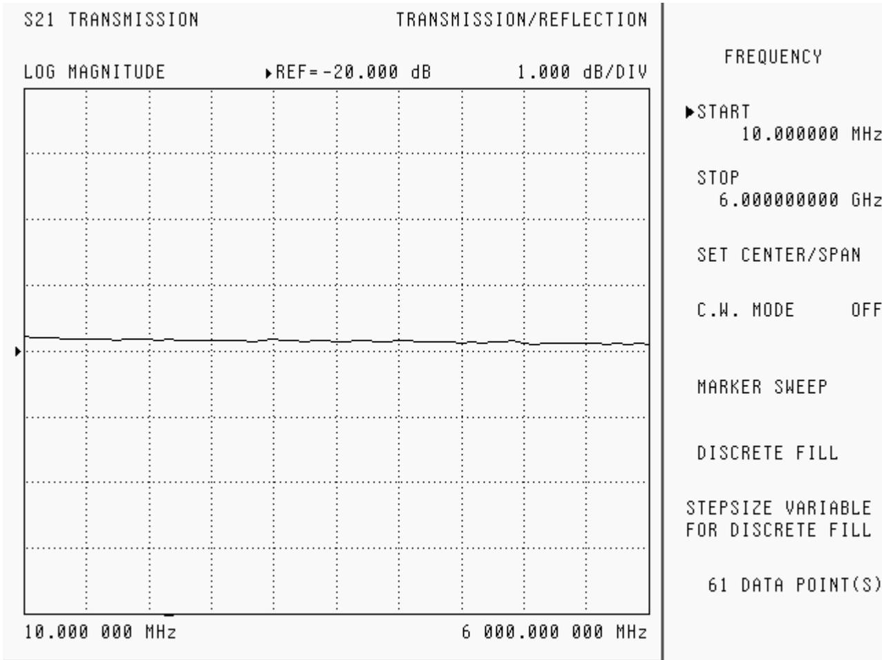
**Figure 2-2.** Example of a good display response
