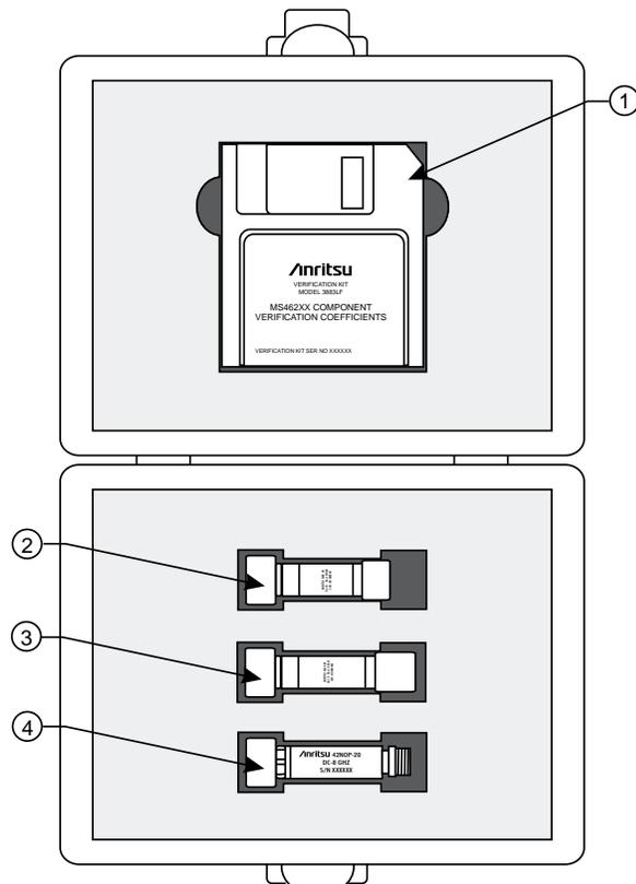
**Figure 1-1.** Model 3663LF (Type N) Verification Kit Components
