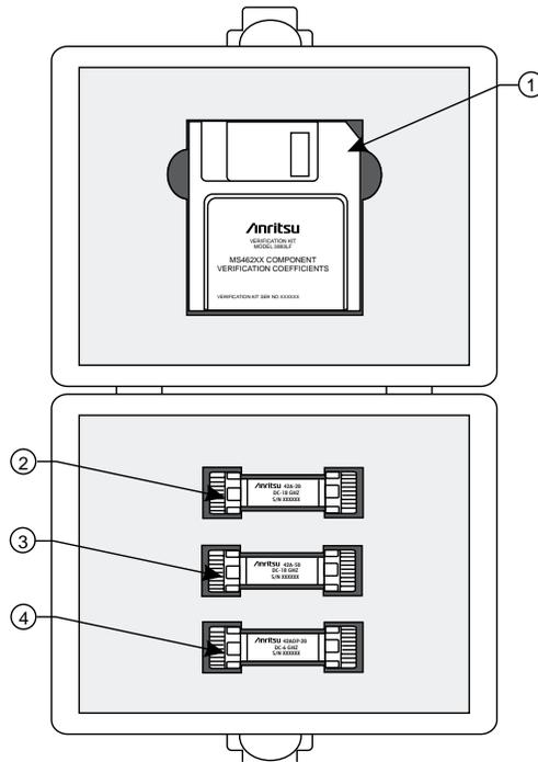
**Figure 1-3.** Model 3667LF (GPC 7) Verification Kit Components
