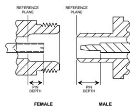
**Figure 3-1.** N Connector Pin Depth
