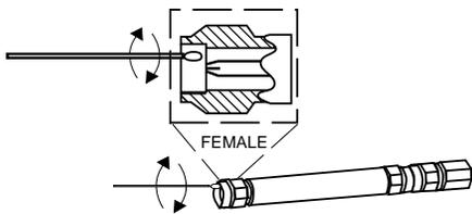
Figure 3-4 illustrates how to clean connectors.
