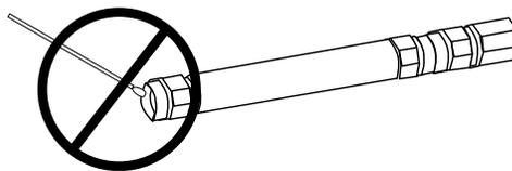
Do NOT put cotton swabs in at an angle, or you will damage the connectors.
