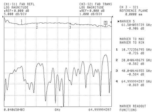
**Figure 4.** Typical V251 Insertion Loss and Return Loss, 40 MHz to 65 GHz
