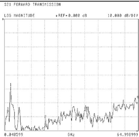
**Figure 3.** Typical Isolation between Data I/P and DC Port
