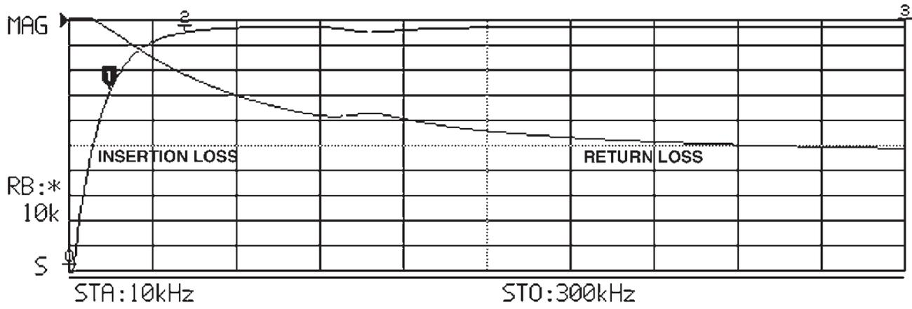
**Figure 2.** Typical V255 Insertion Loss and Return Loss, 1 kHz to 1 MHz
