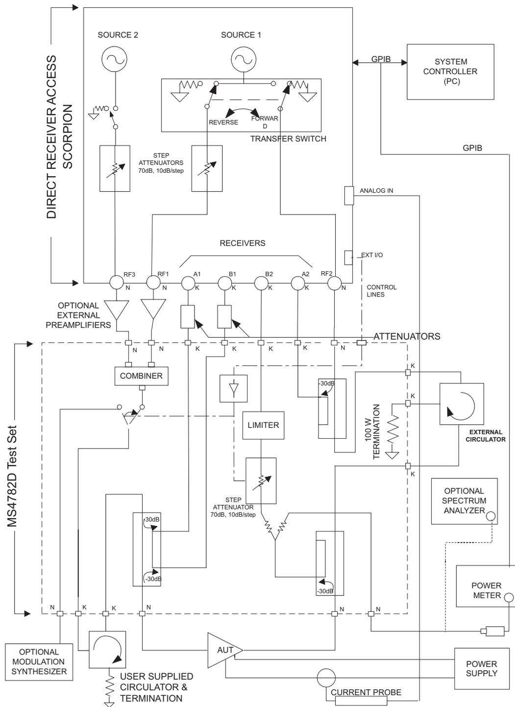
Figure 7-1. MS4782A with External Preamplifiers (Moderate Power)
