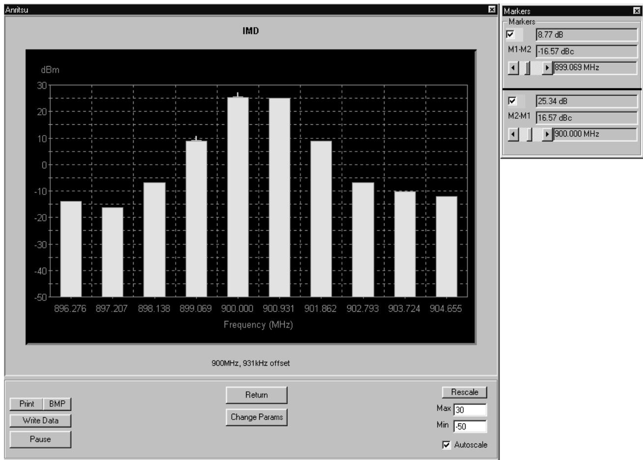
**Figure 5-6.** Intermodulation Distortion Test Screen
