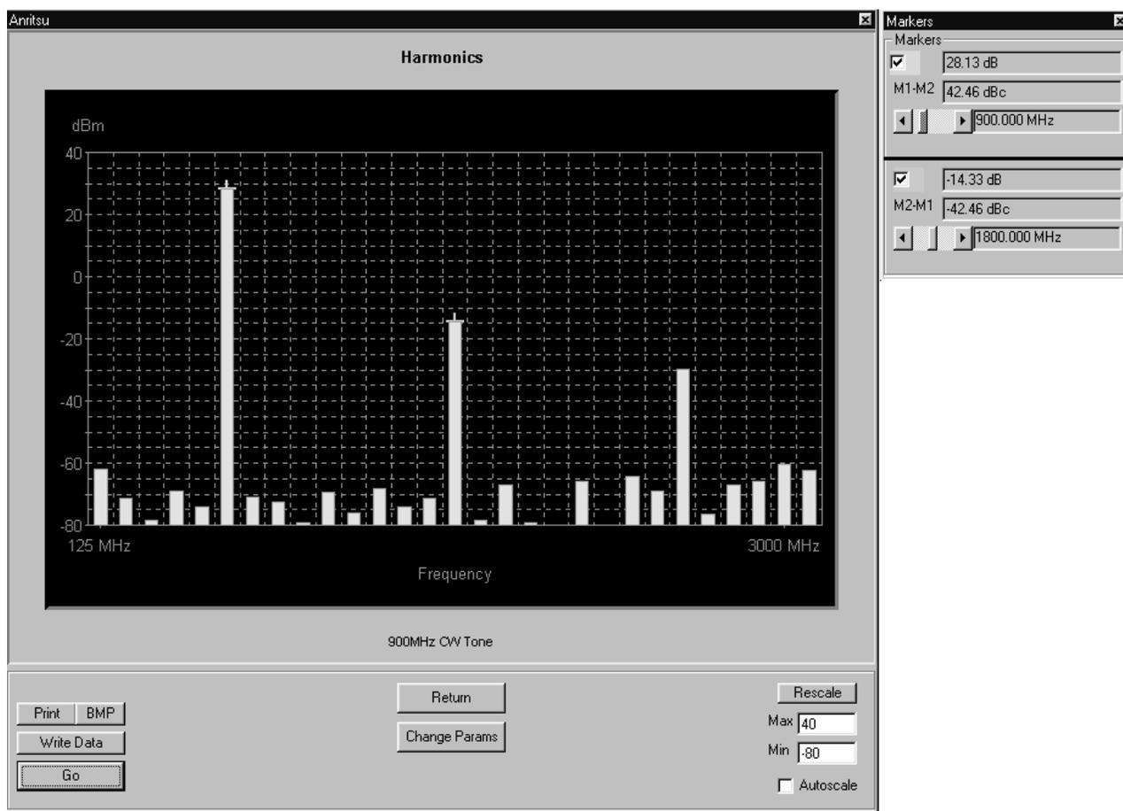
Figure 5-7. Initial Harmonics Test Screen
