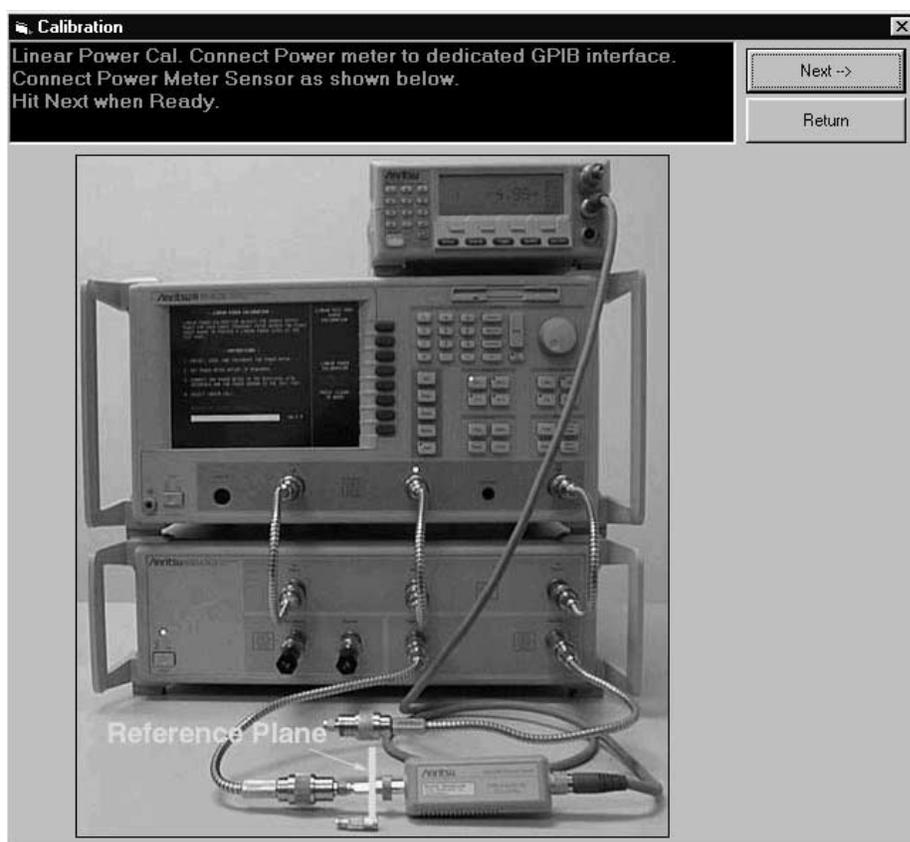
**Step 6.** Before hitting the “Next” button, connect the power meter to at the point where power enters the device-under-test (AUT), which becomes the power reference plane as shown in the prompt.
