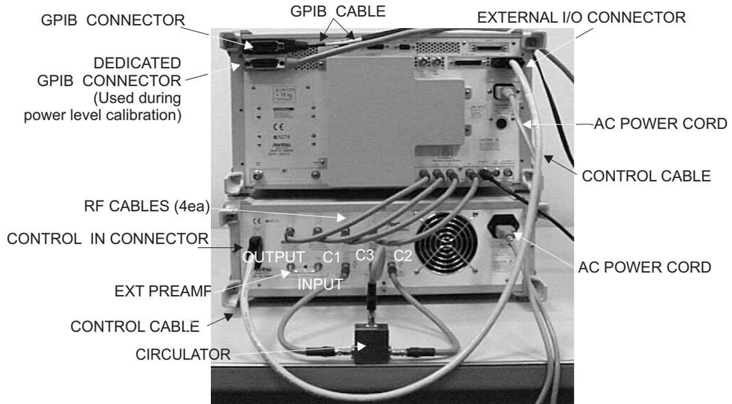
**Figure 2-2.** ME7840A Rear Cable Connections
