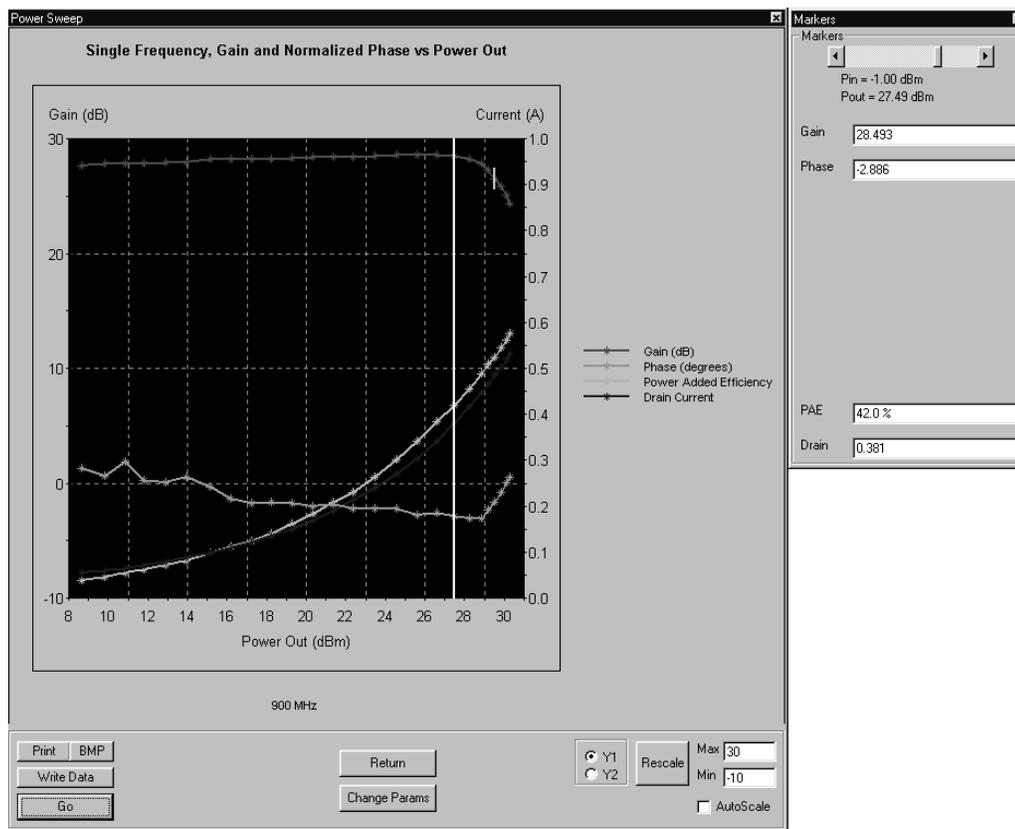
Figure 5-5. Single Frequency Power Sweep Test
