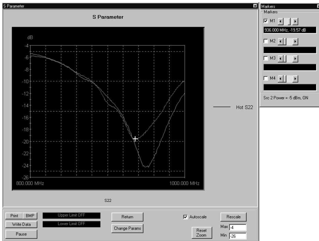
**Figure 5-8.** Hot  $S_{22}$  Test Screen
