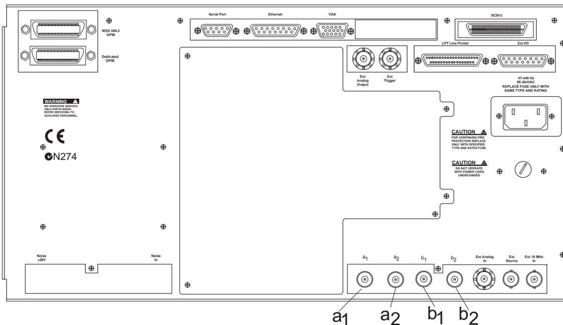
Figure 1-4. MS462XC Rear Panel Showing Ports a<sub>1</sub>, a<sub>2</sub>, b<sub>1</sub>, and b<sub>2</sub>
