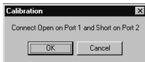
**Step 20.** Press “OK” for the next step (below). Connect the Short to Test Port 1 and the Open to Test Port 2.
