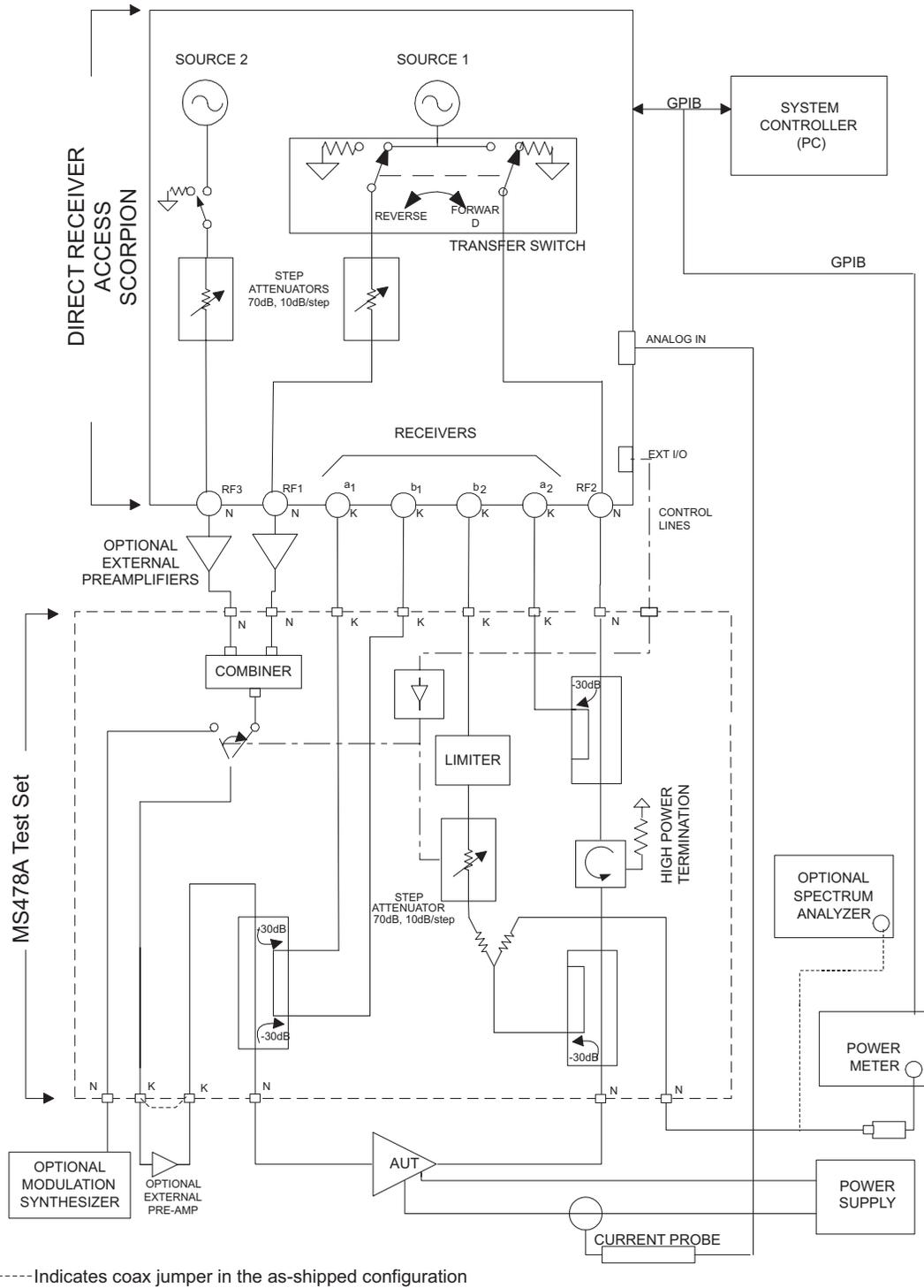
**Figure 1-3.** Overall Functional Block Diagram of the Option 2 Power Amplifier Test System (PATS) with MS4782A Test Set
