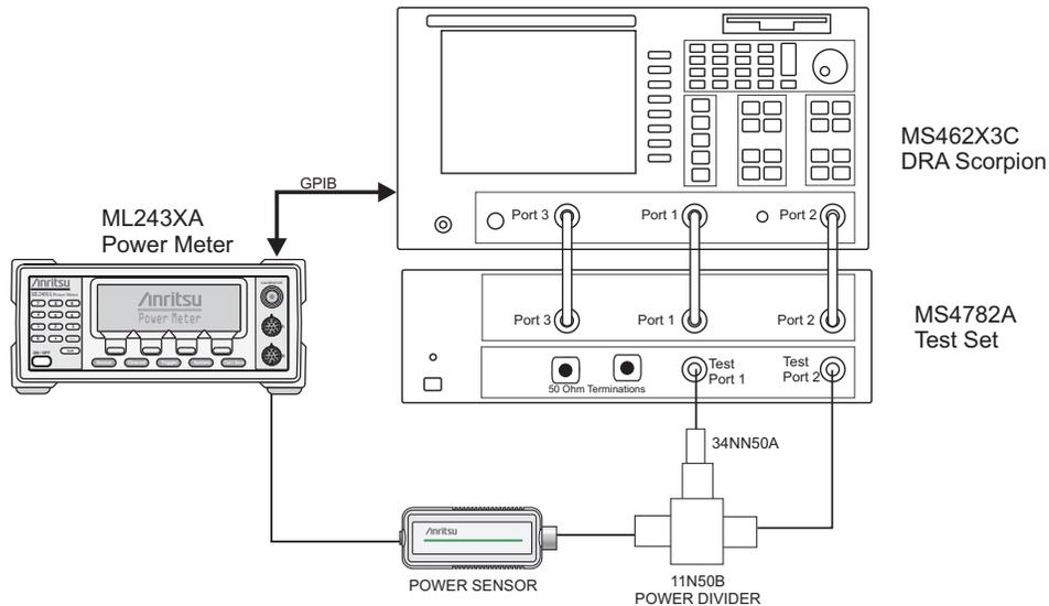
**Figure 6-2.** Receiver Magnitude Display Linearity Test Setup
