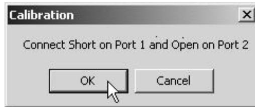
**Step 19.** Press OK for the next step (below). Connect the throughline between Port 1 and Port 2.
