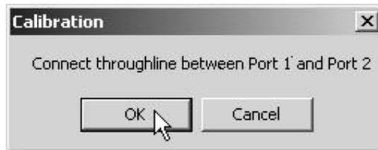
**Step 20.** Press OK to complete the Hot S22 calibration.
