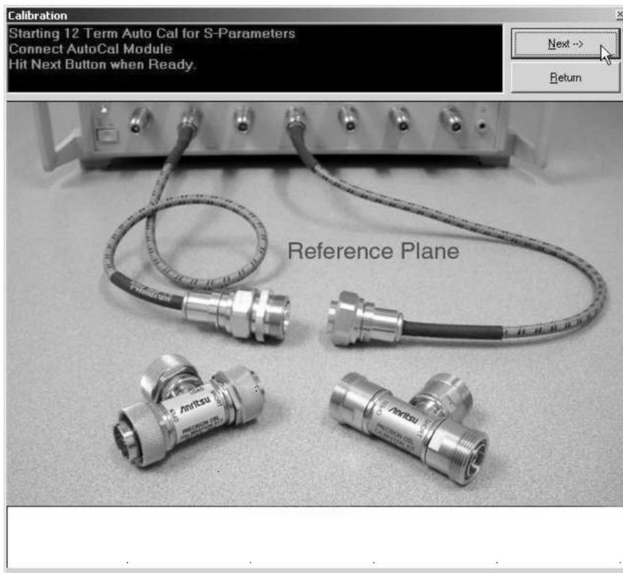
**Step 22.** Press Next for the next step (below). The 3753R Calibration Kit contains a disk with calibration data. The data has to be installed from the MS4623B front panel. To do so, place the floppy disk from the kit into the MS4623B disk drive. Press the Cal key then COMPONENTS UTILITIES/INSTALL KIT INFO FROM FLOPPY DISK softkeys.
