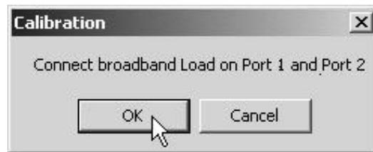
**Step 24.** Press OK for the next step (below). Connect the Open to Port 1 and the Short to Port 2.
