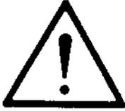
Always refer to the operation manual when working near locations at which the alert mark, shown on the left, is attached. If the operation, etc., is performed without heeding the advice in the operation manual, there is a risk of personal injury. In addition, the equipment performance may be reduced. Moreover, this alert mark is sometimes used with other marks and descriptions indicating other dangers.
