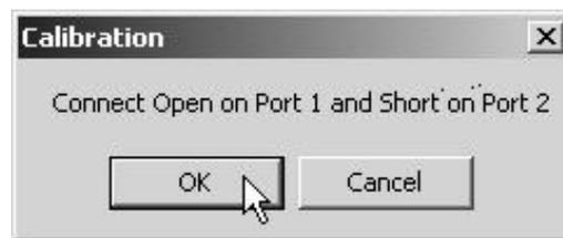
**Step 25.** Press OK for the next step (below). Connect the Short to Port 1 and the Open to Port 2.
