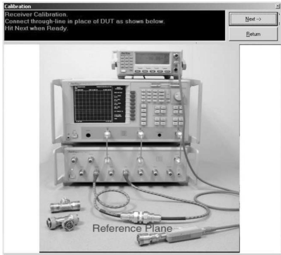
**Step 12.** Press Next to perform a Receiver Calibration.
