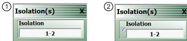
The button above left shows the test has not been started. The user makes the necessary physical connections between the VNA and the required connector/adaptor, and then clicks the button to begin the test. The button dims while the test is performed. After the test is successfully completed, the completion icon appears on the left side of the button as shown above right.
