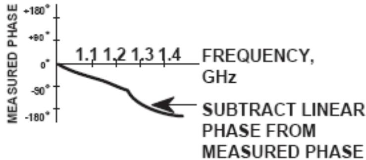
**Figure A-12.** Phase Difference Increases Linearly with Frequency
