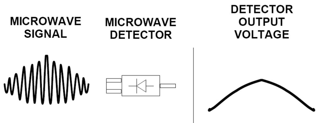
DETECTOR OUTPUT VOLTAGE IS PROPORTIONAL TO SIGNAL AMPLITUDE.
