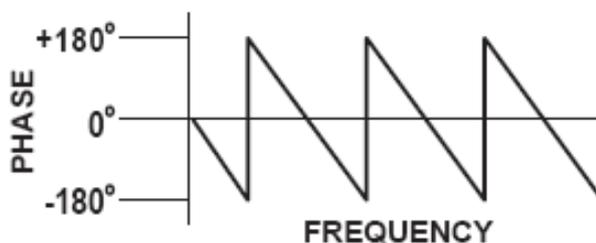
**Figure A-15.** Linear Phase with Frequency Waveform
