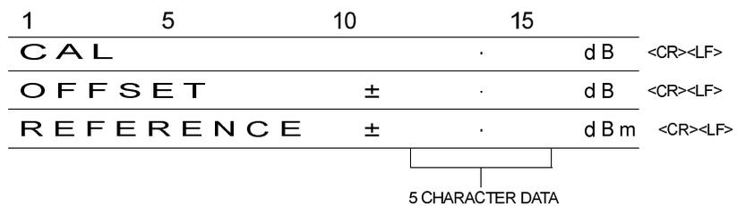
Figure 6-3. ODT Data Output Format
