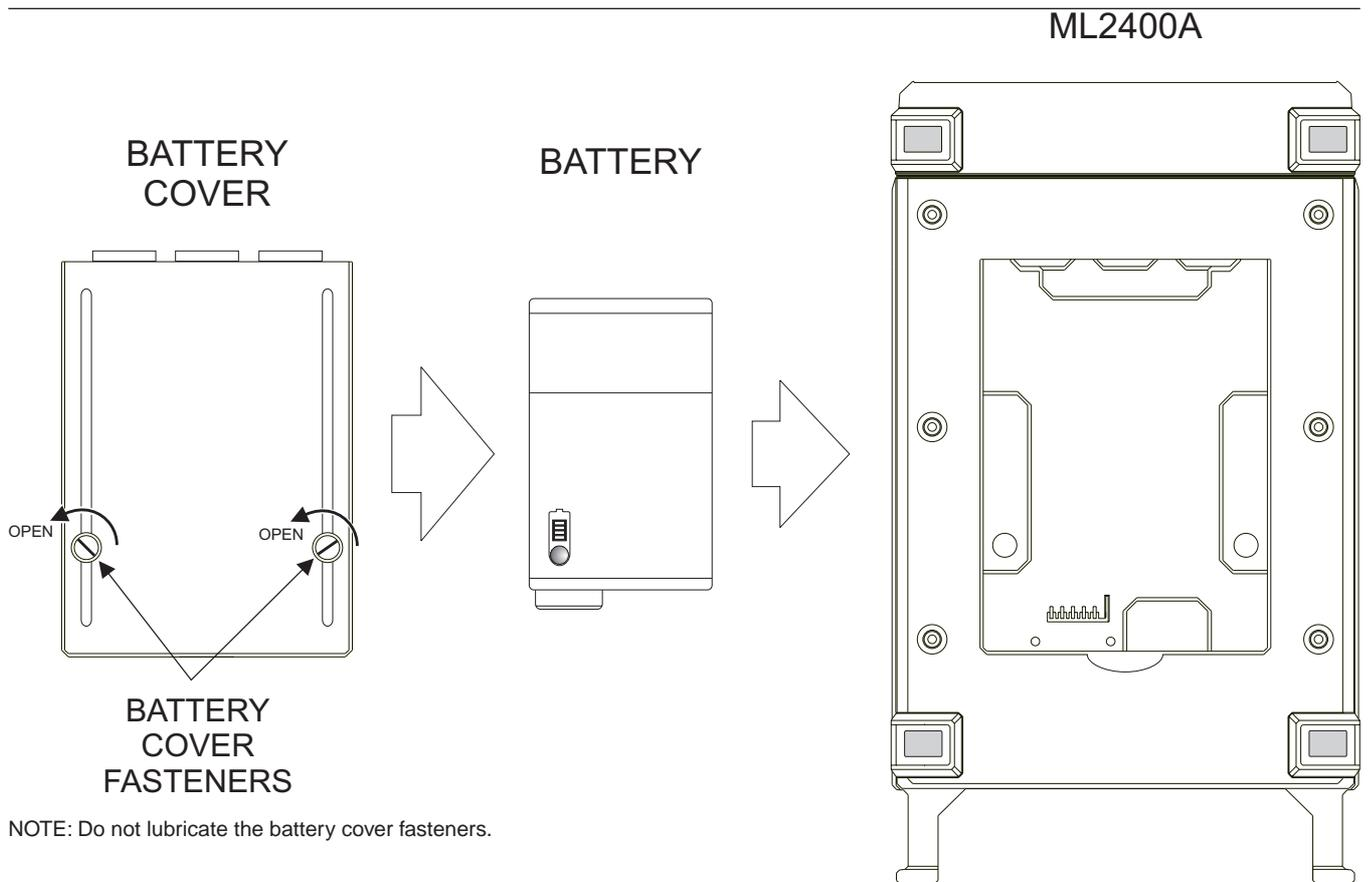
NOTE: Do not lubricate the battery cover fasteners.
