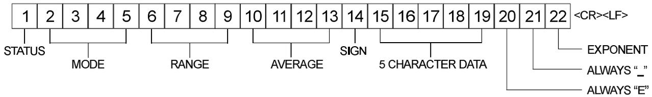
Figure 6-5. OPW Data Output Format
