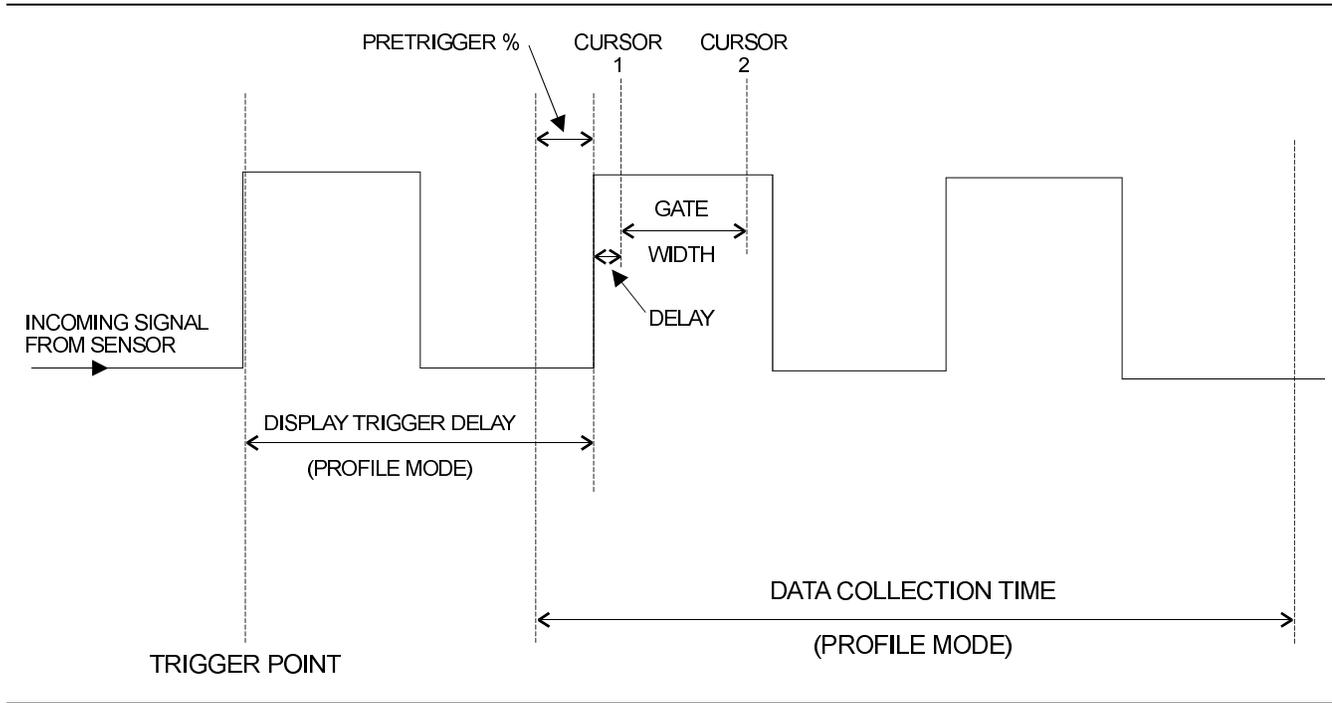
Figure 4-4. Sample Trigger in Graphic Mode
