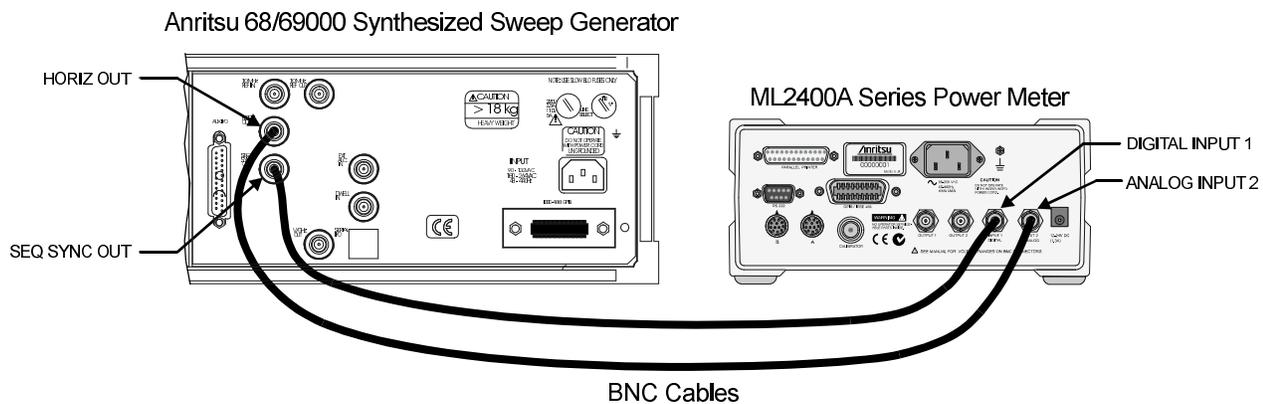
**Figure 4-5.** Source Sweep Mode Interconnection Example
