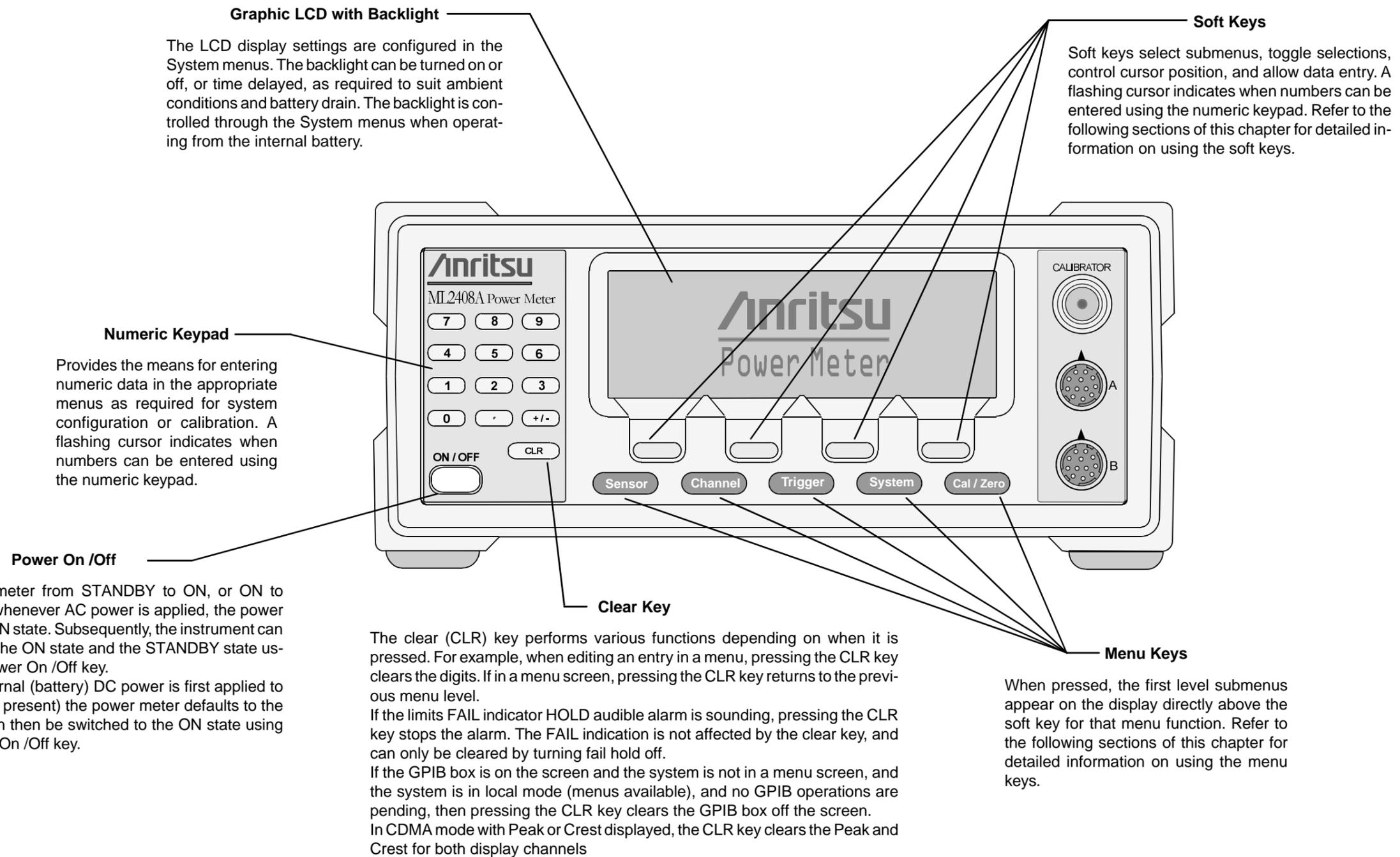
Figure 4-1. ML2400A Series Front Panel Controls
