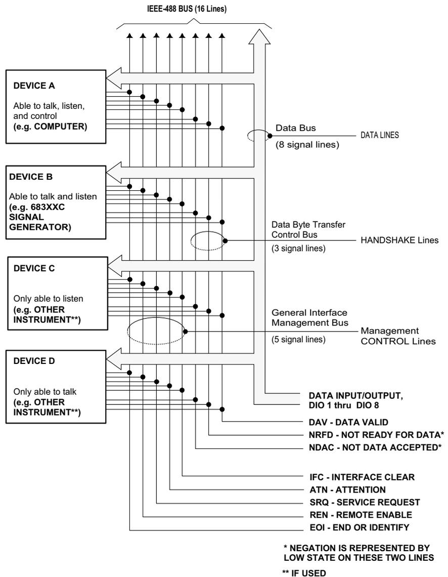
**Figure 1-1.** Interface Connections and GPIB Bus Structure
