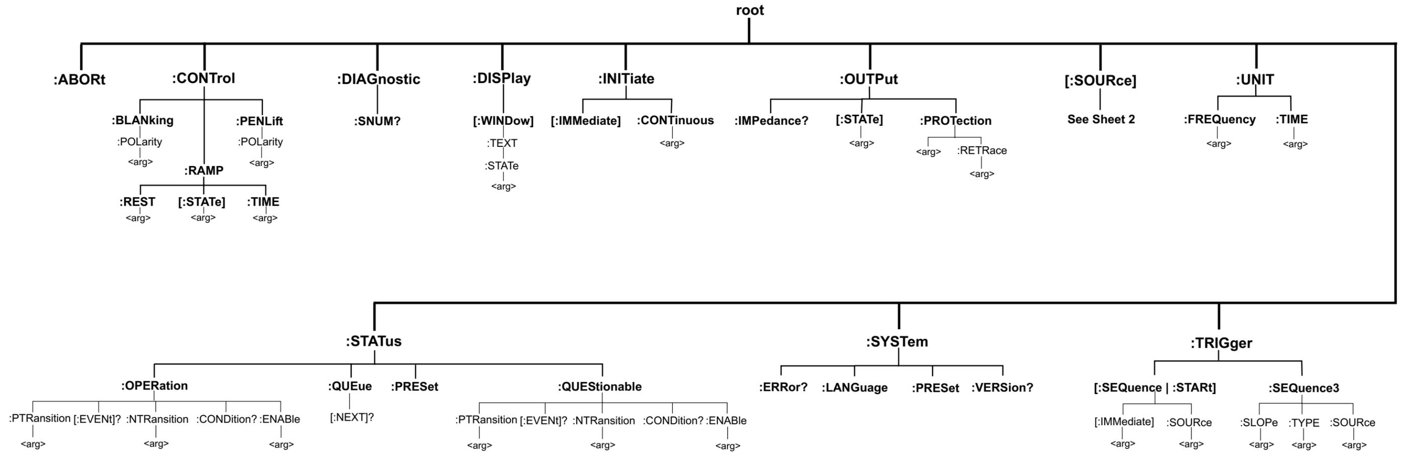
**Figure A-1.** Overall MG369XA SCPI Command Tree (Sheet 1 of 2)
