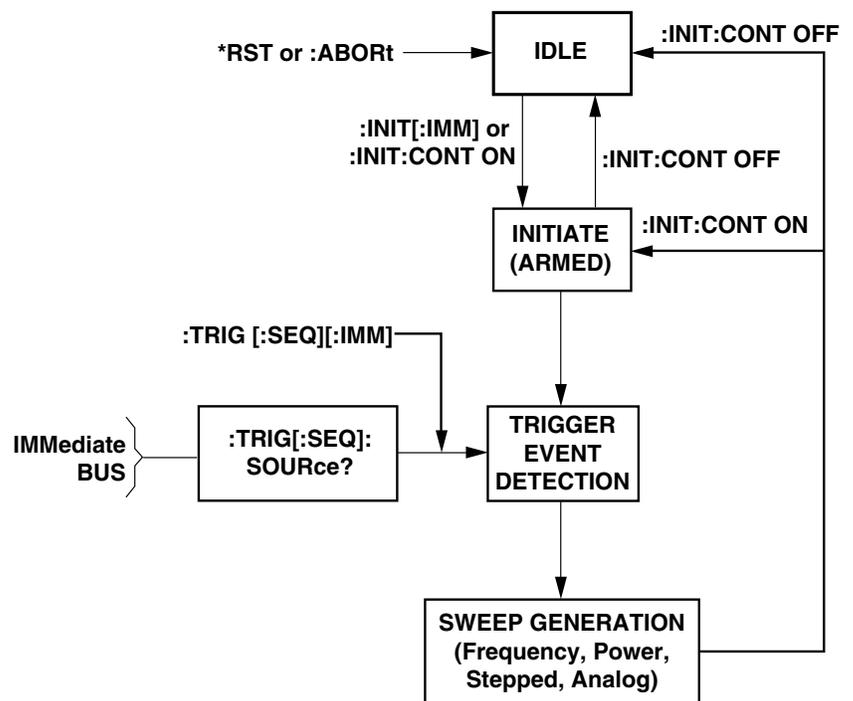
**Figure 2-2.** MG369XA Trigger Model
