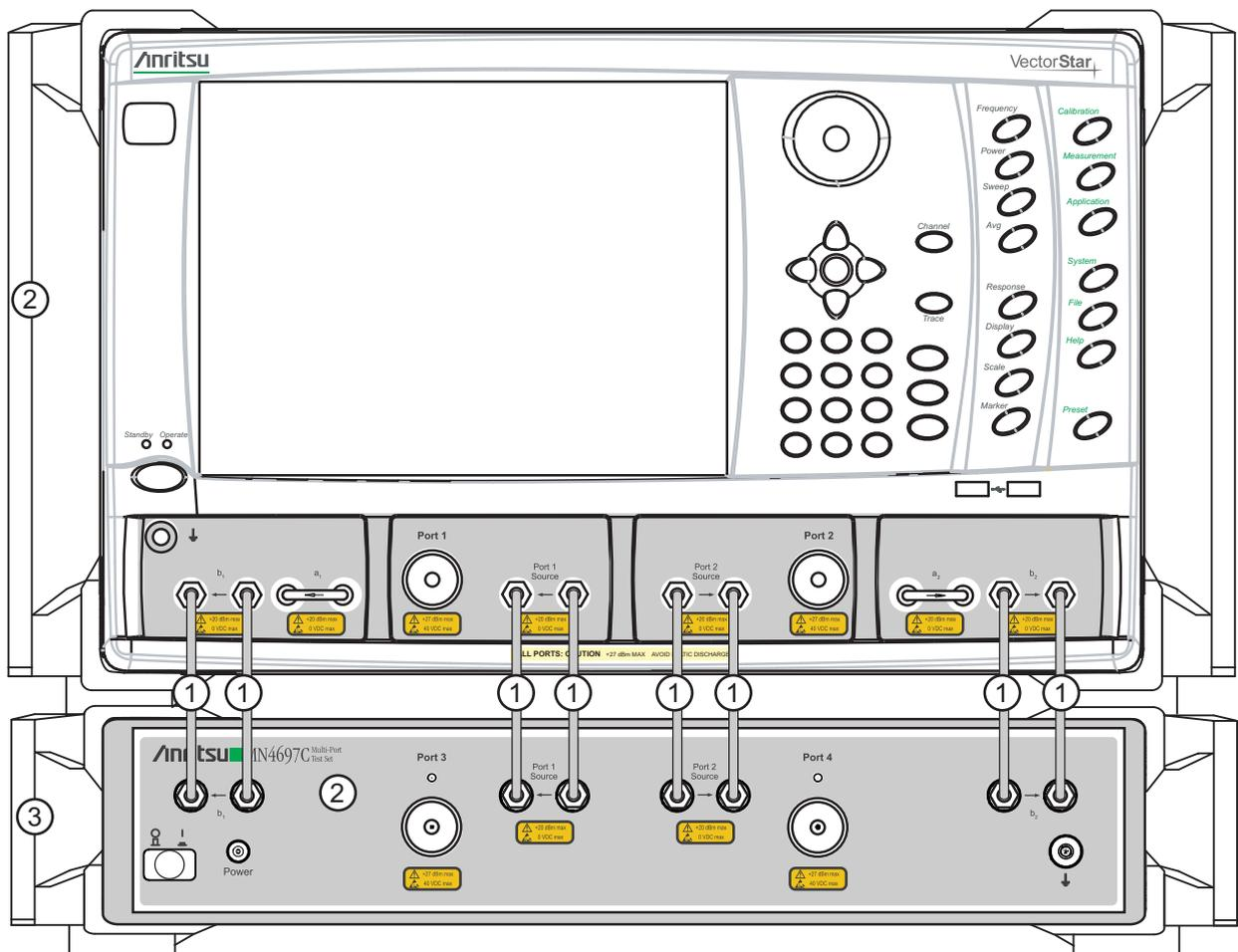
**Figure 1.** MS464xA/B VNA and MN469xC Test Set Front Panel Connections
