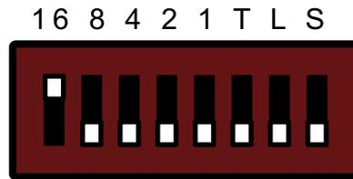
**Figure 3.** MN469xC DIP Switches (factory setting)
