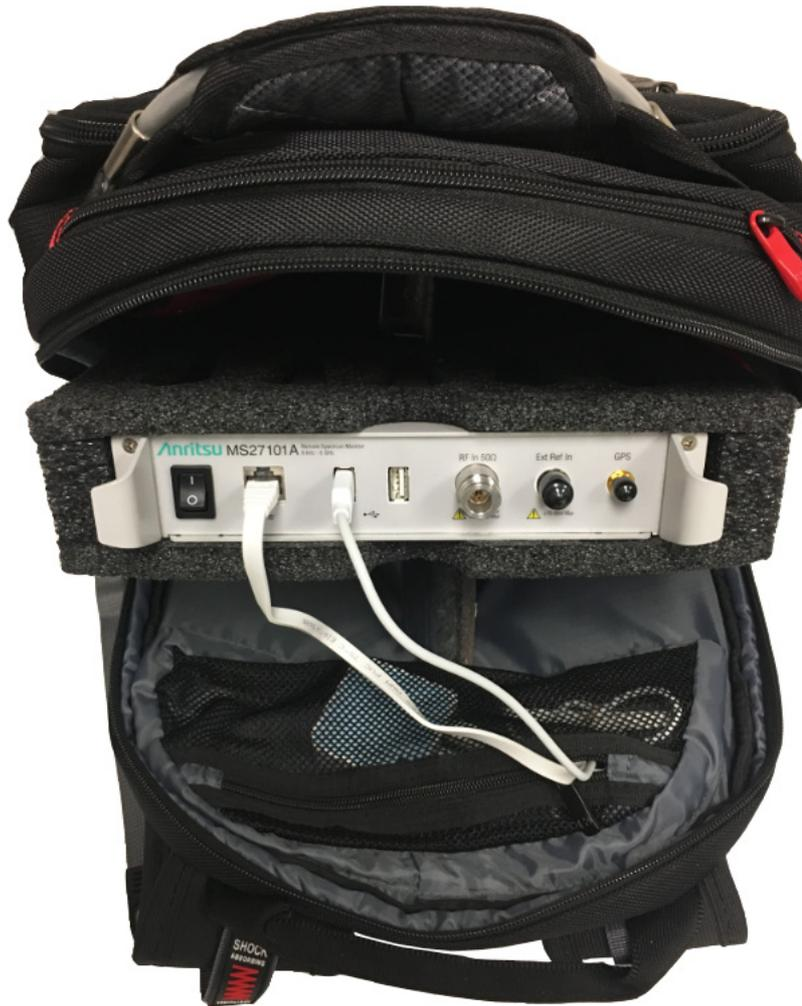
**Figure QSG-10.** Router Fitted Inside Backpack
