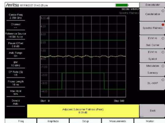
**Spectral Flatness** is a check for un-even amplitude of sub-carriers. The overall flatness of the signal is checked by the mask.
