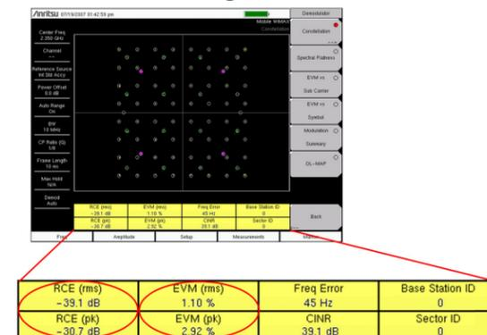
**RCE and EVM** measure the difference between the actual and ideal signal. RCE is measured in dB and EVM in percent.
