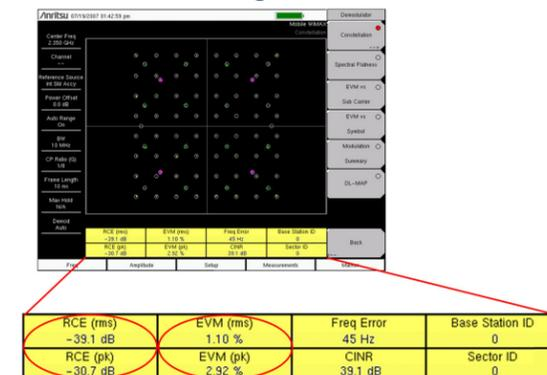
**RCE and EVM** measure the difference between the actual and ideal signal. RCE is measured in dB and EVM in percent.
