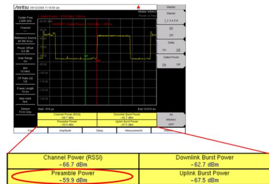
**Preamble Power** set cell size. A 1.5 dB change in power levels means a 15% change in coverage area. Coverage is directly affected by preamble power settings.
