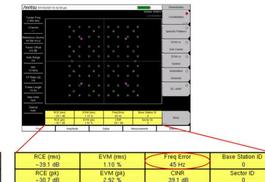
**Frequency Error** is a check to see that the carrier frequency is precisely correct.
