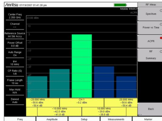
**Adjacent Channel Power Ratio (ACPR)** measures how much BTS signal gets into neighboring RF channels. ACPR checks the closest (adjacent) and the second closest (alternate) channels.
