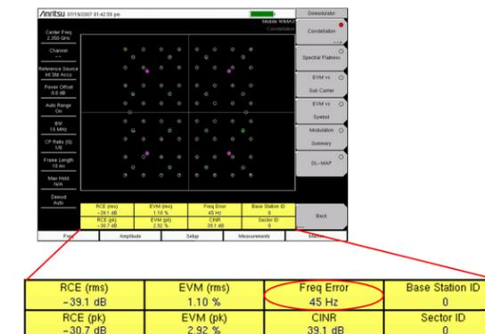
**Frequency Error** is a check to see that the carrier frequency is precisely correct.
