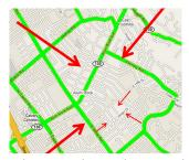
directional antenna, such as a Yagi, tuned to the band of interest. The DF process involves taking a series of directional readings, or bearings, of the suspect signal and recording those readings on a map. By
