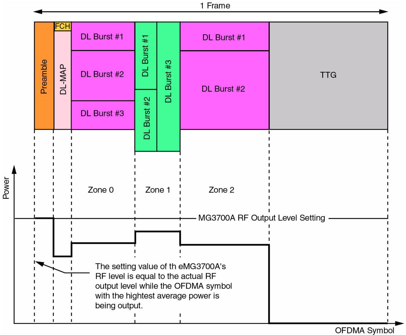
Figure 2-42. Power Per Symbol and MG3700A's RF Output Level
