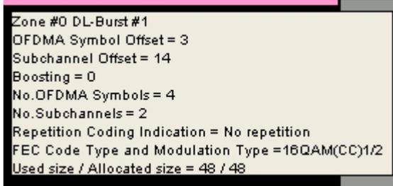
Figure 2-41. Example of Burst Area Information Display
