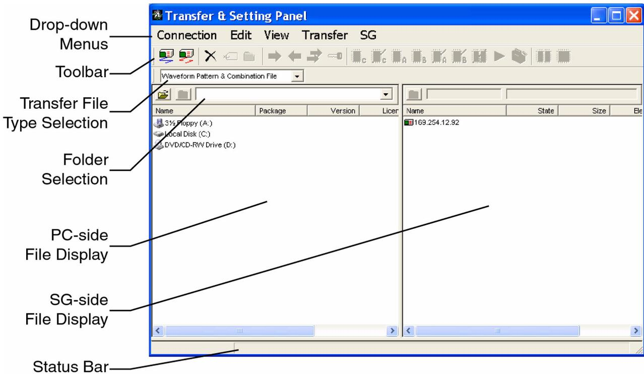
**Figure 2-53.** Transfer & Setting Panel Screen
