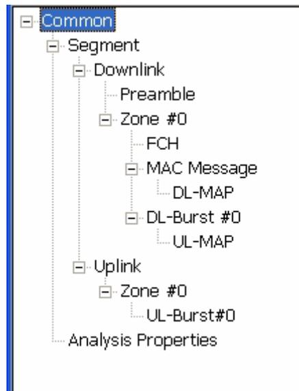
**Figure 2-32.** Typical OFDMA Tree View
