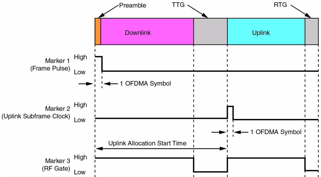
**Figure 3-23.** Auxiliary Signal Output Timing
