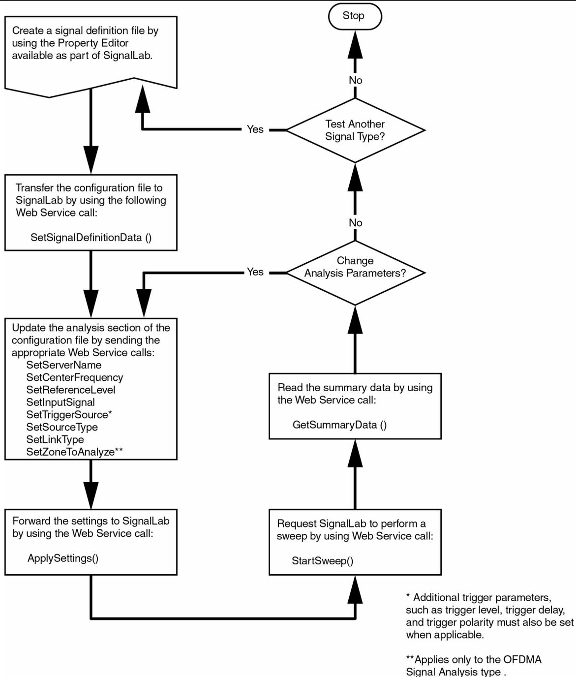
Figure 3-24. Remote Control Programming Flow Chart
