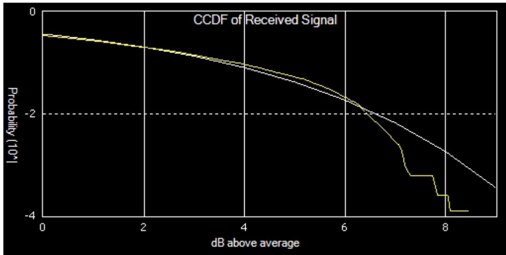
Figure 2-10. CCDF of Received Signal Viewer
