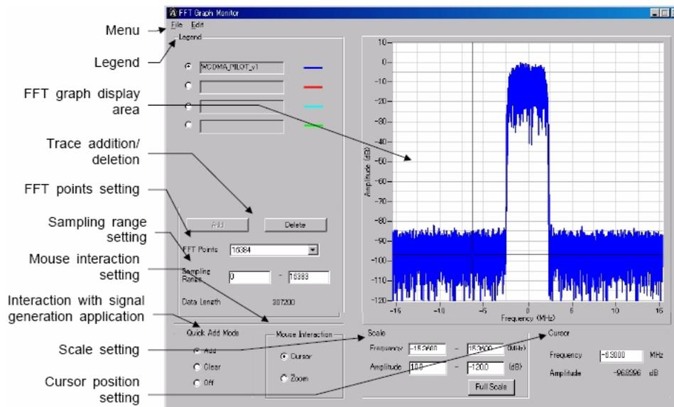
**Figure 2-48.** FFT Graph Display and Controls
