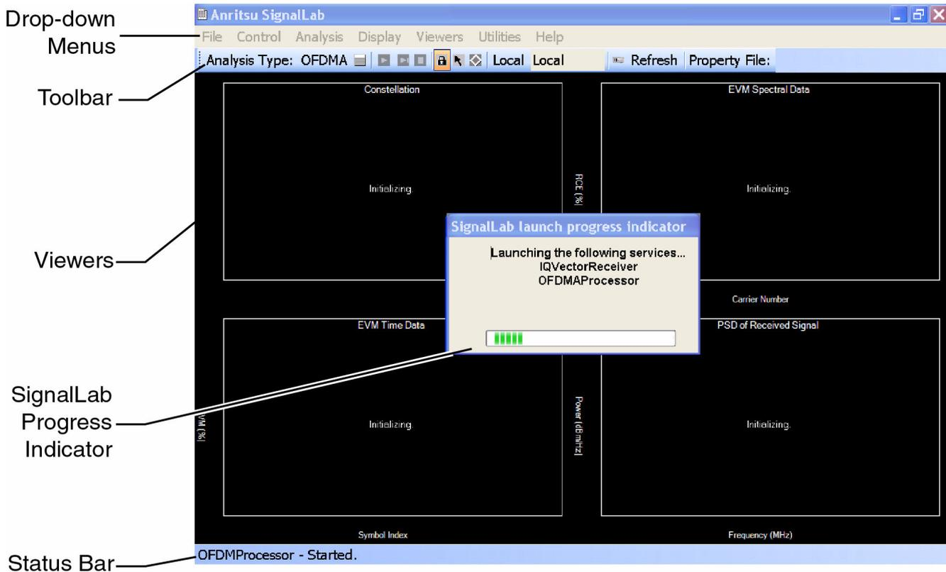
**Figure 2-2.** Main Anritsu SignalLab Display
