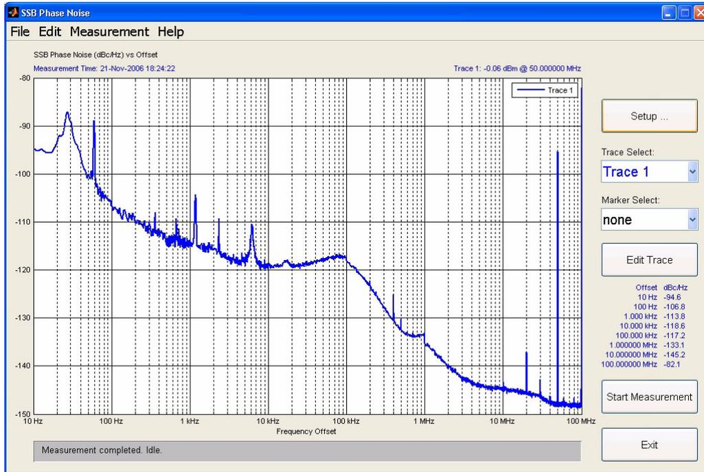
Figure 3-2. 50 MHz Phase Noise Measurement
