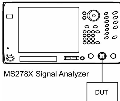
**Figure 3-1.** Phase Noise Measurement Setup
