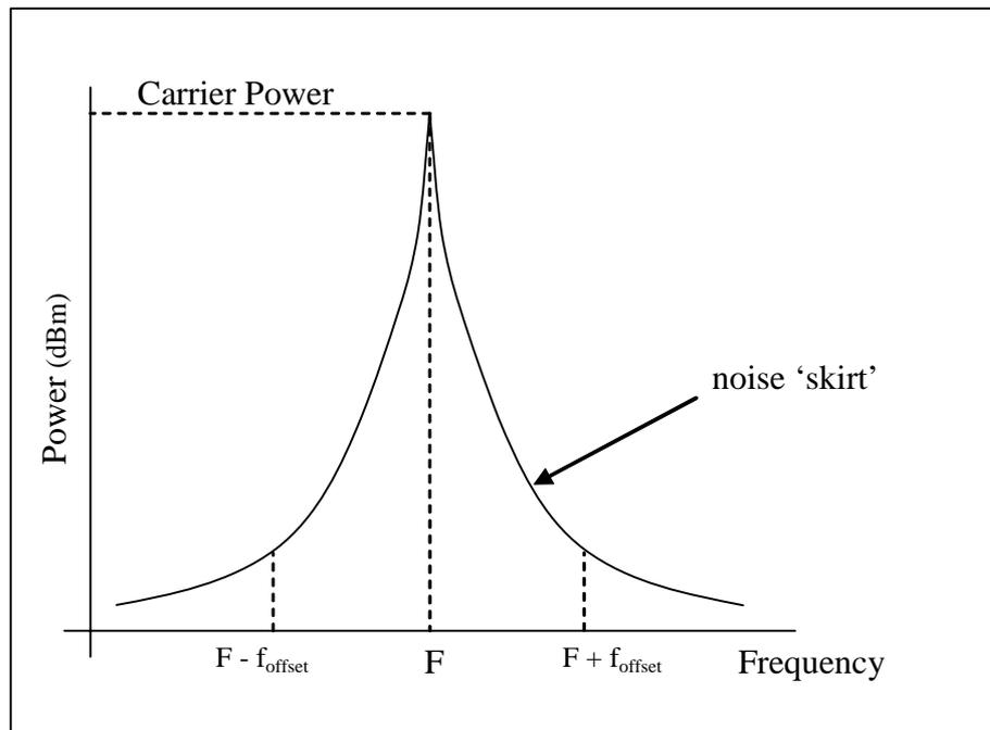
**Figure A-1.** Carrier Phase Noise
