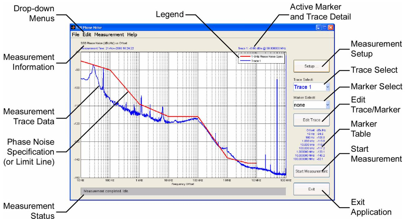
**Figure 2-1.** Main SSB Phase Noise Display
