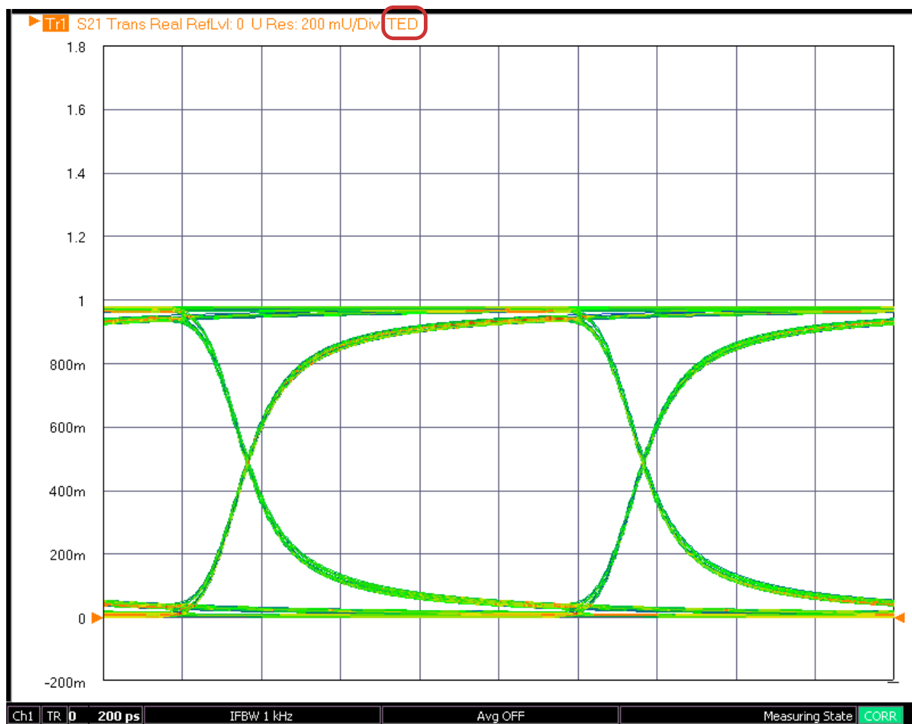
Figure 27-19. Time, Eye Diagram Display Example – Note that when in Time, Eye Diagram mode, the display trace annotation displays “TED”.
