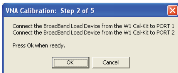
Figure 4-25. VNA Calibration: Step 2 of 5 Dialog
