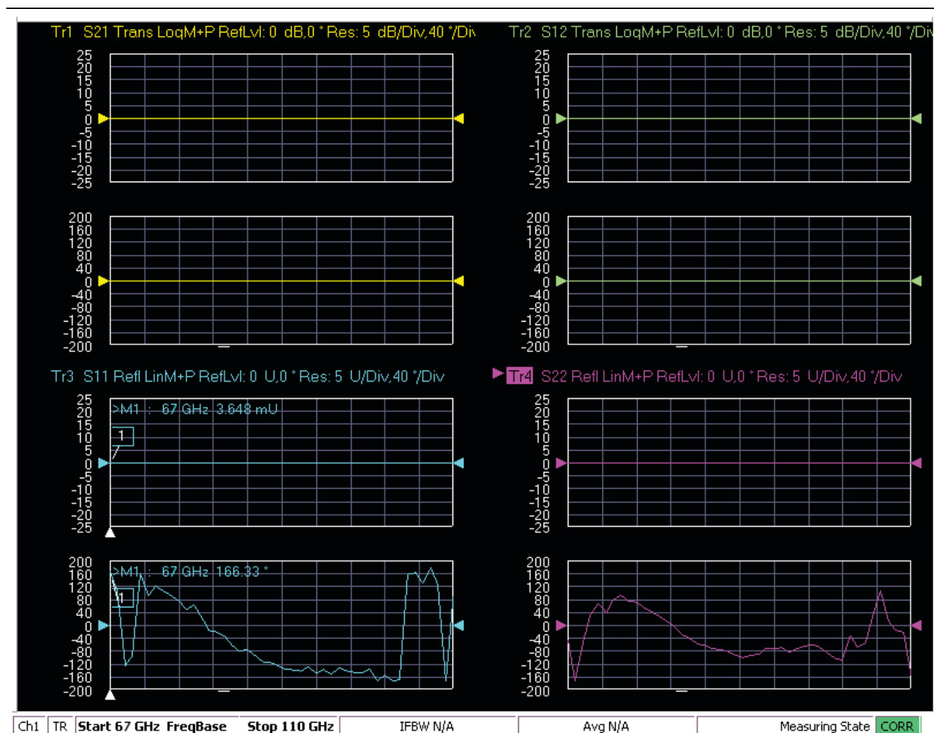
Figure 2-37. MS4640A/B Series VNA Auto Scale Example – Trace Display
