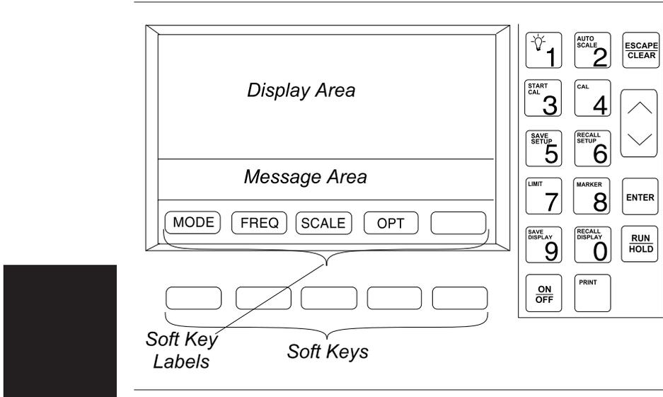
Figure 2-2. Site Master Front Panel Display Layout
