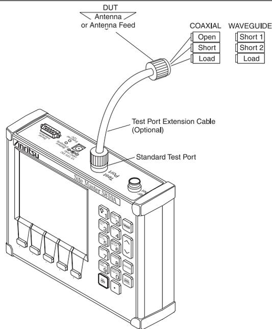
Figure 2-8. One-Port Measurement/Calibration Test Setup
