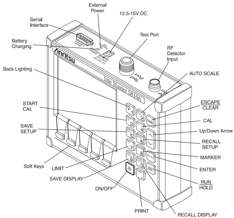
Figure 2-1. **Site Master** Controls and Connectors
