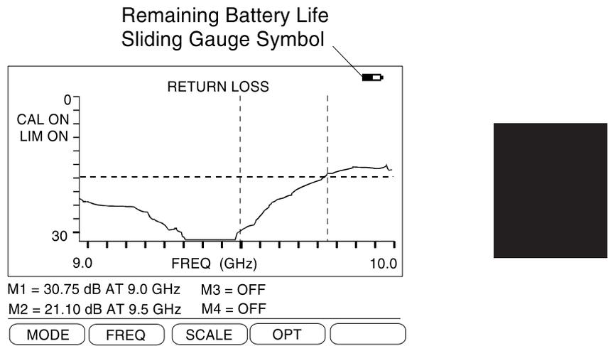
Figure 2-9. Battery Monitor
