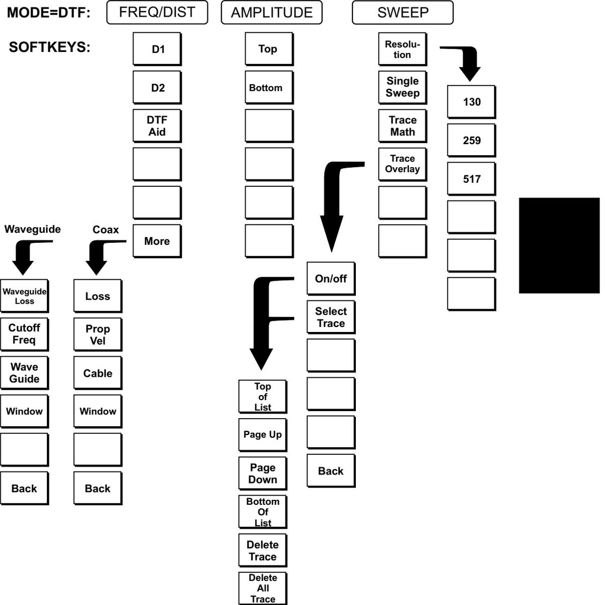
Figure 2-5. Distance to Fault Mode Soft Key Labels
