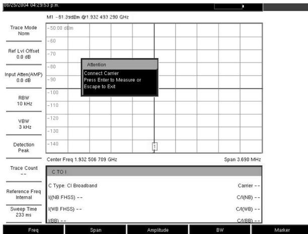
**Figure 3-19. C/I Measurement, Ready to Measure the Carrier**
