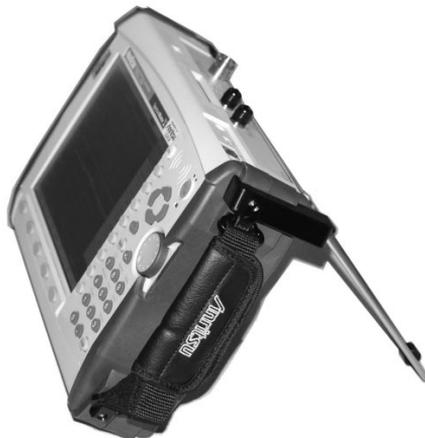
Figure 1-5. Tilt Bail Installed
