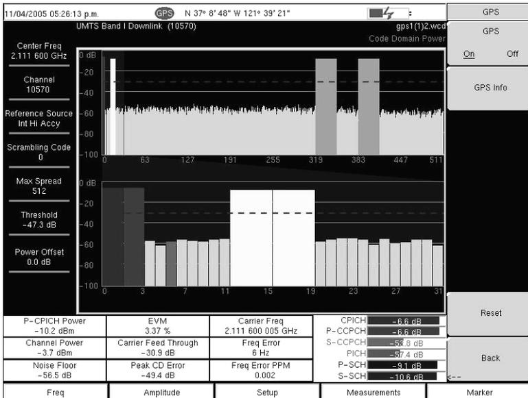
Figure 4-17. HSDPA Code Domain Power Measurement Screen Example
