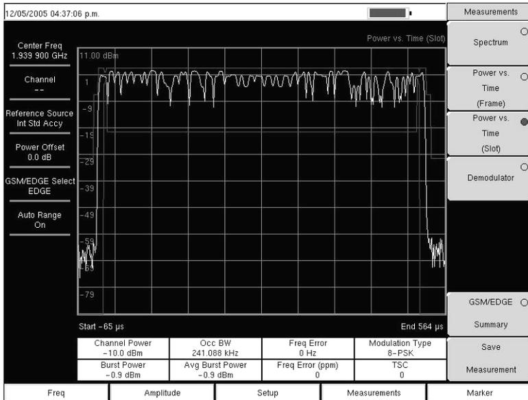
Figure 5-10. EDGE Power versus Time (Slot) Measurement Example
