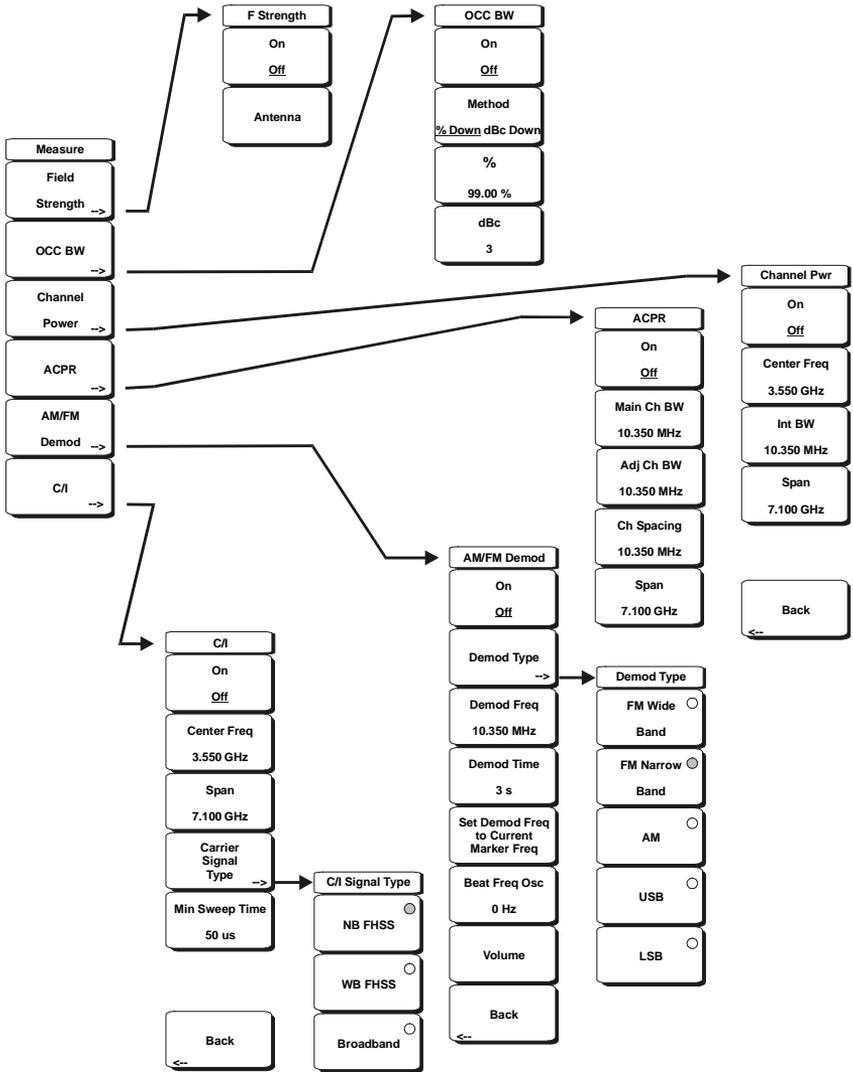
**Figure 3-8. Spectrum Analyzer Mode Measure Menu**
