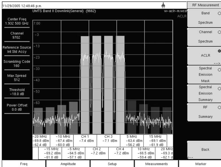
Figure 4-11. ACLR Multi-channel Measurement Example
