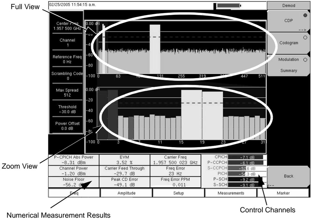
Figure 2-4. WCDMA Signal Analyzer CDP Display Overview
