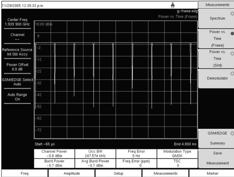
Figure 5-7. GSM Power versus Time (Frame) Measurement Example
