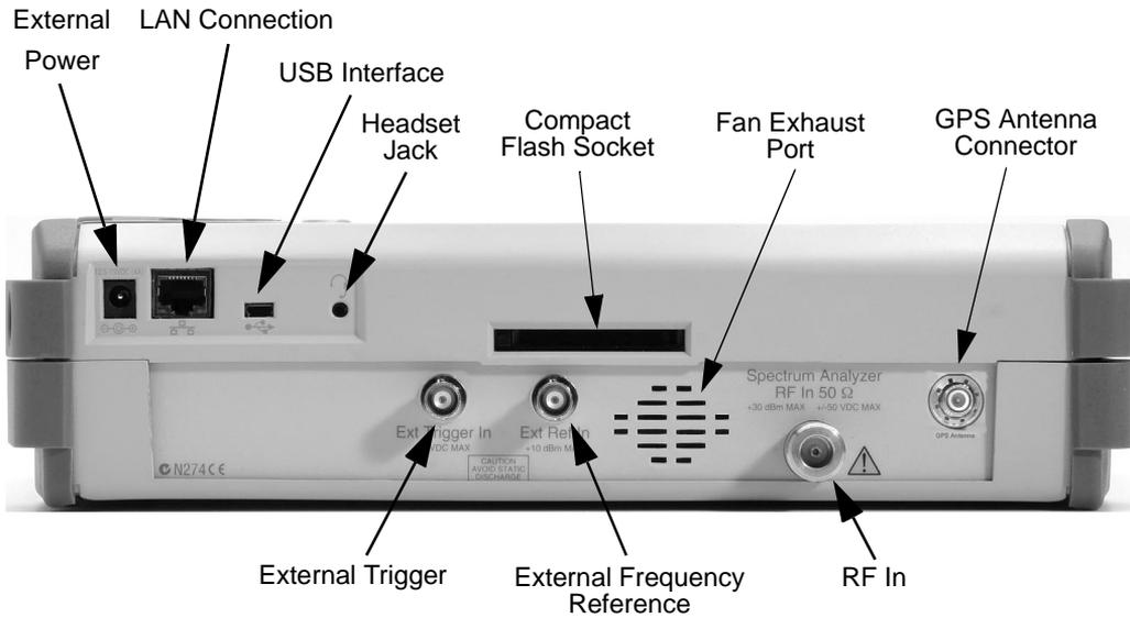
Figure 2-7. Test Panel Connectors
