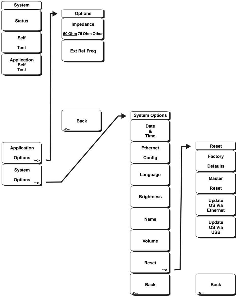
Figure 3-12. Spectrum Analyzer Mode System Menu
