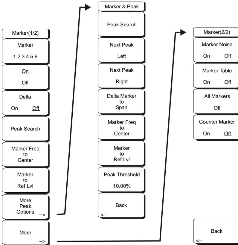
**Figure 6-9. Interference Analyzer Mode Marker Menu**
