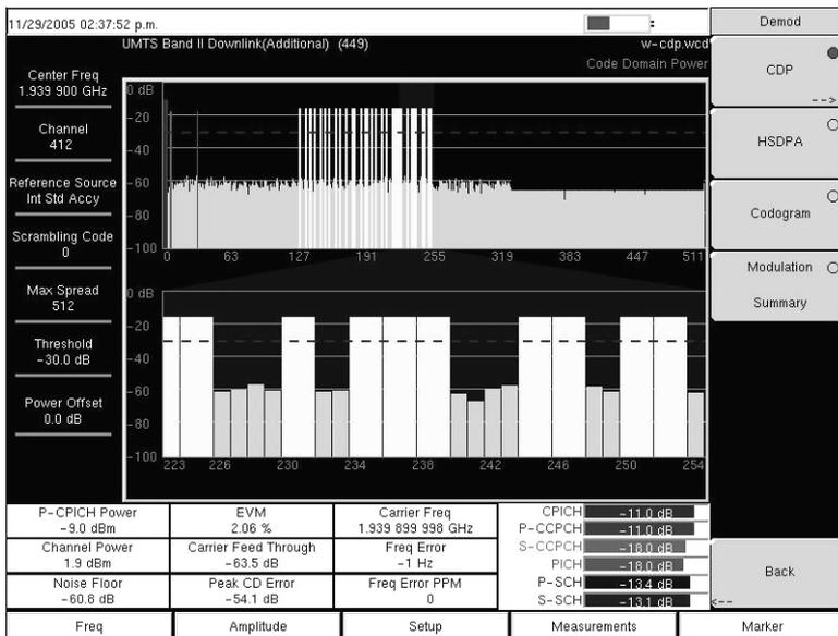
**Figure 4-15. WCDMA Code Domain Power Measurement Screen Example**
