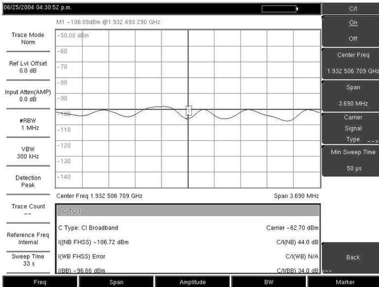
Figure 3-21. C/I Measurement, Results
