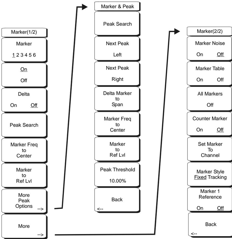
**Figure 3-6. Spectrum Analyzer Mode Marker Menu**
