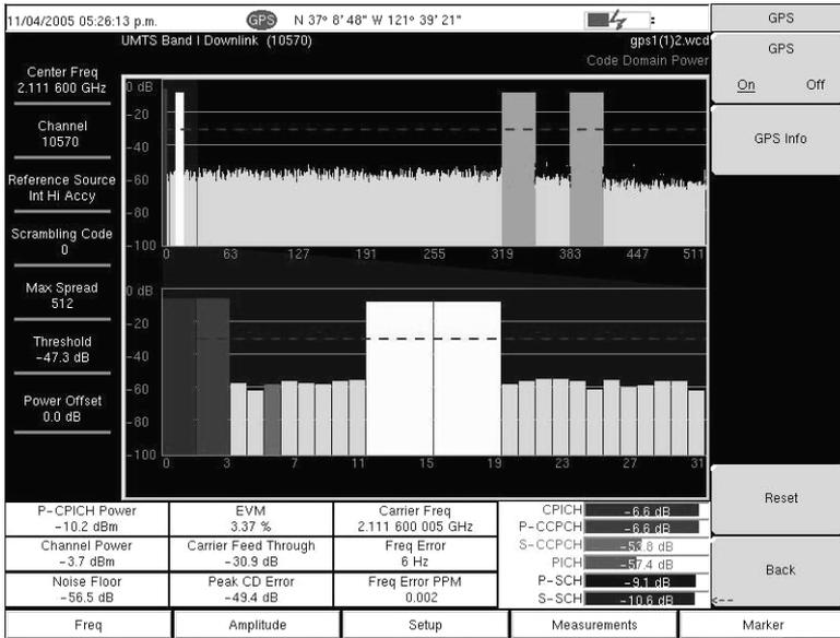
Figure 4-16. Code Domain Power Measurement Screen with GPS High Accuracy Example
