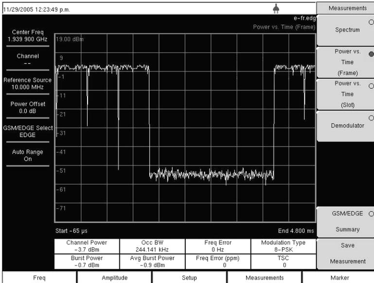
Figure 5-8. EDGE Power versus Time (Frame) Measurement Example
