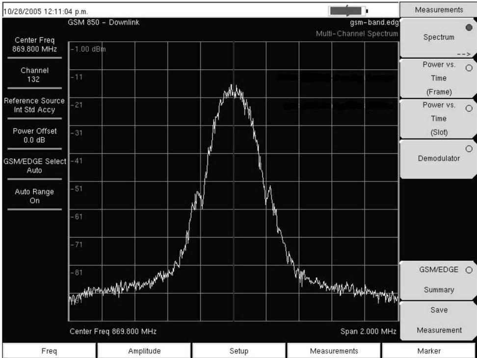
Figure 2-6. GSM Signal Analyzer RF Spectrum Display
