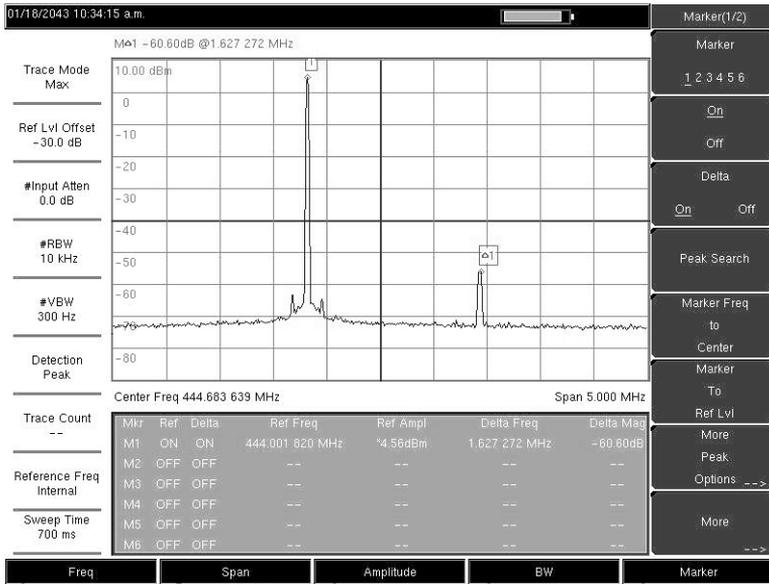
Figure 3-18. In-band Spurious Measurement
