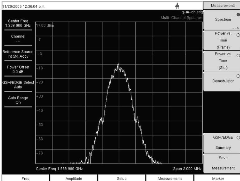
Figure 5-6. GSM Multi-channel Measurement Example
