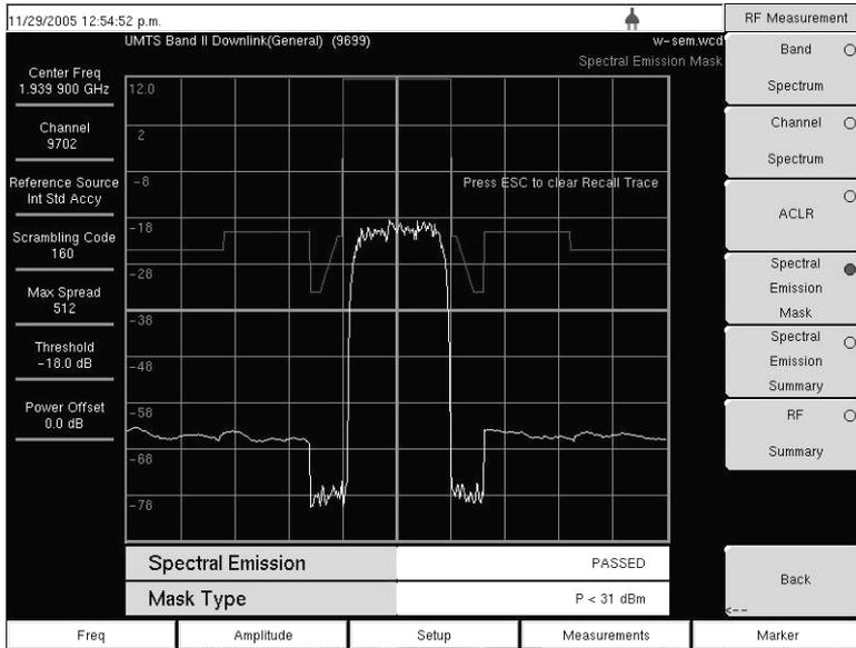
Figure 4-12. Spectral Emission Mask Measurement Example
