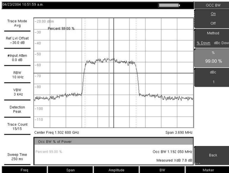
Figure 3-16. Occupied Bandwidth Results Using the % of Power Method
