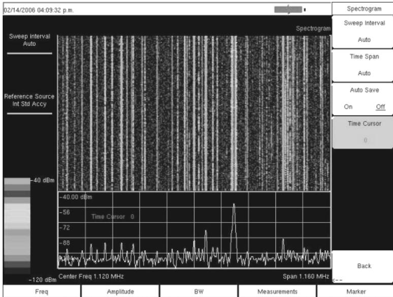
**Figure 6-10. Interference Analyzer Mode Sample Spectrogram Display**
