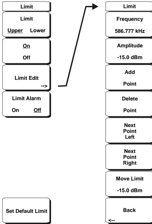
**Figure 3-5. Spectrum Analyzer Mode Limit Menu**
