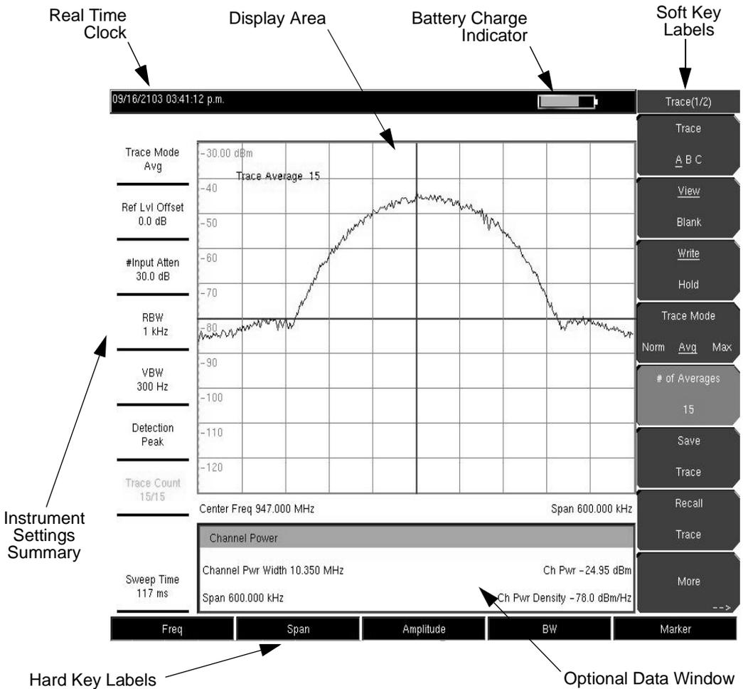
Figure 2-3. Spectrum Analyzer Display Overview
