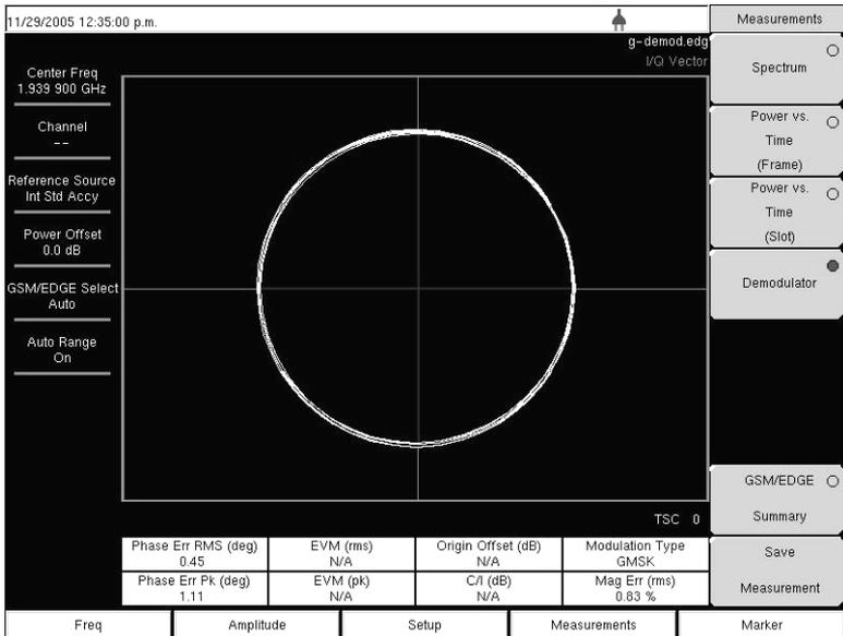
**Figure 5-11. GSM Demodulator Measurement Example**
