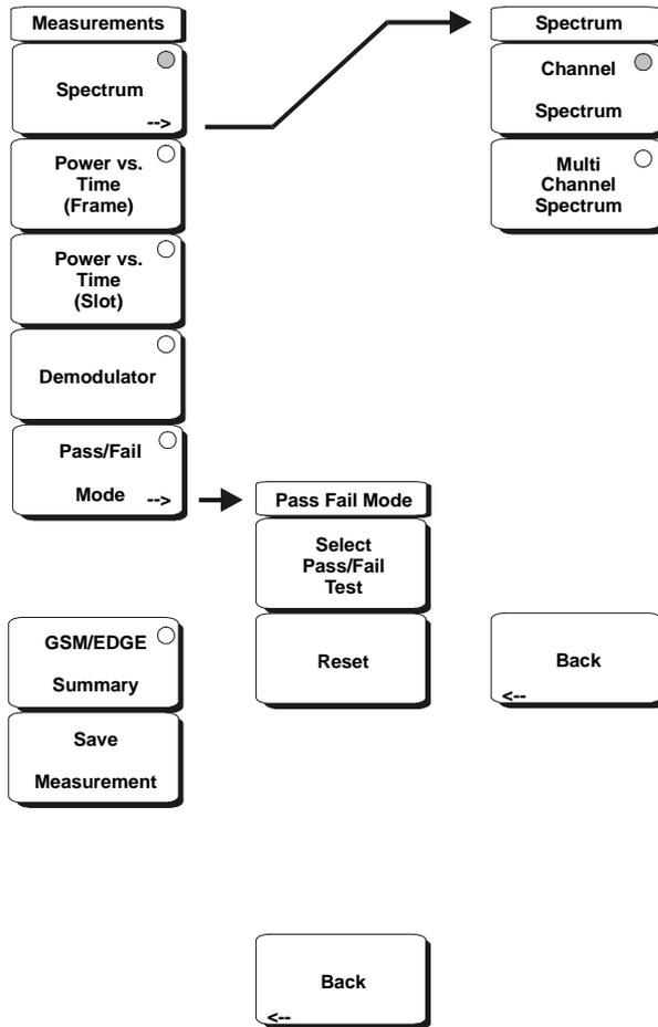
**Figure 5-4. GSM/GPRS/EDGE Mode Measurements Menu**
