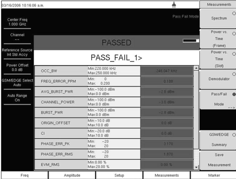
Figure 5-15. Pass/Fail Mode Example Screen
