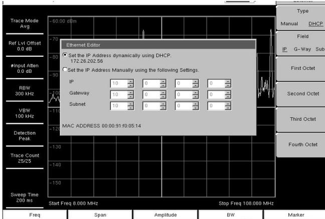
**Figure 2-8. IP Address Assigned Using DHCP**
