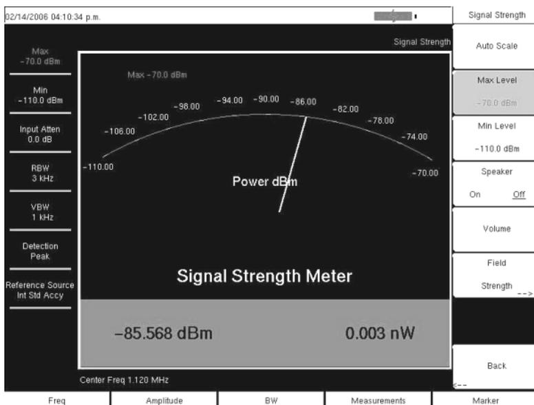
Figure 6-11. Interference Analyzer Mode Signal Strength Display
