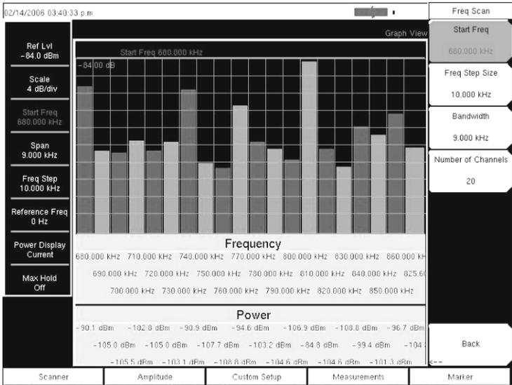
**Figure 7-5. Channel Scanner Mode Sample Graph Display**
