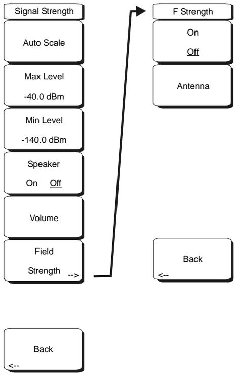
**Figure 6-7. Interference Analyzer Mode Signal Strength Menu**
