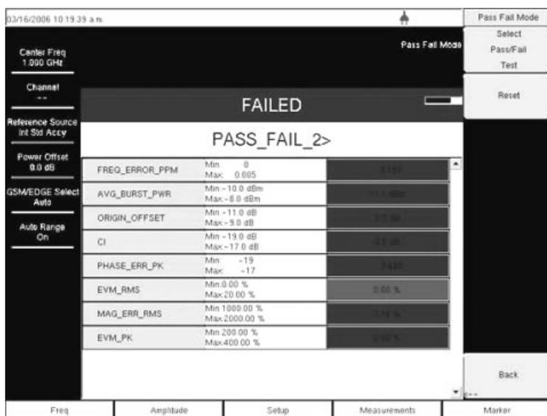
**Figure 5-16. Pass/Fail Mode Test Results Example**
