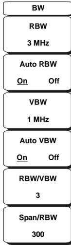
**Figure 3-2. Spectrum Analyzer Mode Bandwidth Menu**
