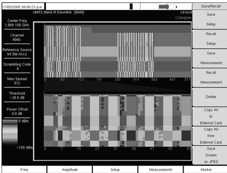
**Figure 4-19. Codogram Measurement Screen Example**
