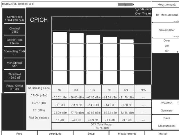
**Figure 4-20. OTA Measurement Screen Example**
