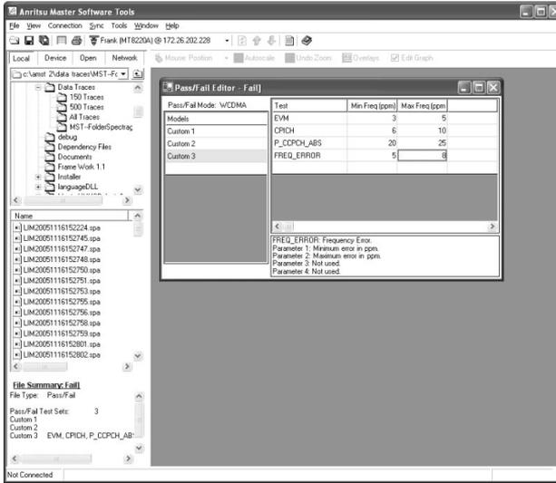
Figure 9-9. Master Software Tools Pass/Fail Editor
