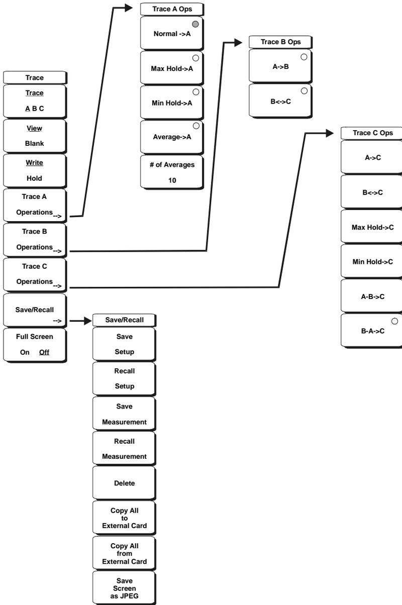
**Figure 3-13. Spectrum Analyzer Mode Trace Menu**
