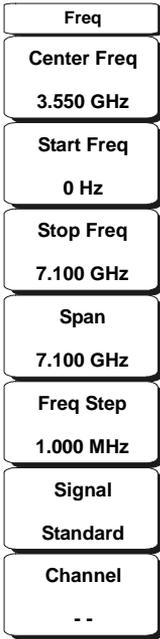
**Figure 3-4. Spectrum Analyzer Mode Frequency Menu**
