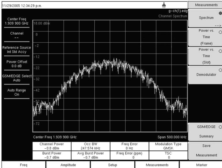
Figure 5-5. GSM Single Channel Measurement Example
