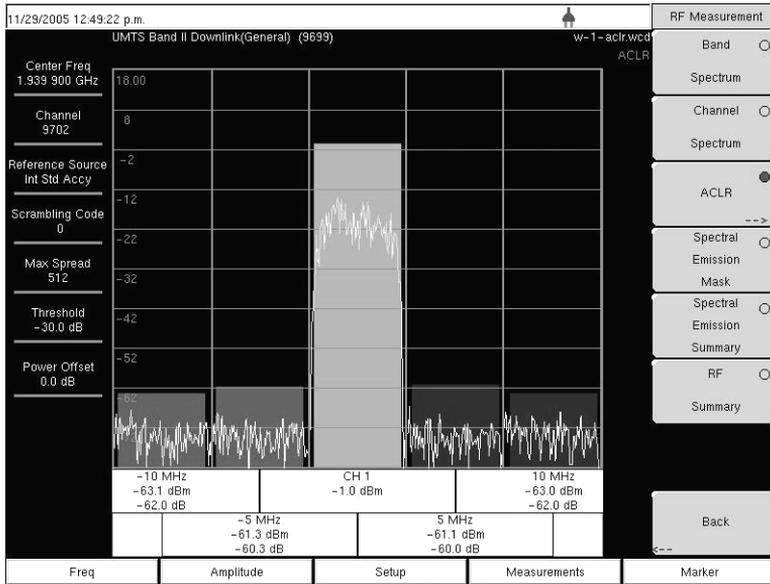
**Figure 4-10. ACLR Measurement Example**
