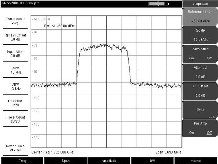
Figure 3-14. Preamplifier Off
