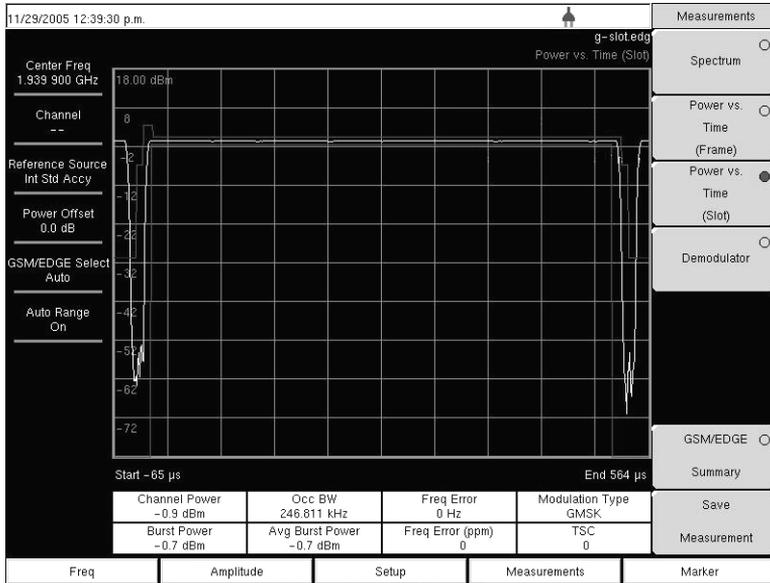
Figure 5-9. GSM Power versus Time (Slot) Measurement Example
