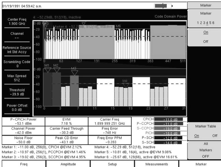
**Figure 4-18. Code Domain Power Measurement Screen Example with Markers Activated**
