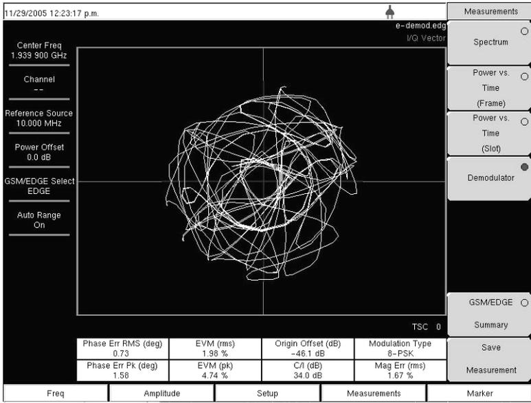
**Figure 5-12. EDGE Demodulator Measurement Example**
