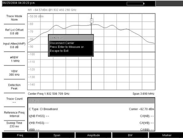
Figure 3-20. C/I Measurement, Carrier Measured
