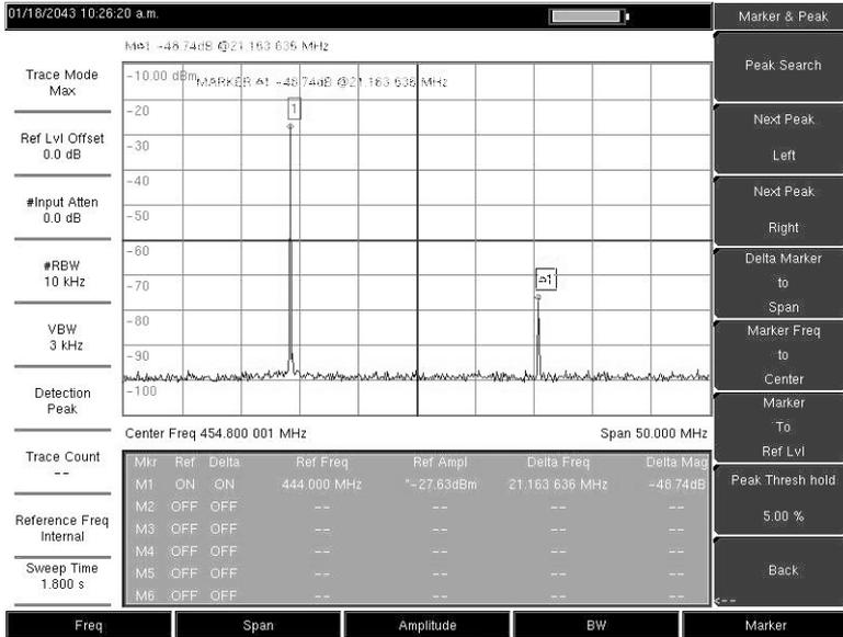
Figure 3-17. Simulated Out-of-Band Spurious Emission Measurement
