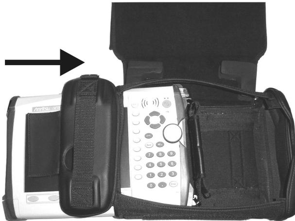
**Figure 1-3. Inserting the Instrument into the Soft Case**
