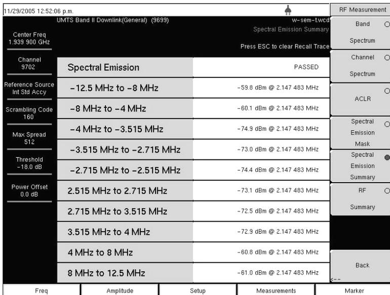
Figure 4-13. Spectral Emission Mask Measurement Summary Example
