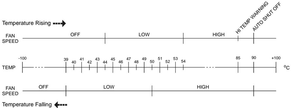
**Figure B-1. Fan Speed vs. Temperature**
