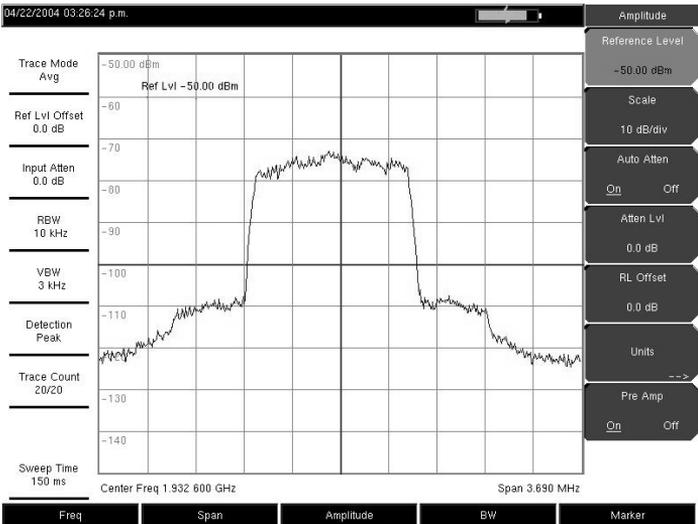
Figure 3-15. Preamplifier On
