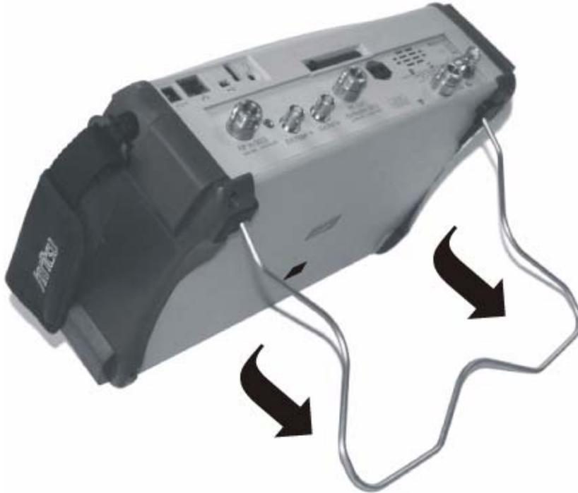
**Figure 1-5.** Tilt Bail Extended on VNA Master
