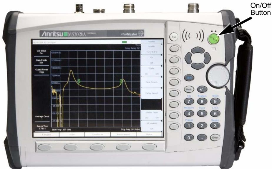
**Figure 2-1.** VNA Master On/Off Button (MS2026A shown)
