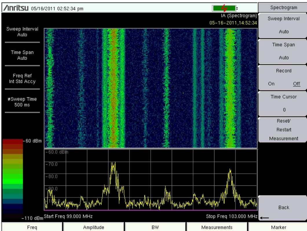
Figure 3-1. Spectrogram Example
