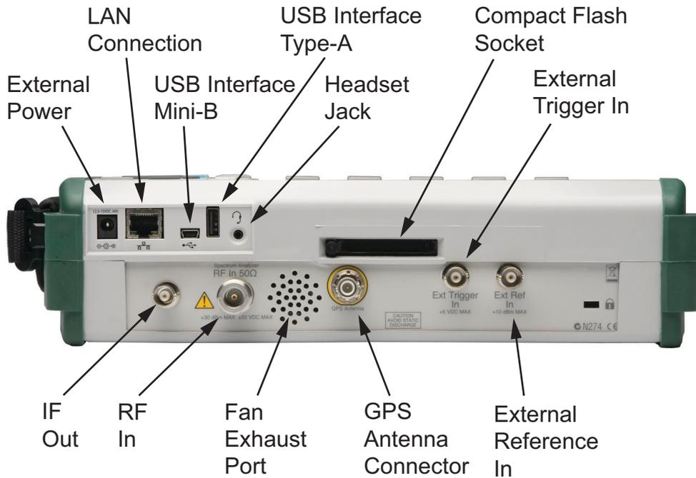
**Figure 2-11.** Test Panel Connectors for MS2723B and MS2724B
