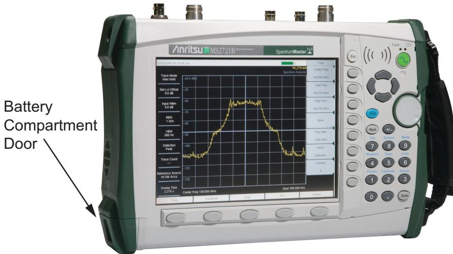
**Figure 1-1.** Battery Compartment Door
