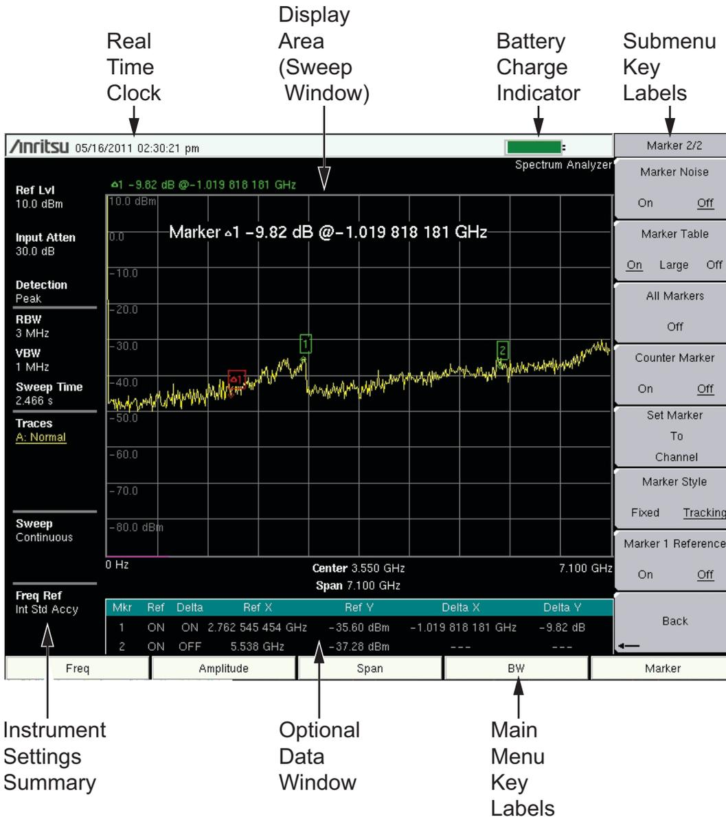
Figure 2-6. Spectrum Analyzer Display
