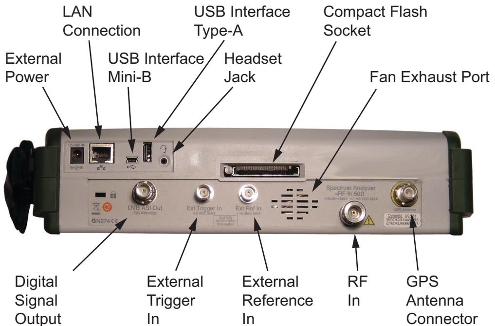
**Figure 2-12.** Test Panel Connectors for MS8911B
