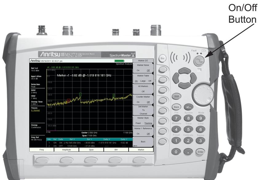
Figure 2-1. Spectrum Master On/Off Button
